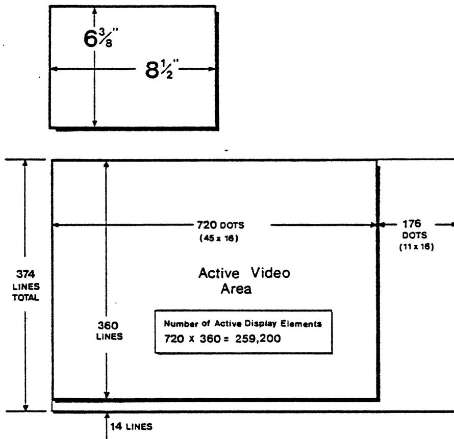
The video circuit fetches a 16 bit word from main memory once every four CPU clock cycles, and shifts it out to the CRT to provide a bit mapped display. The data in the bit map is displayed as an image of the bits in memory. A one corresponds to a dark (off) dot, and a zero corresponds to a bright (on) dot. Wait states are inserted into each memory fetch so that it takes a multiple of four cycles.
