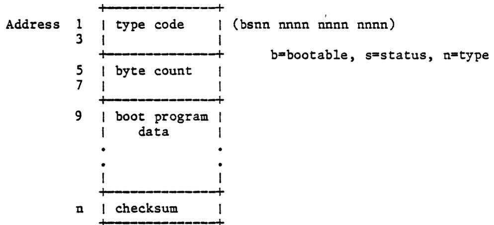
The type code is a 16 bit female byte sex number (most significant byte first) stored in the first two bytes of the ROM. If the first bit is a 1 (see above), the device claims to be bootable. If the device's status should be checked at boot time, its status bit (the second bit) is a 1. The other 14 bits are the identification number which identifies the card.
