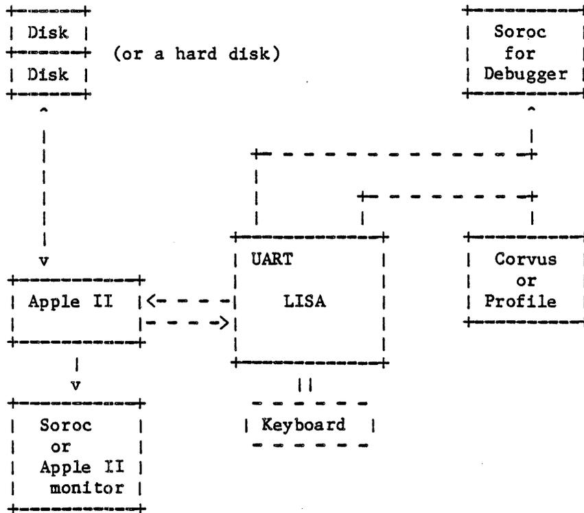
The hard disk can be connected directly to the Lisa, or it can be accessed through the Apple II. It can also be omitted.
