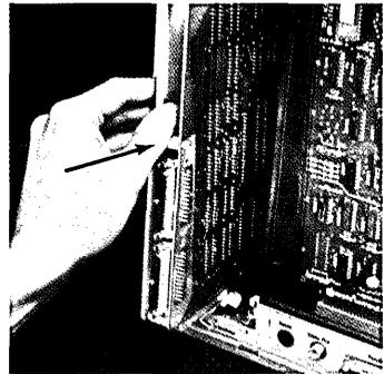
10. Turn the metal lever counterclockwise 90 degrees, back to the 12 o'clock position.
