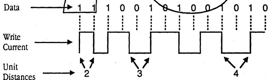
Fig. 8.1 MFM Encoding
