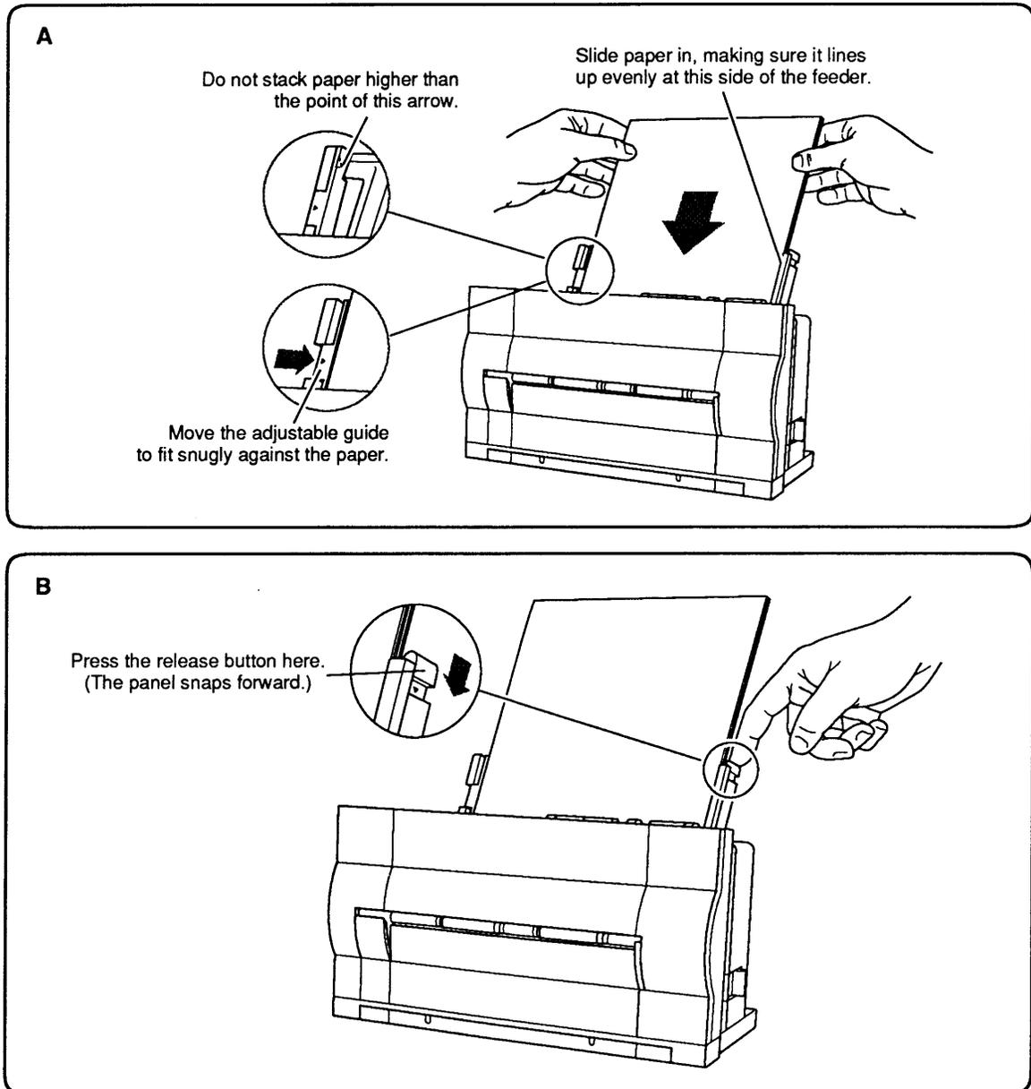
**Figure 1-9** Loading Paper into the Cut Sheet Feeder
