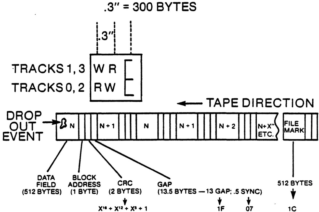
1. Read head detects error on block N —write head at byte 287 of N + 1.
