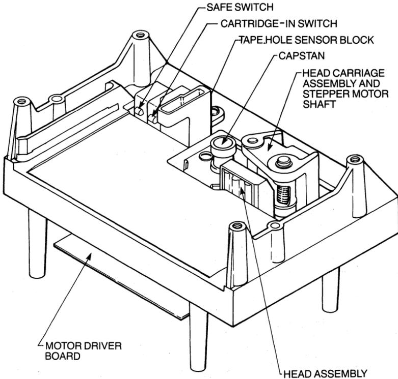
**Figure 5-12** Archive streaming-cartridge drive subassemblies.
