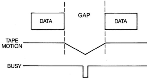
**Figure 4-5** Conventional start-stop operation, ½-inch tape.
