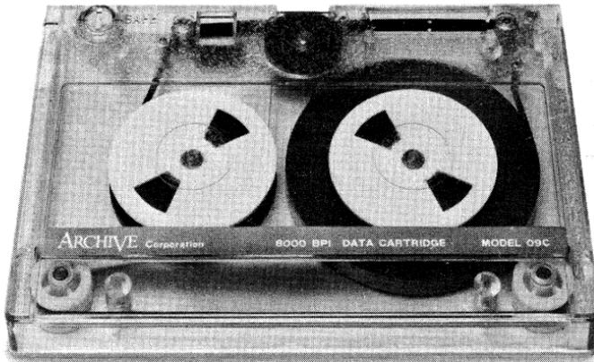
**Figure 5-3** Standard ¼-inch tape cartridge.
