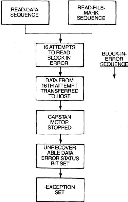
Figure 9-41 Block-In-Error Sequence.
