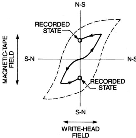
Figure 1-14 Unsaturated recording for higher densities.
