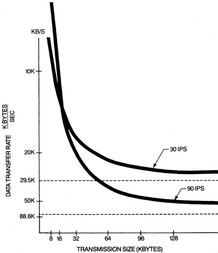
**Figure 7-1 Effect of transmission size on transfer rate.**
