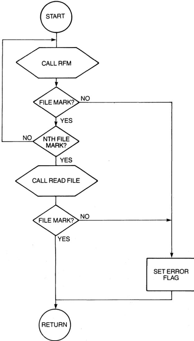
Figure 6-11 Flow diagram, read Nth file.
