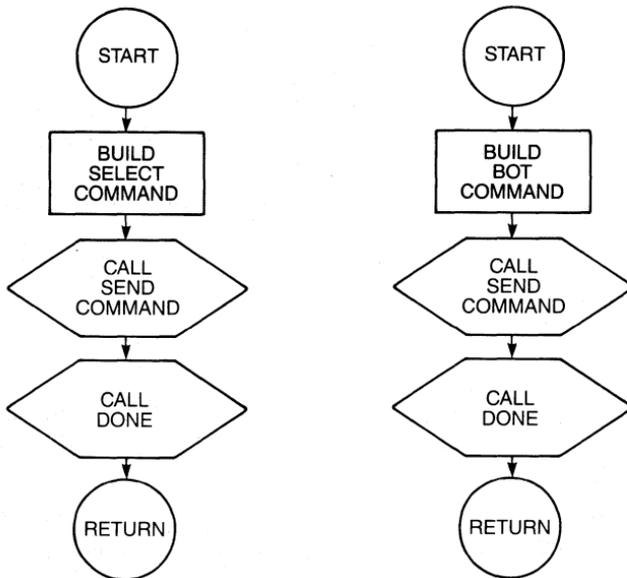
**Figure 6-5 Flow diagrams, SELECT and BEGINNING OF TAPE commands.**
