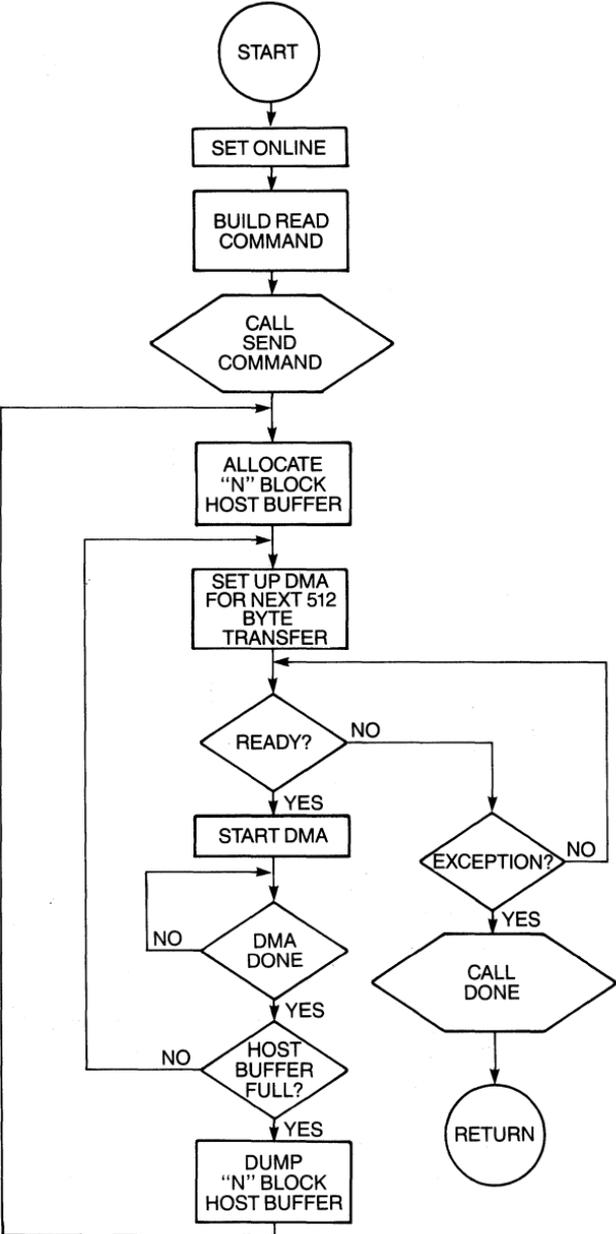
Figure 6-10 Flow diagram, read file.
