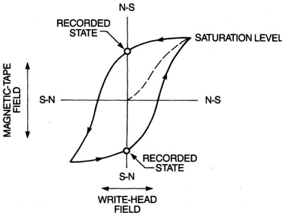
Figure 1-13 Conventional saturated recording.
