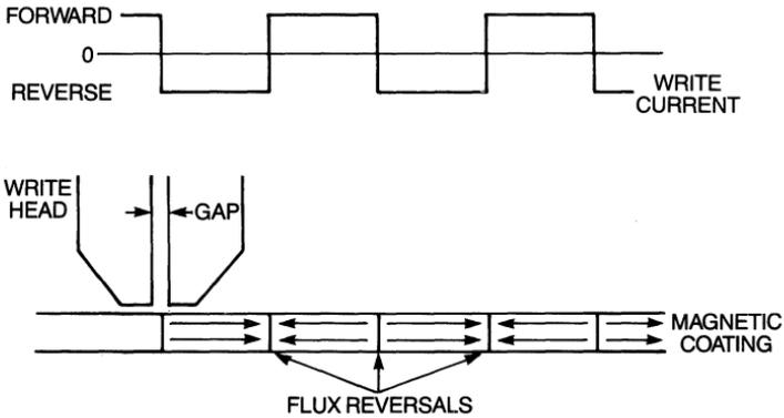
Figure 1-10 Flux reversals produced by write current.
