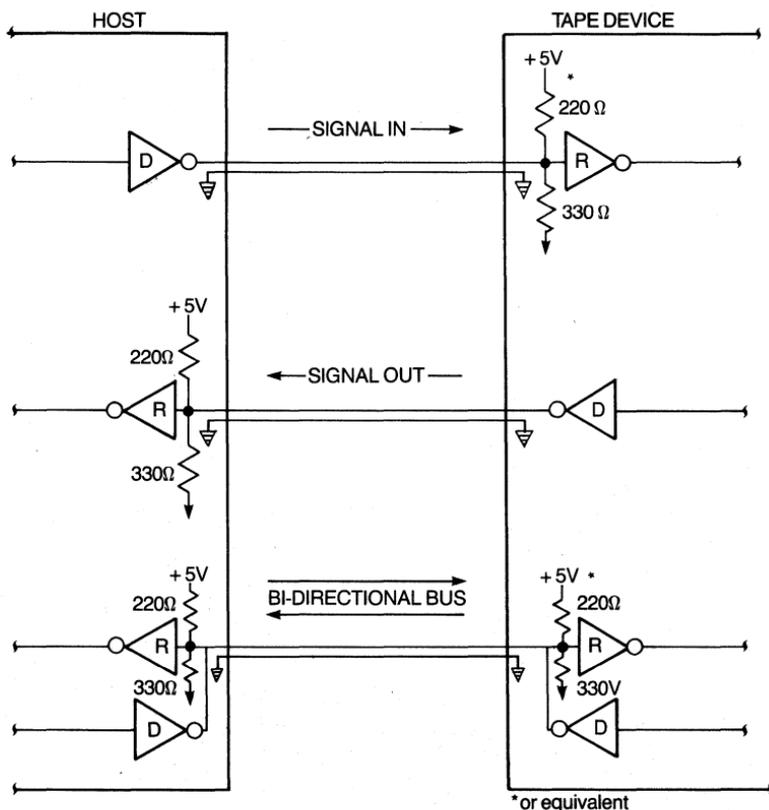
**Figure 9-8 Interface drivers and receivers.**
