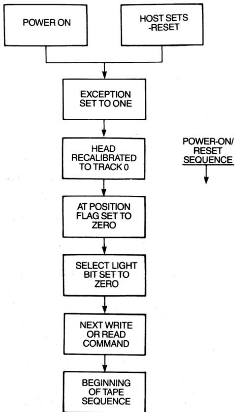
**Figure 9-12 Power On/Reset Sequence.**
