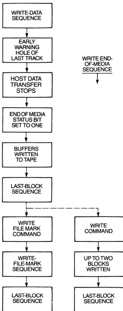
**Figure 9-24 Write End-of-Media Sequence.**
