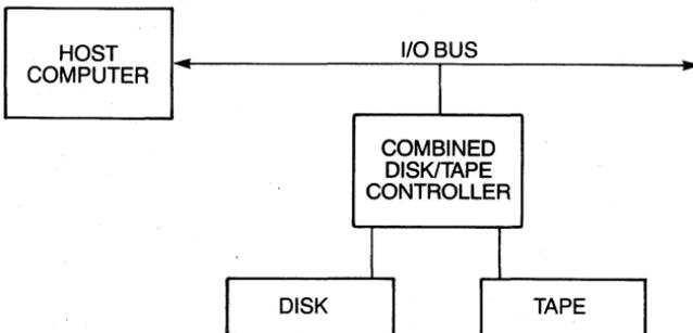
Figure 1-19 Combined disk-tape mass storage system.
