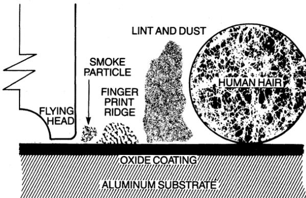
**Figure 2-2 Sources of disk contamination.**
