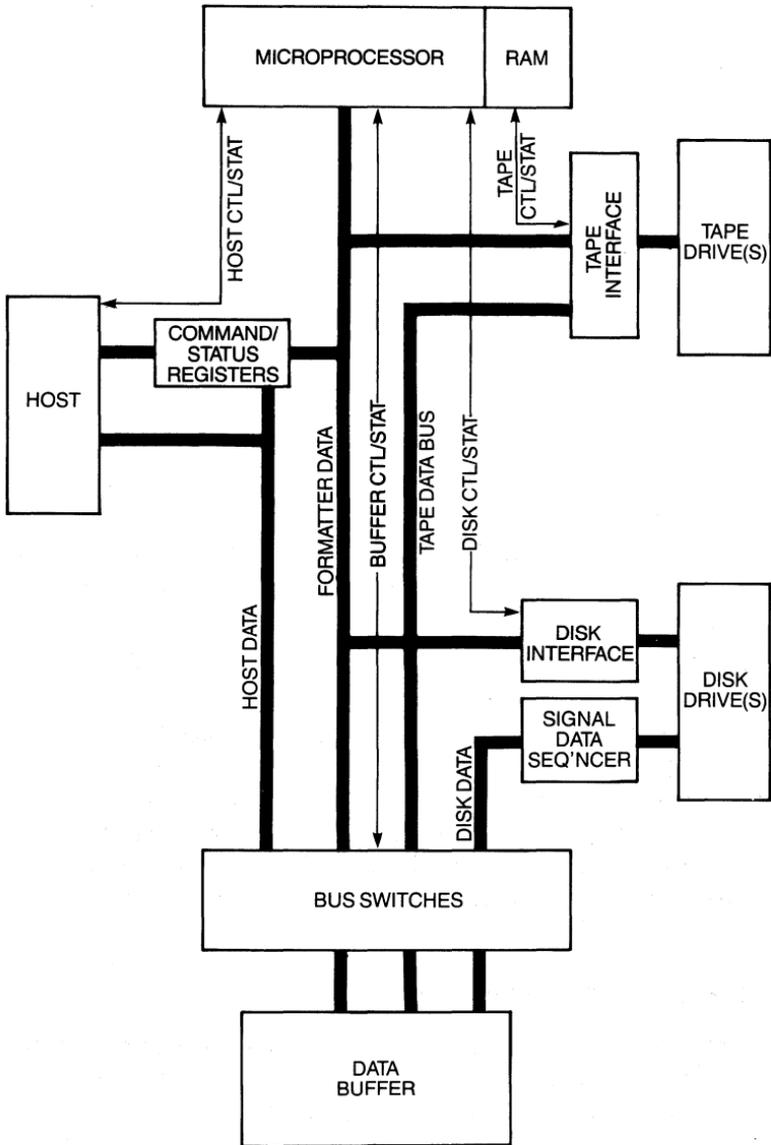
Figure 8-2 Block diagram, typical disk-tape controller.
