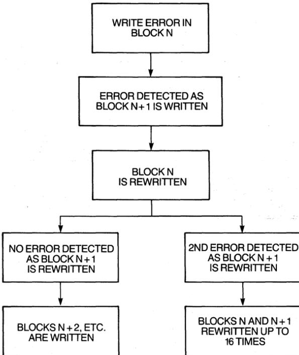
**Figure 9-30 Write-Error Sequence.**
