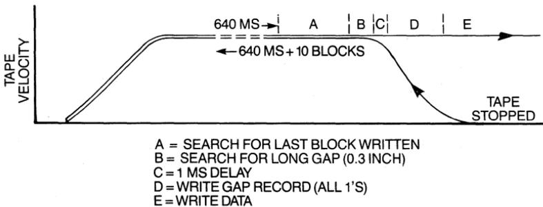
**Figure 9-28** Tape motion, Write-Reposition Sequence.
