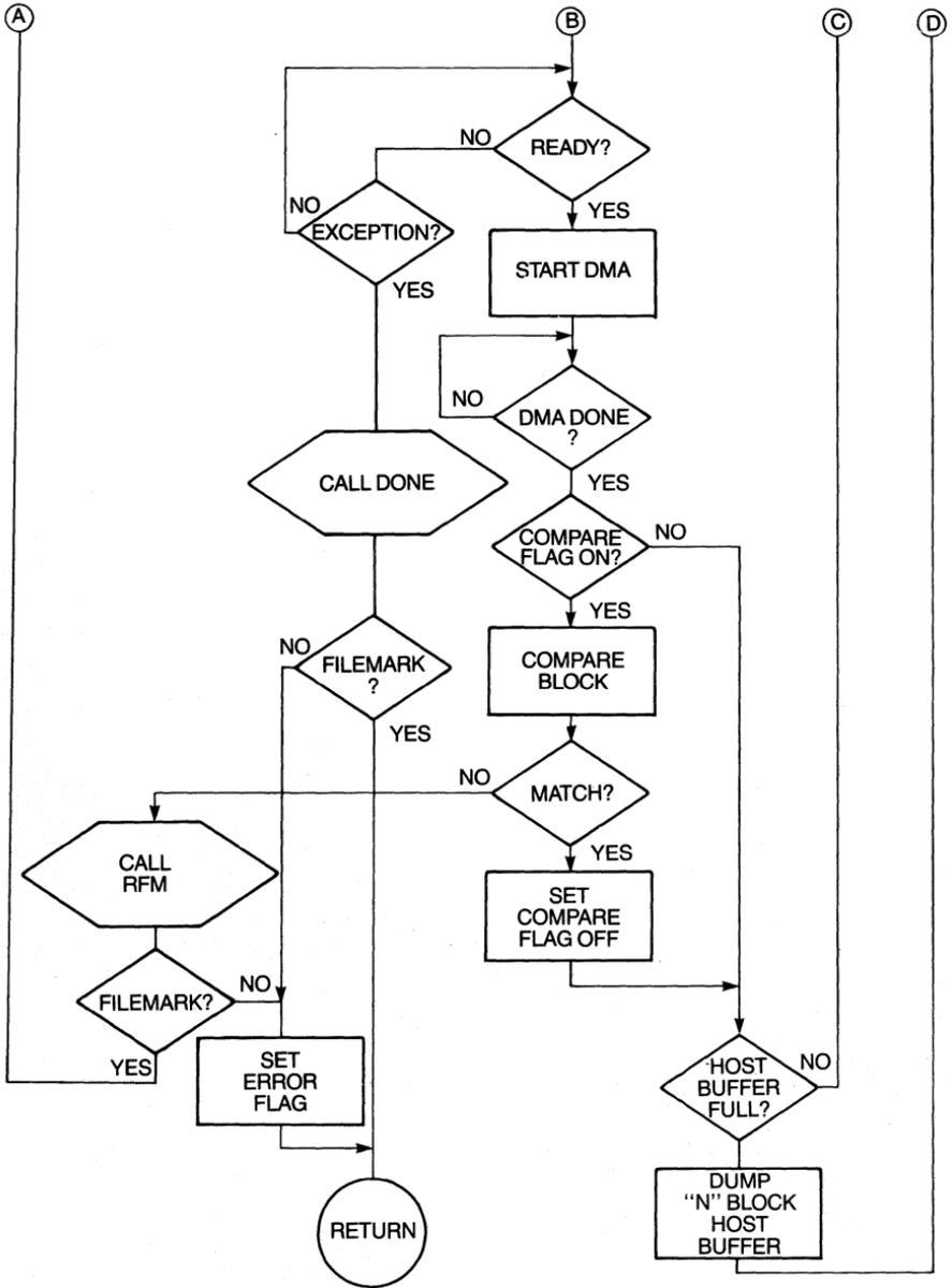
Figure 6-12(con.) Flow diagram, read file with first-block ID.
