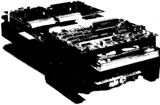
**Figure 5-21 Intelligent streaming-cartridge drive.**
