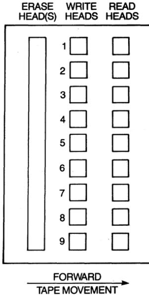
**Figure 4-1** Nine-track head for recording on 1/2-inch tape.
