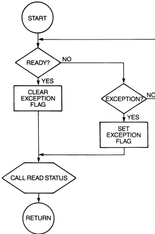
**Figure 6-3 Flow diagram, host done.**
