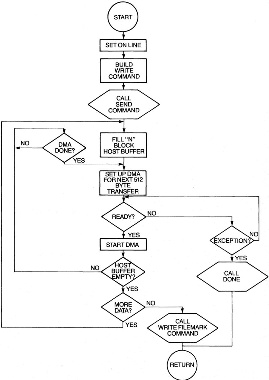
Figure 6-8 Flow diagram, write file .
