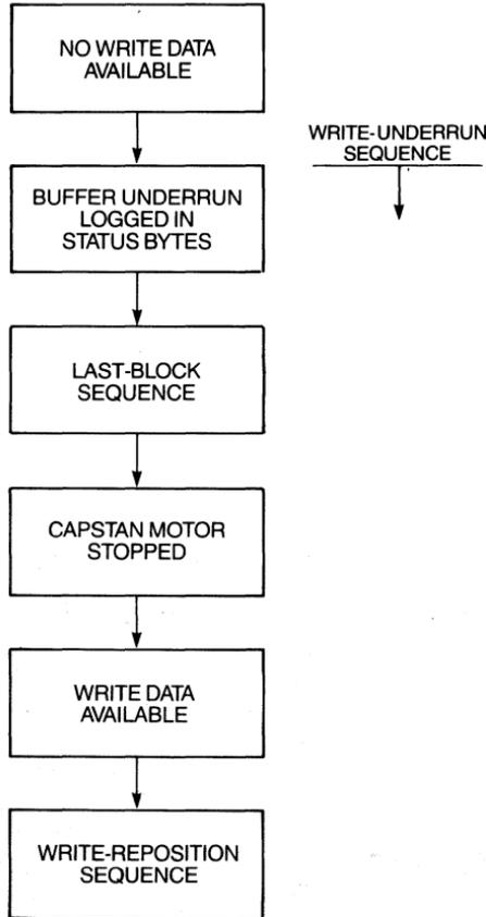
**Figure 9-22 Write-Underrun Sequence.**
