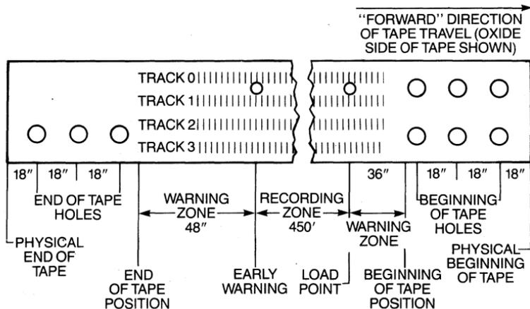
**Figure 5-7** Tape-position holes, 1/4-inch cartridge tape.
