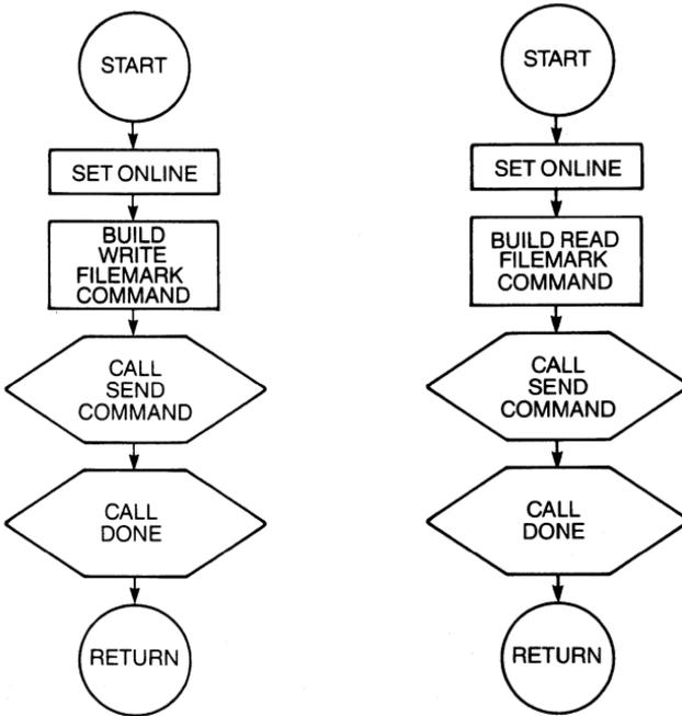
**Figure 6-7 Flow diagrams, WRITE FILE MARK and READ FILE MARK commands.**
