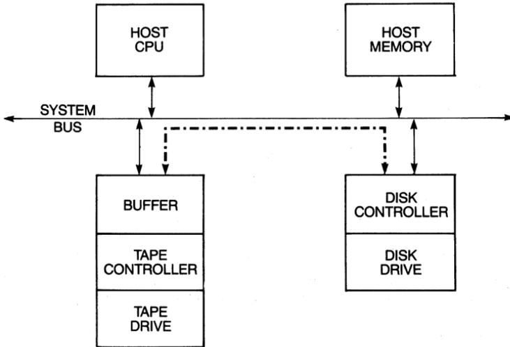
**Figure 7-3 Data buffer in tape controller.**
