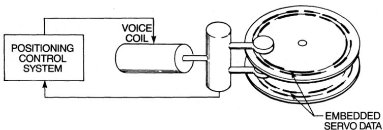
**Figure 2-6 Closed-loop with embedded servo code.**
