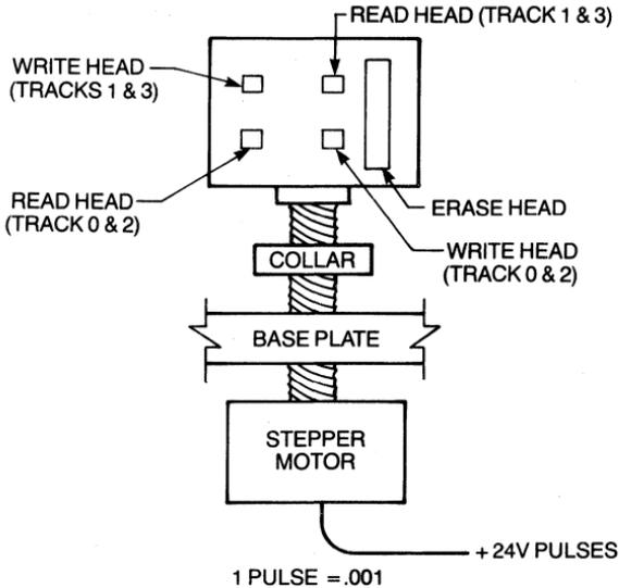
**Figure 5-14 Head-positioning mechanism.**
