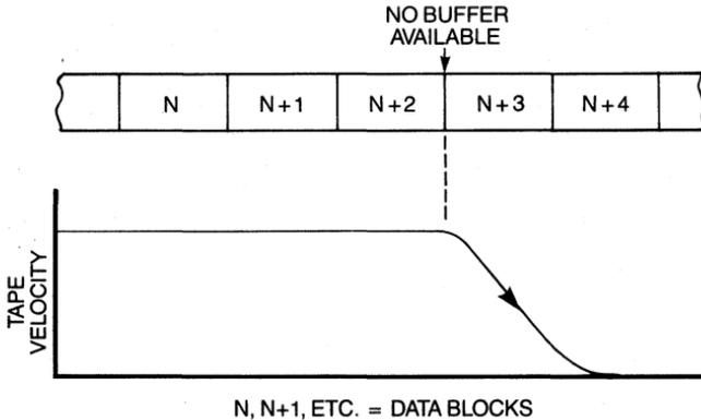
**Figure 9-33 Tape motion, Read-Underrun Sequence.**
