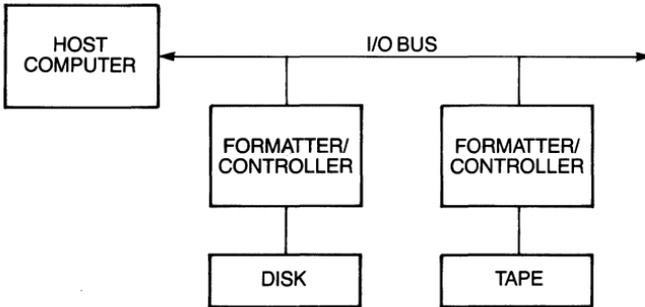
Figure 1-17 Non-intelligent devices with separate formatter/controllers.
