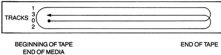
**Figure 5-10 Four-track serpentine recording.**
