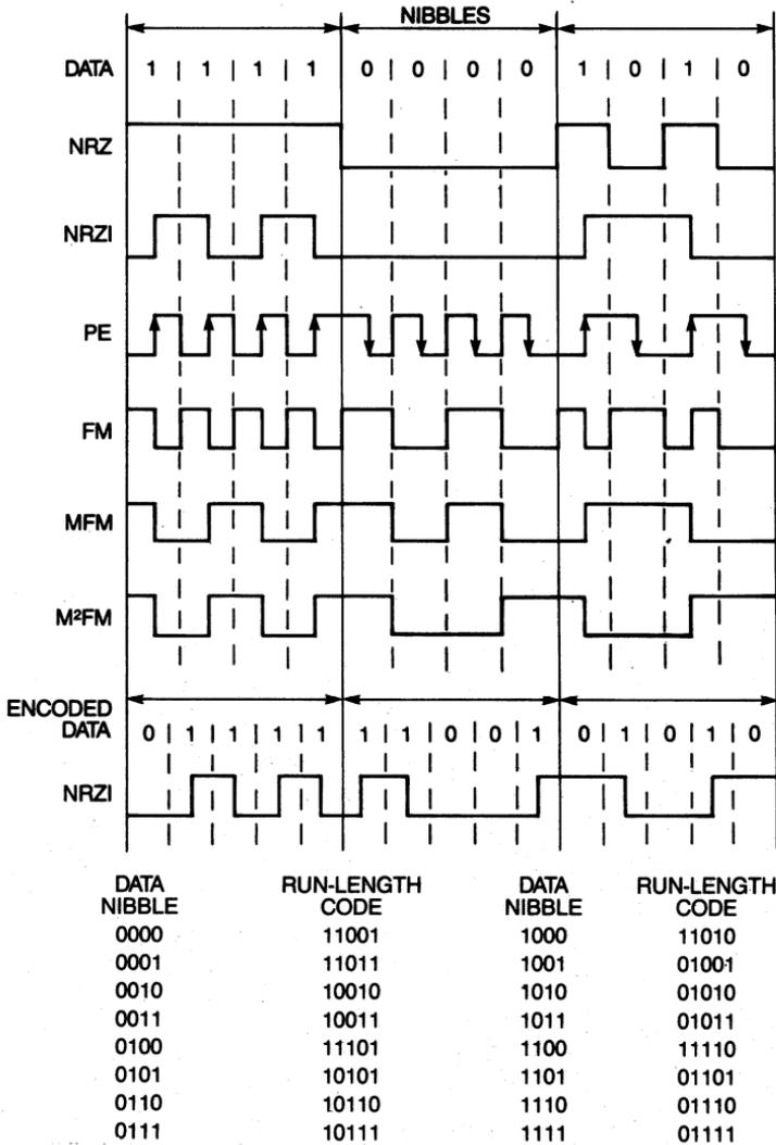
Figure 1-16 Flux-reversal codes for digital recording.
