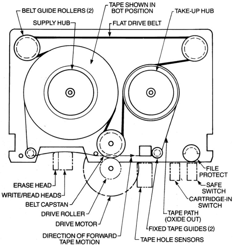
**Figure 5-4** Internal construction, 1/4-inch tape cartridge.
