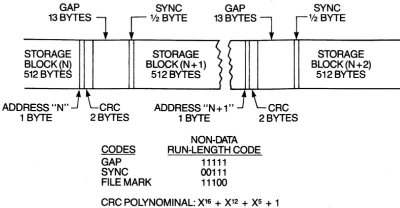
Figure 5-16 Streaming-cartridge tape format.
