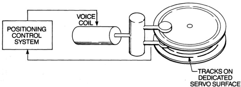
**Figure 2-5 Closed-loop with dedicated servo surface.**
