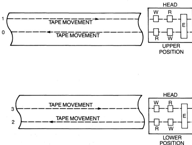
**Figure 5-13** Dual-head positions for 4-track recording.
