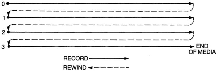
**Figure 5-8 Four-track, forward-only recording.**
