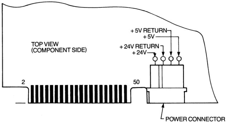
**Figure 9-9** Signal and power connectors.
