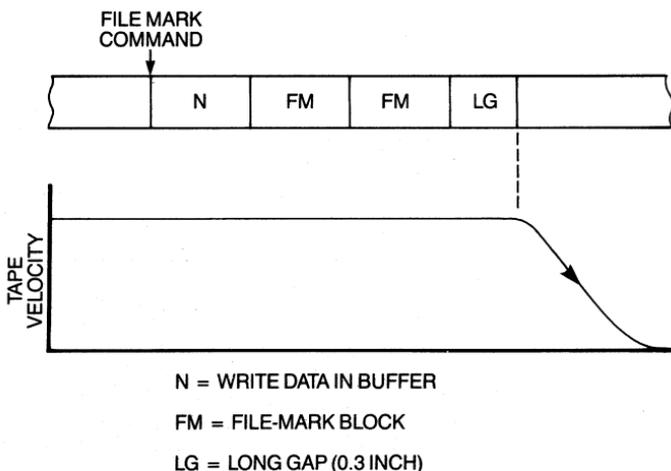
**Figure 9-26** Tape motion, Write-File-Mark Sequence.
