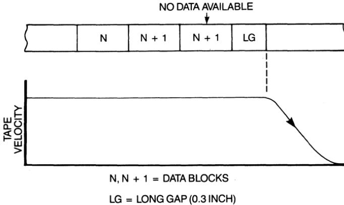
**Figure 9-23 Tape motion, Write-Underrun Sequence.**
