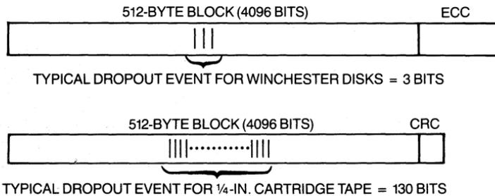
**Figure 5-17 ECC (error-correcting code) versus CRC (cyclic redundancy check).**
