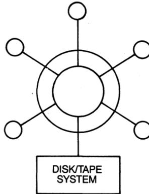
**Figure 1-22 Ring-type network with shared mass storage.**
