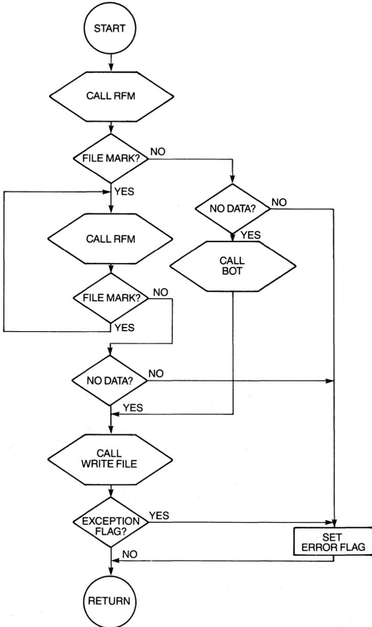
Figure 6-9 Flow diagram, append a file.
