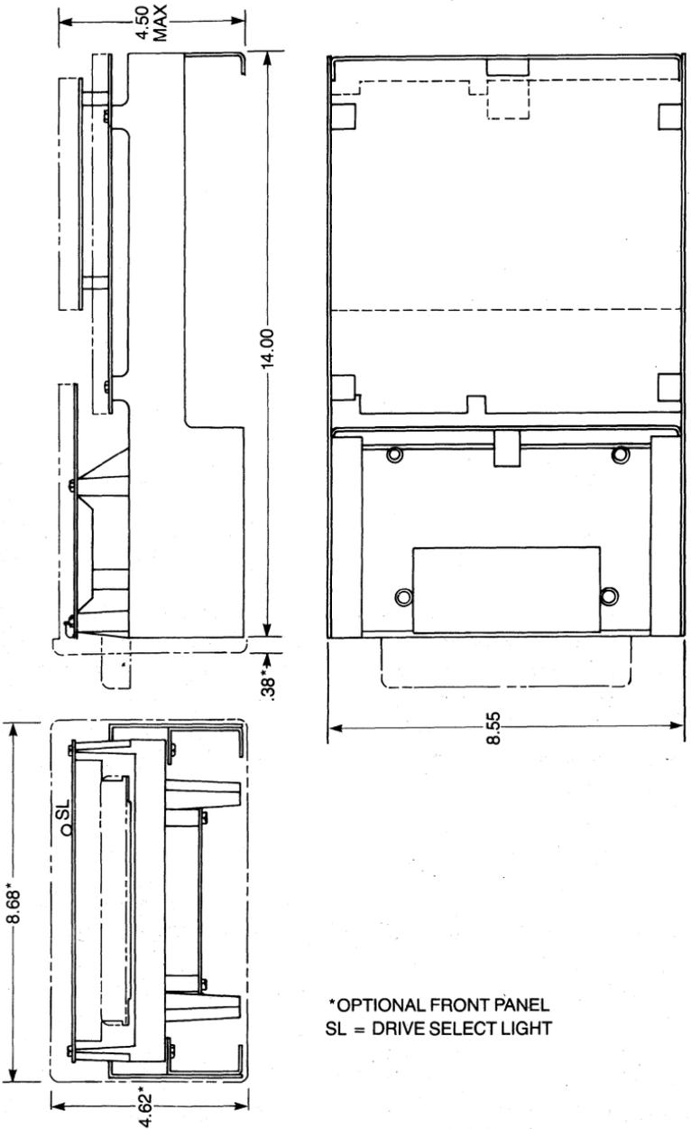
Figure 9-2 Dimensions, intelligent drive.
