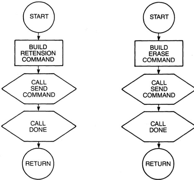
**Figure 6-6 Flow diagrams, RETENSION and ERASE commands.**
