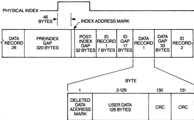
**Figure 3-3 Sector format, 8-inch flexible disk.**
