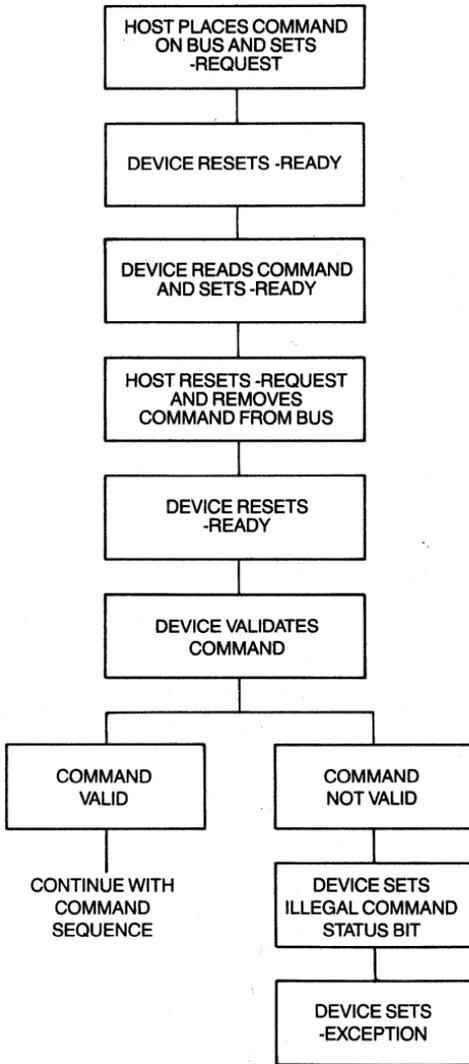
**Figure 9-13 Command-Reject Sequence**
