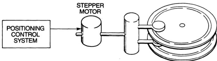
**Figure 2-4 Open-loop head positioning.**
