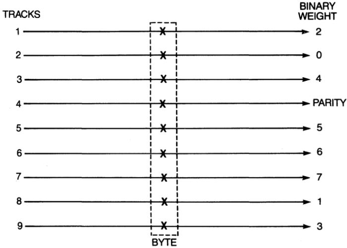
Figure 4-2 NRZI and PE recording, 1/2-inch tape.
