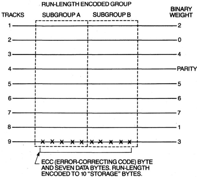
Figure 4-3 GCR (group-coded recording) 1/2-inch tape.
