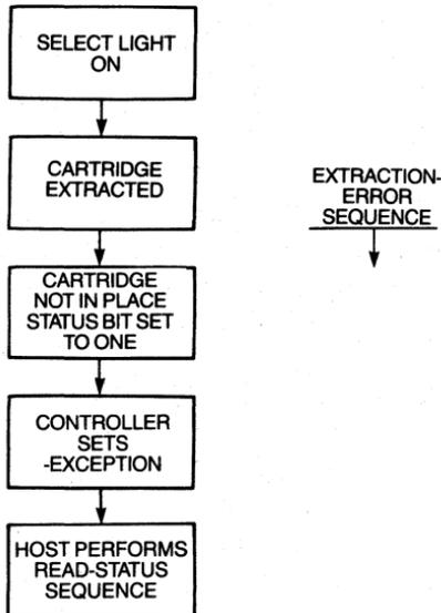
Figure 9-14 Cartridge-Extraction Sequence.
