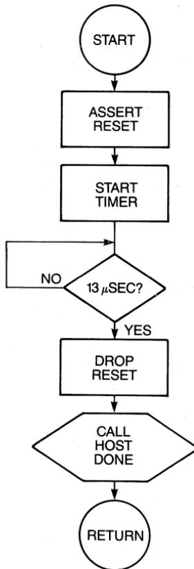
**Figure 6-4** Flow diagram, reset drive.
