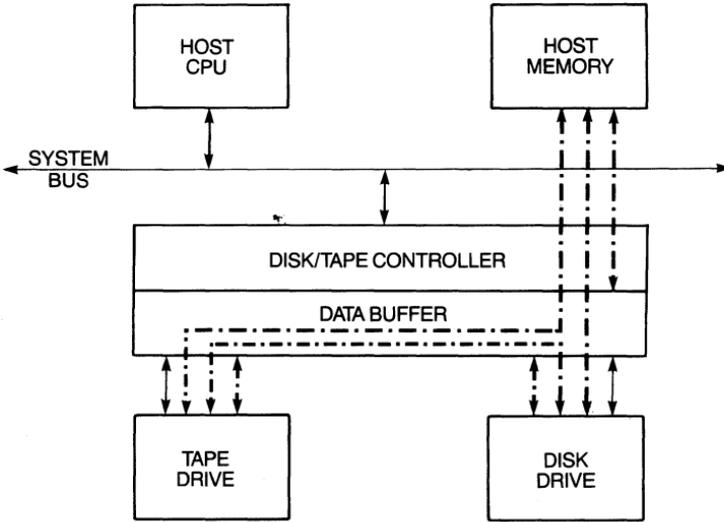
Figure 7-4 Data buffer in combined controller.
