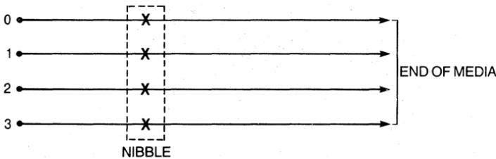
**Figure 5-9 Four-track parallel recording.**
