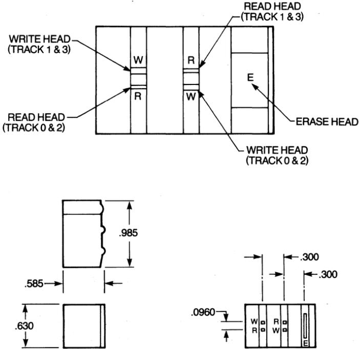
Figure 9-5 Read-after-write head dimensions.
