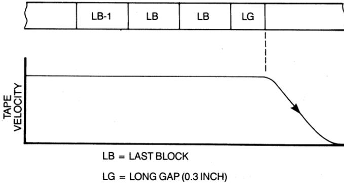
**Figure 9-21 Tape Motion, Last-Block Sequence.**
