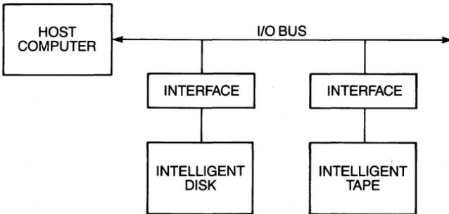
Figure 1-18 Intelligent devices with separate host interfaces.
