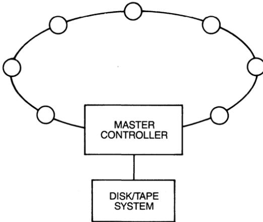
**Figure 1-21** Loop-type network with shared mass storage.
