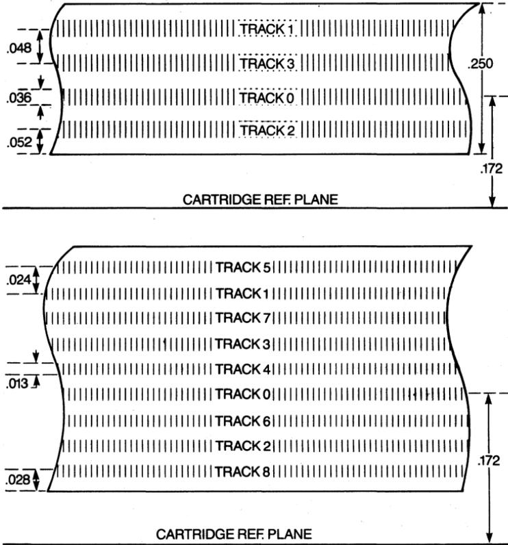
**Figure 9-4** Track dimensions, 1/4-inch cartridge tape.
