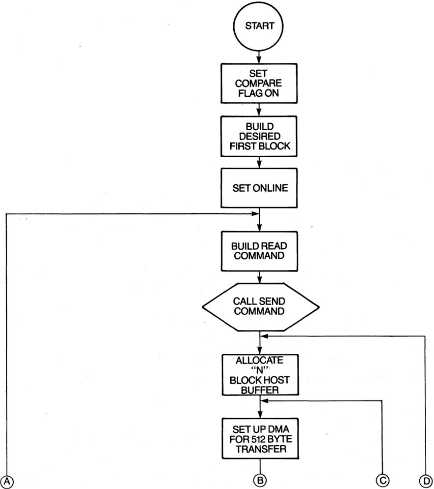
Figure 6-12 Flow diagram, read file with first-block ID.
