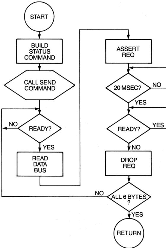
**Figure 6-2 Flow diagram, read status.**
