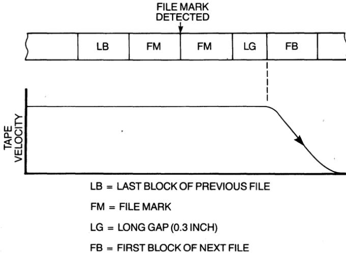
**Figure 9-34 Tape motion, Read-File-Mark Sequence.**
