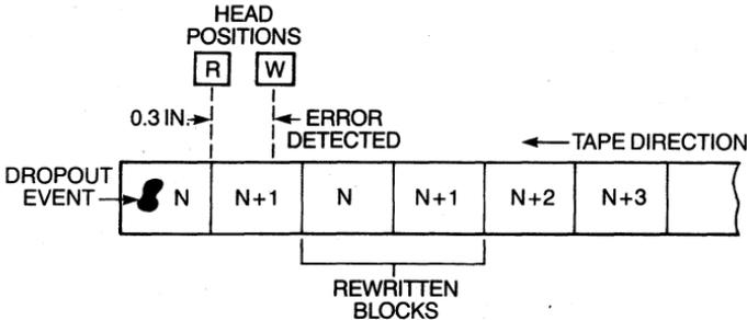
**Figure 5-18 Correction by rewriting BIE (block in error).**
