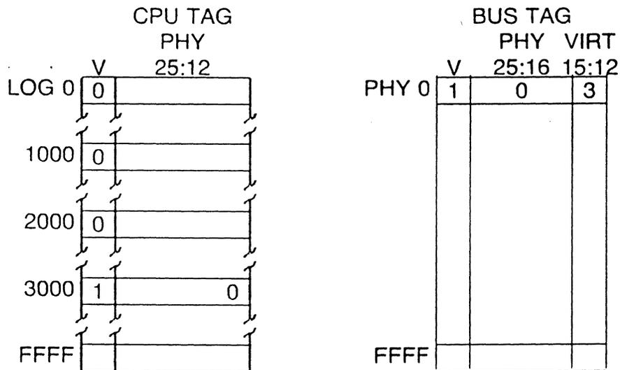
Figure 3-4. Cache Fill: Read Virtual 3000 And Physical 0
