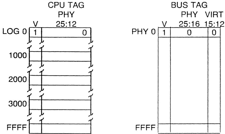
Figure 3-1. Cache Fill: Read Virtual 0 And Physical 0
