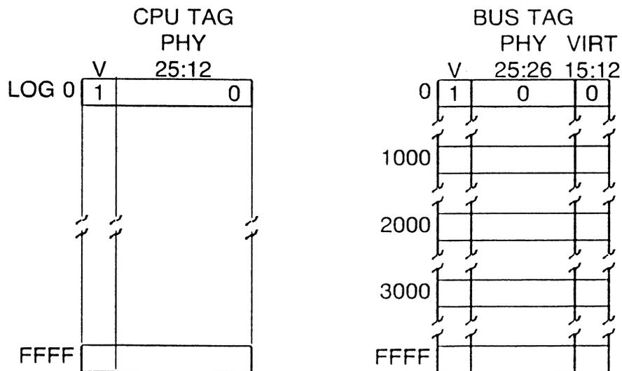
Figure 3-5. Cache Fill: Read Virtual 0 And Physical 0
