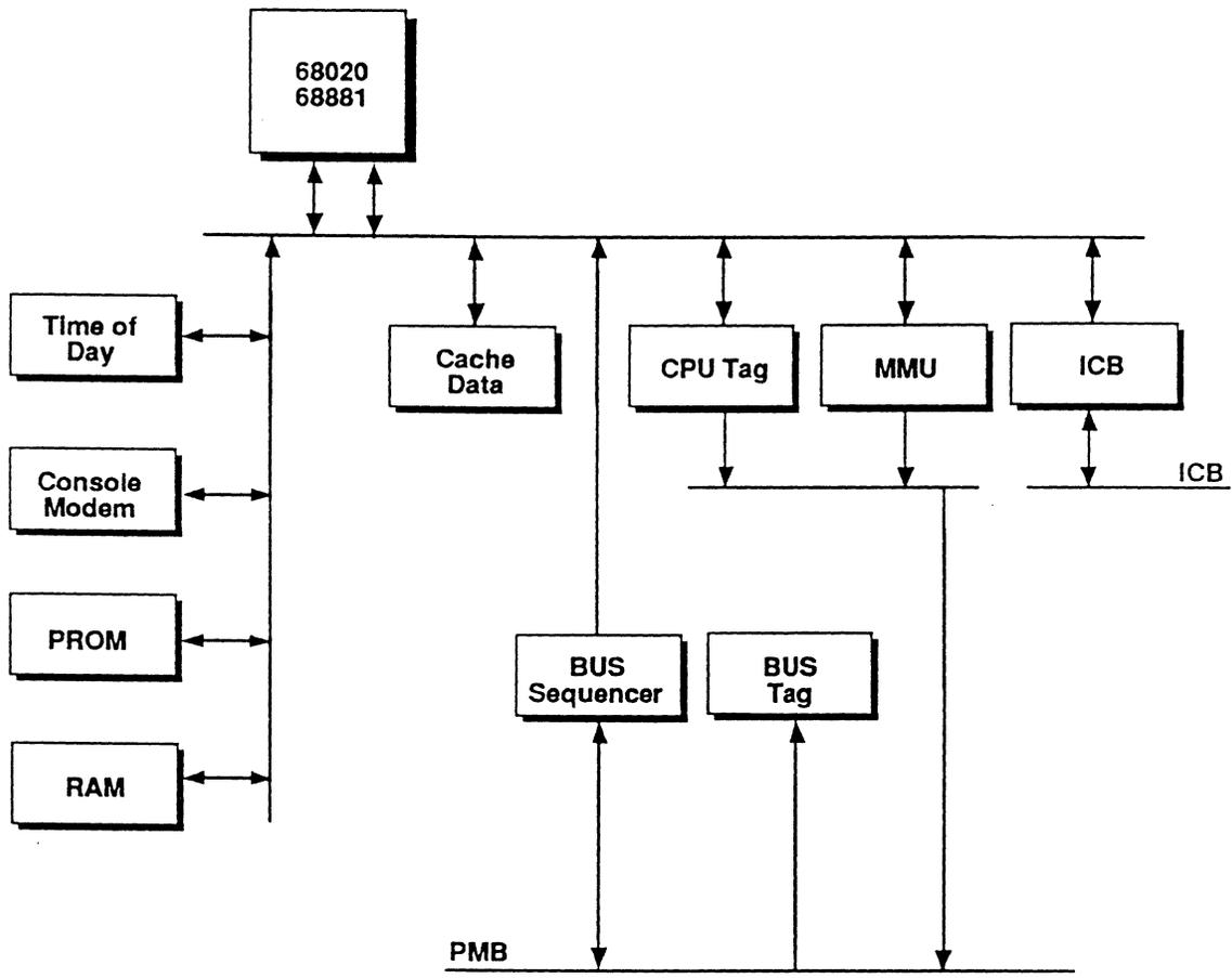
Figure 1-1. CPU32/25 Block Diagram
