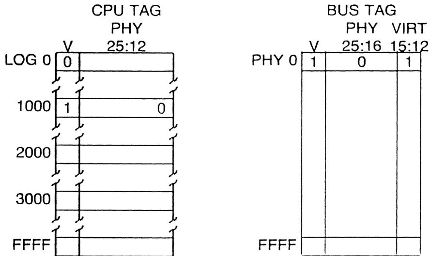
Figure 3-2. Cache Fill: Read Virtual 1000 And Physical 0
