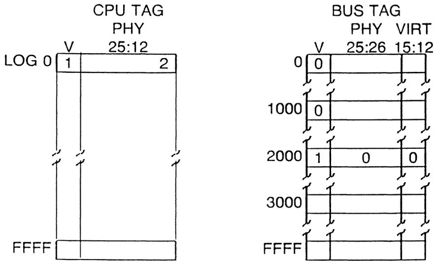
Figure 3-7. Cache Fill: Read Virtual 0 And Physical 2000
