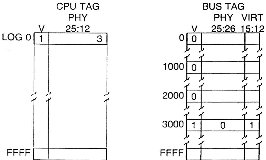
Figure 3-8. Cache Fill: Read Virtual 0 and Physical 3000
