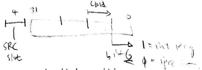
The cmd-pend bit goes to 0 when the processor resets it by writing at CLR NMI. Separately, a write to INC\_READY is required to allow more commands.
