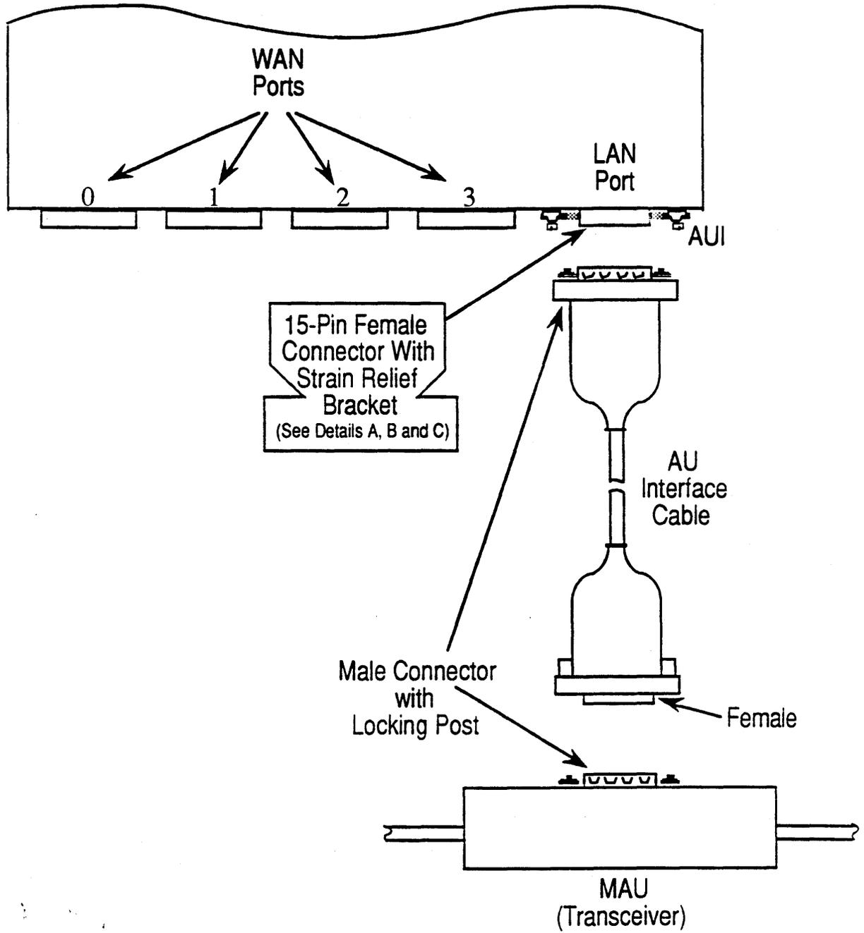
Figure B-3 LWDB Connector Hardware and AUI Cable Detail
