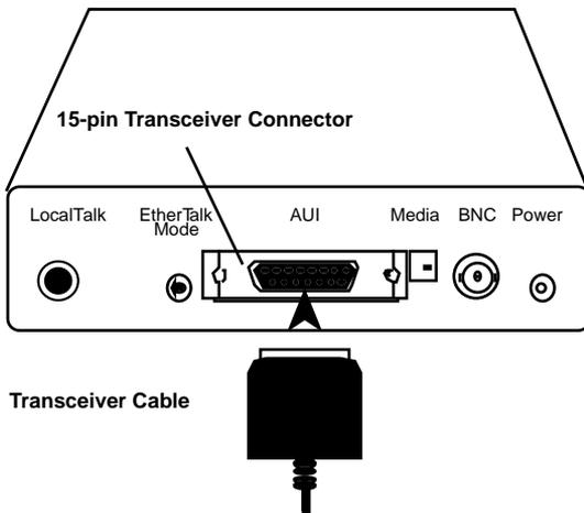
**Figure 2-2** Connecting the 15-pin transceiver to the AsantéPrint unit
