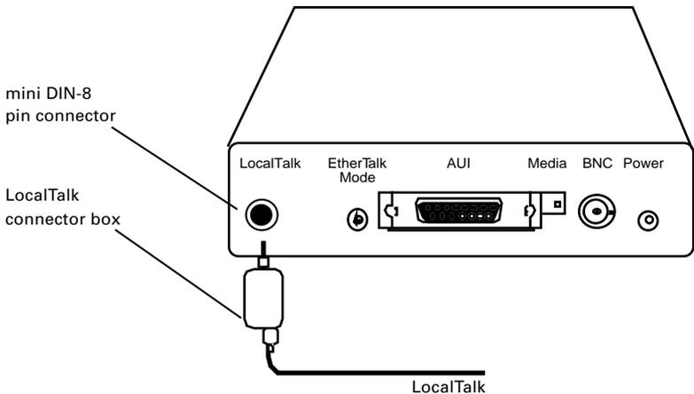
**Figure 2-8** Connecting the LocalTalk connection box
