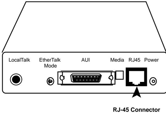
**Figure 2-6** RJ-45 connector on the AsantéPrint unit
