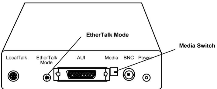
Figure 2-1 EtherTalk Mode rotary switch and media switch
