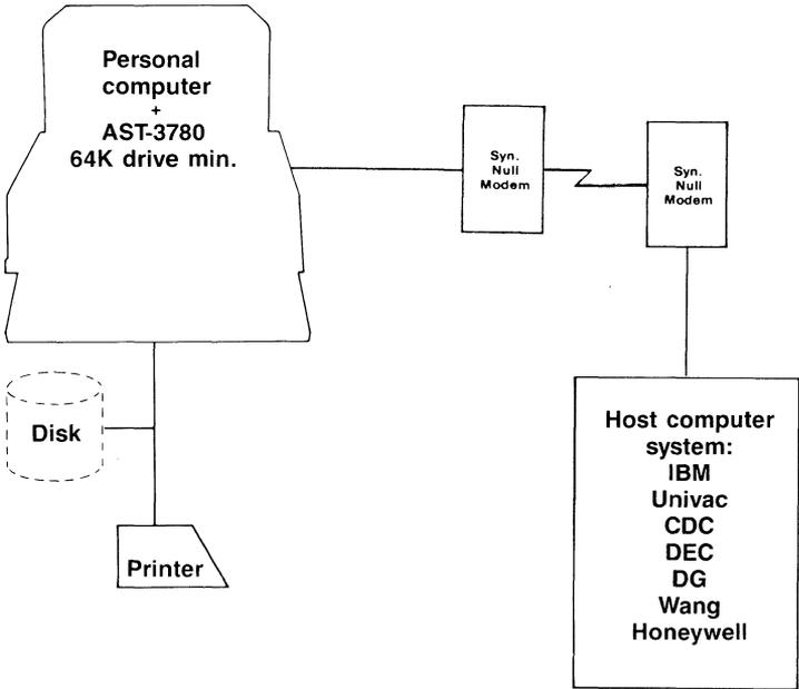
Figure 3. Remote Connection Using a Modem.
