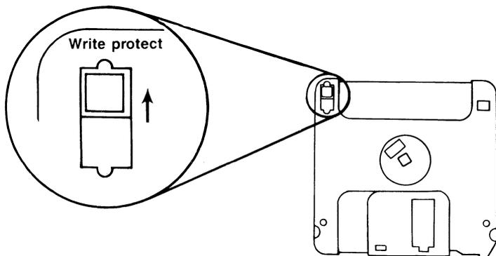
**Figure 2-1. Write Protecting a Diskette.**
