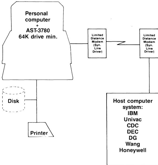
Figure 2. Local Connection Using a Limited Distance Modem.
