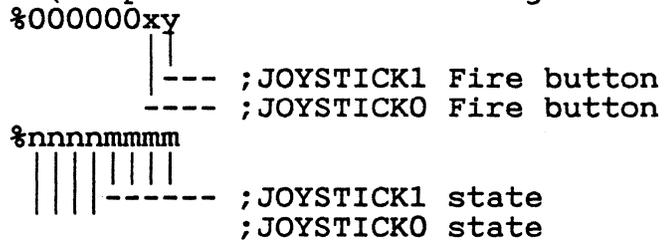
Sets the ikbd to do nothing but monitor the serial command line, maintain the time-of-day clock, and monitor the joystick. The rate sets the interval between joystick samples.
