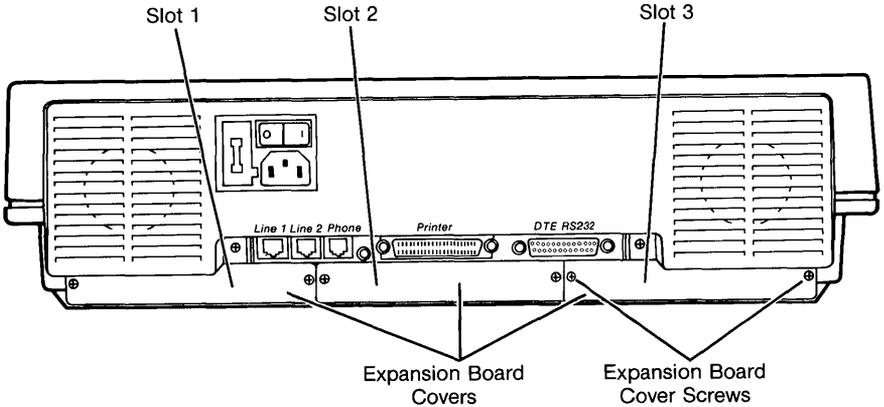
Figure 3 Rear View of UNIX PC
