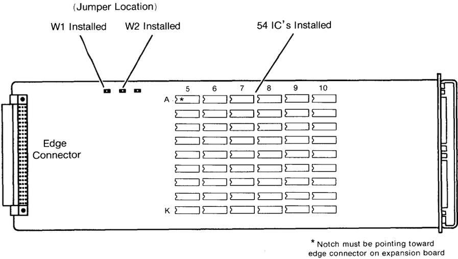
Figure 2 One and One Half MB Expansion IC Location
