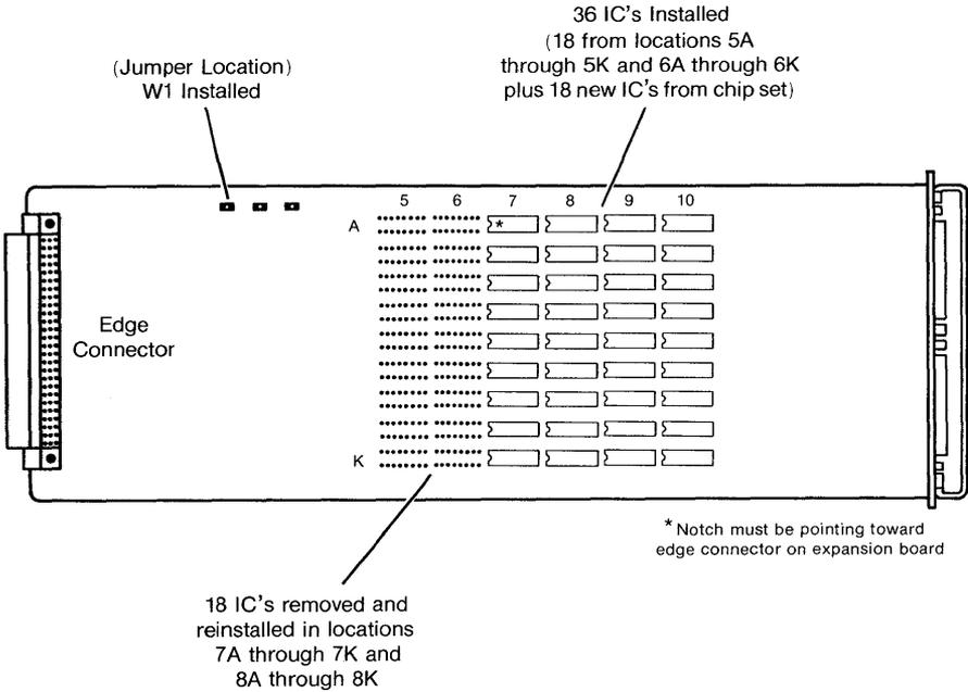
**Figure 1 One MB Expansion IC Installation Location**
