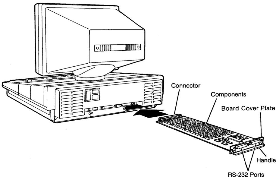
**Figure 4 Inserting an Expansion Board**
