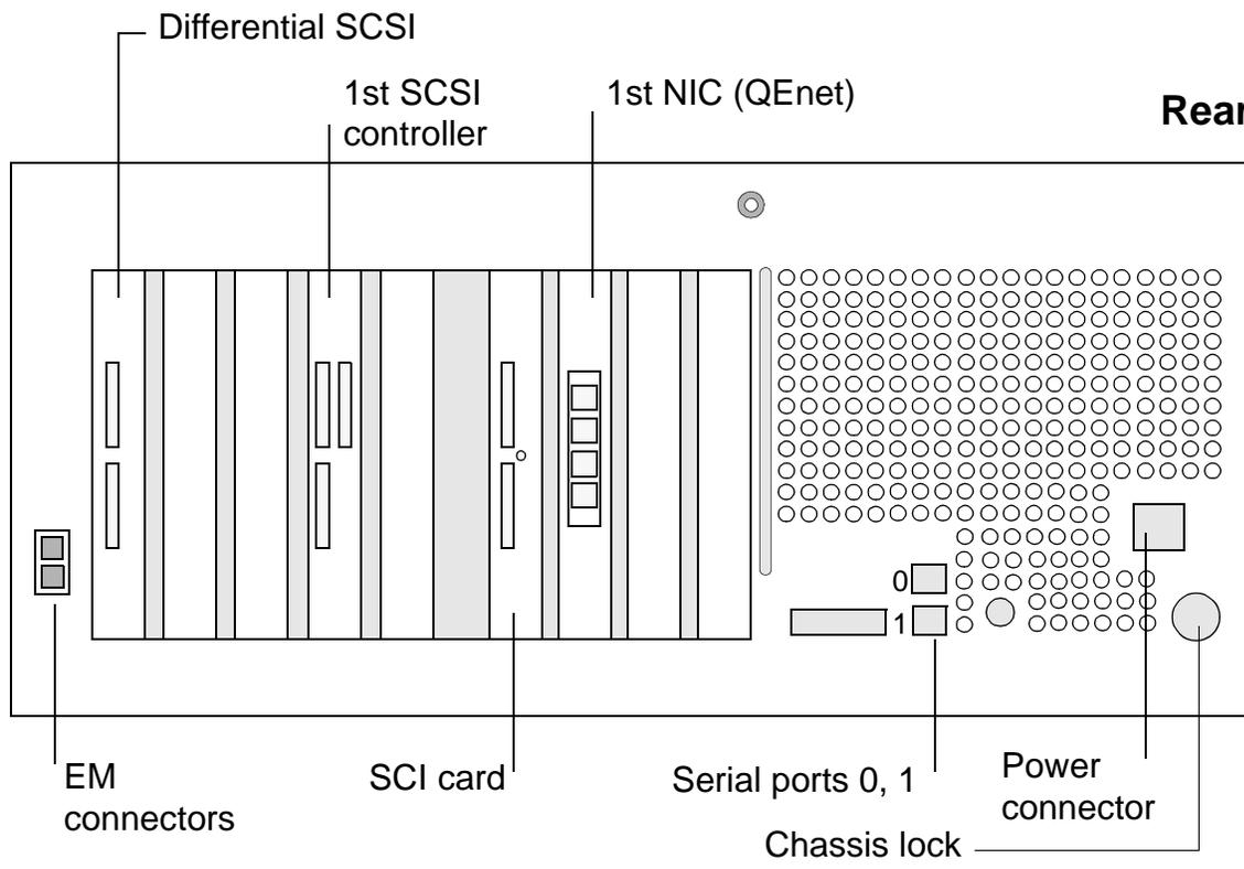
**E-Box module (front, rear; rear bezel removed)**
