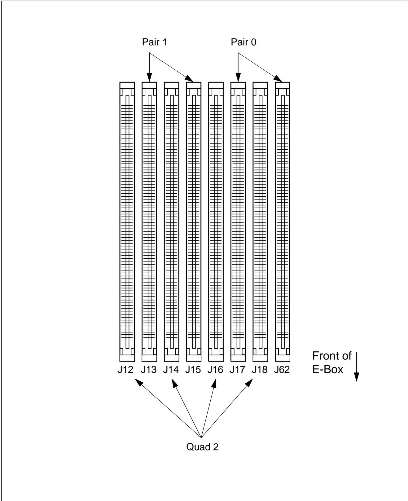
**ECHaP DIMM sockets pair/quad assignments**
