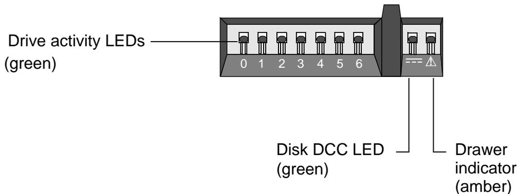
**HDDA front panel LEDs**
