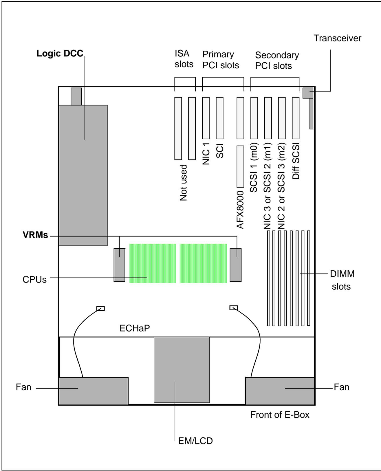
**Voltage Regulator Module and Logic DCC**
