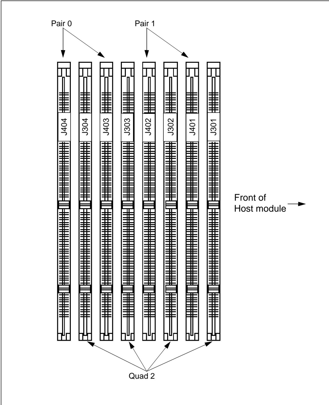
**Host DIMM sockets pair/quad assignments**
