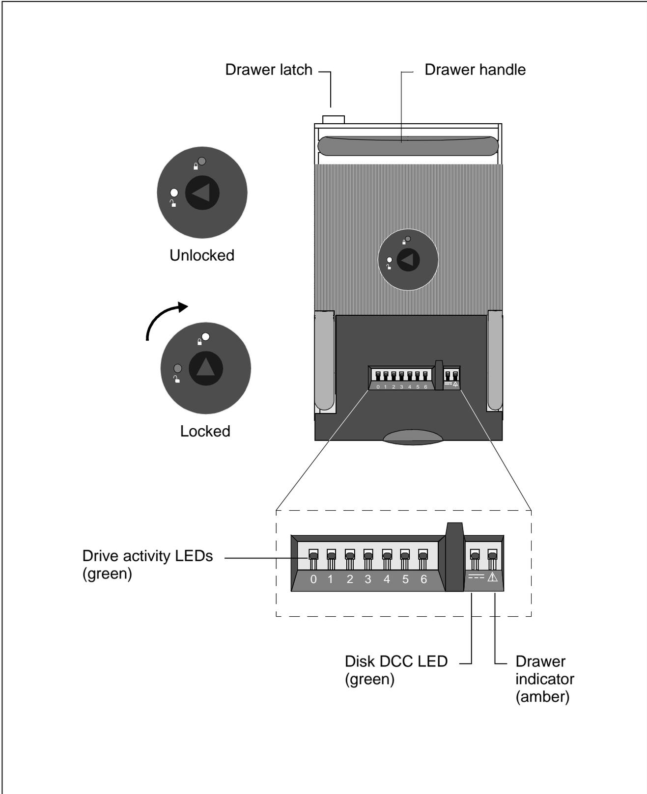
**HDDA drive drawer lock and lower bezel detail**
