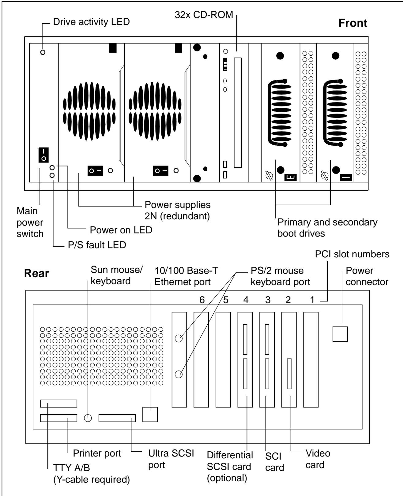
**Host module (front, rear; bezels removed)**
