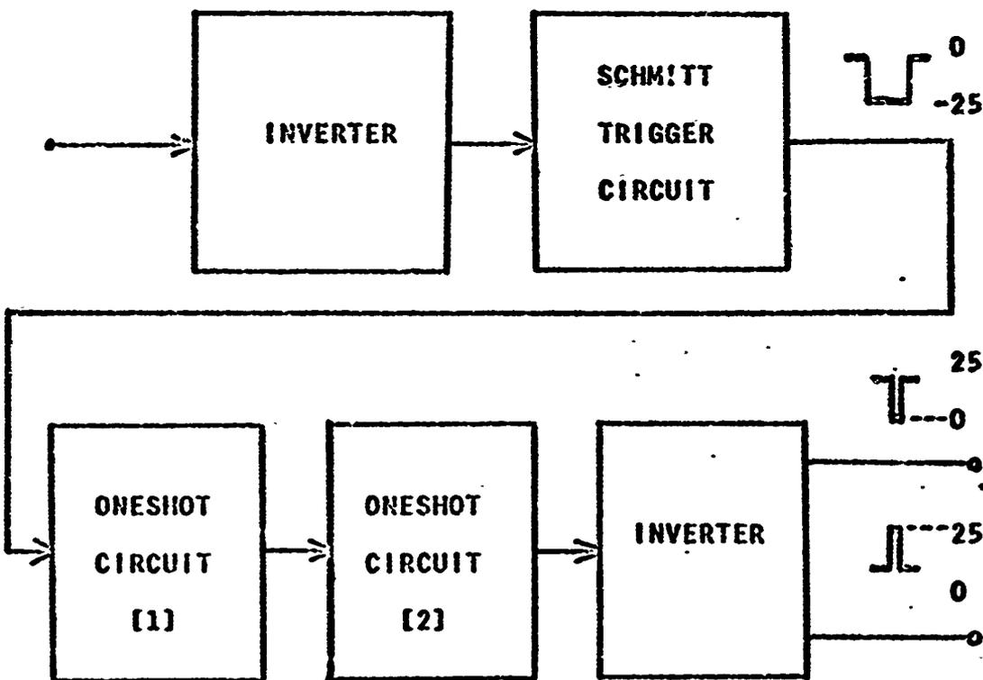
Figure 18. Block diagram of the Flexwriter to D17B interface.
