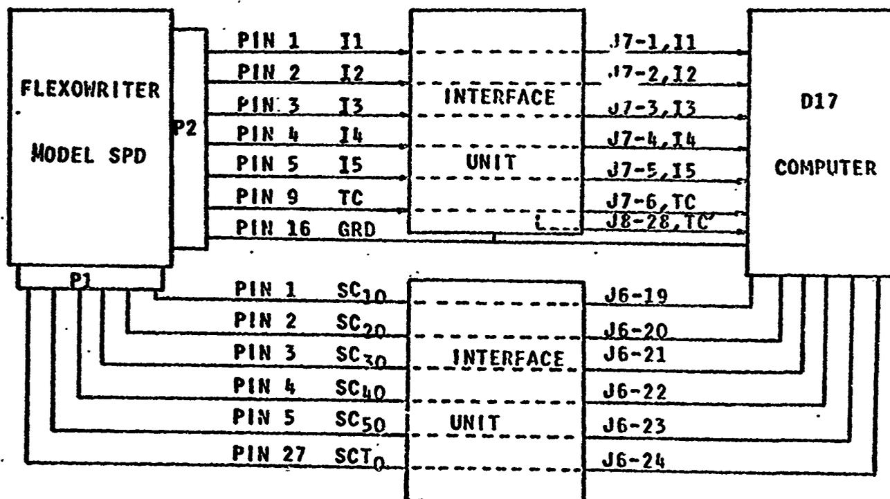
Figure 17. Schematic diagram of the Flexowriter-D17B interface.
