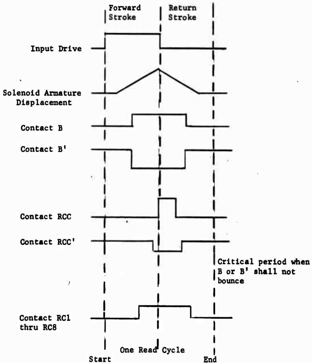
Figure 16. Mechanical Reader Timing Sequence
