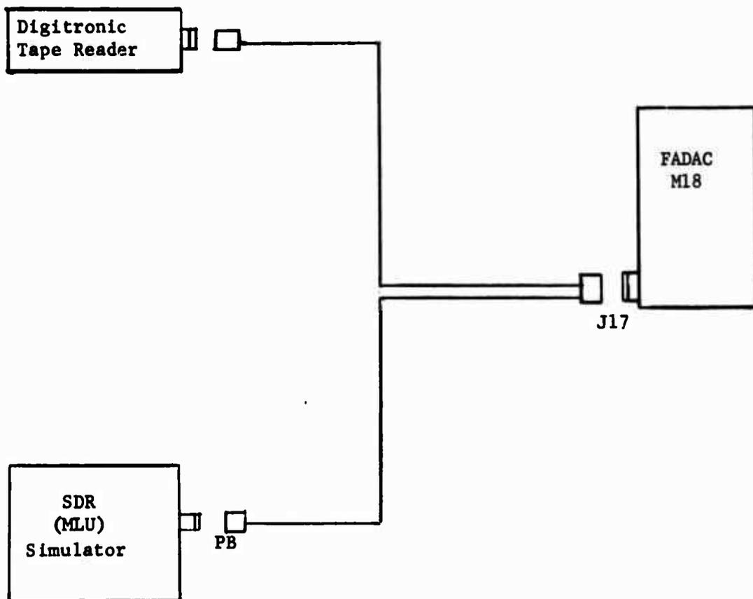
Figure 50. FADAC to Digitronic Reader Cabling
