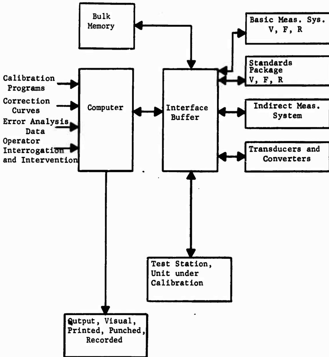
Figure 59. AutoCal Systems Concept
