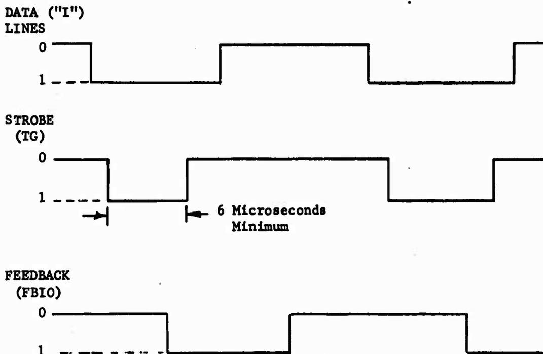
Figure 30. Input Line Timing
