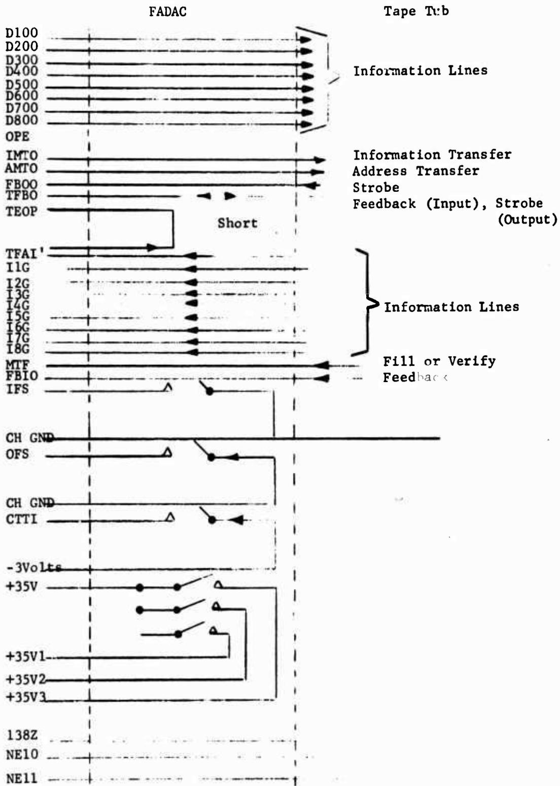
Figure 56. FADAC - Tape Tub Interface
