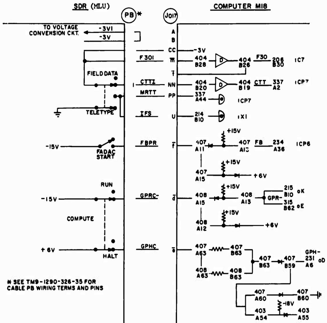
Figure 47. Memory Loading Unit (MLU) to FADAC Signals (Part 1)
