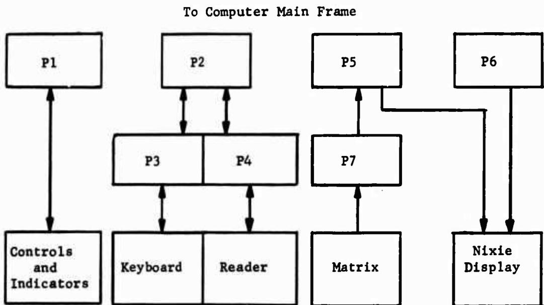
Figure 9. Control Panel Functions and Connector Assignments
