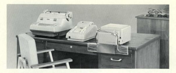
**OPERATING FEATURES** Conventional 10-key keyboard — Simple, handspan operation for easy use. Void key to correct errors — Backspace key or Clear before entry, cancels punching. Parity feedback circuits for punching accuracy — Selfcontained mechanism verifies punched tape accuracy. Convenient tape holders — Transparent holders guide tape into punch and catch chad, provide visual check on tape supply. Remote use — Punch unit will operate in separate area to isolate punch sounds.
