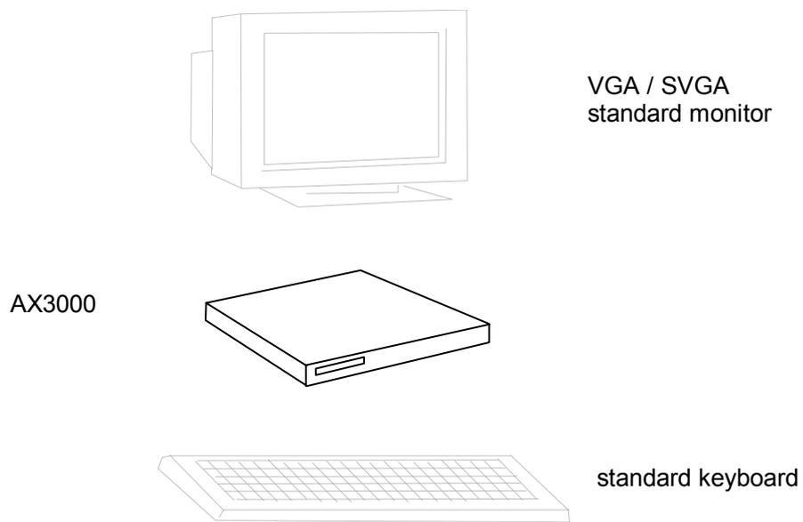
The AX3000 is totally designed and manufactured by Axel. The terminal's electronics is contained within a slim base unit which provides connections for a VGA or SVGA monitor, keyboard, system printer, serial devices and Ethernet network.
