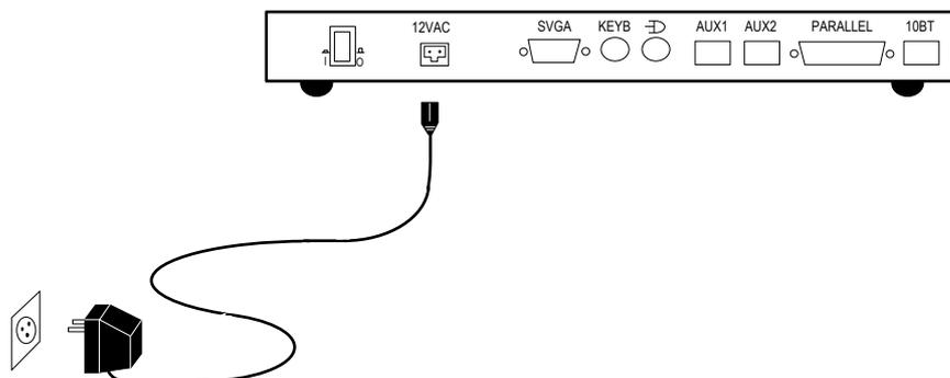
**Warning: Only use the Axel external transformer supplied with your AX3000 Model 75E. Use of any other transformer may cause permanent damage to the AX3000.**
