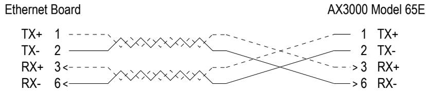
**IMPORTANT:** the cable is composed of two twisted pairs. The two wires TX+ / TX- must belong to one pair and the two wires RX+ / RX- must belong to the other pair.
