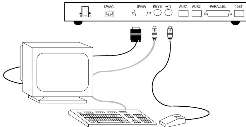
If your keyboard is fitted with a DIN connector, connect it using a DIN-to-Mini-DIN adaptor.
