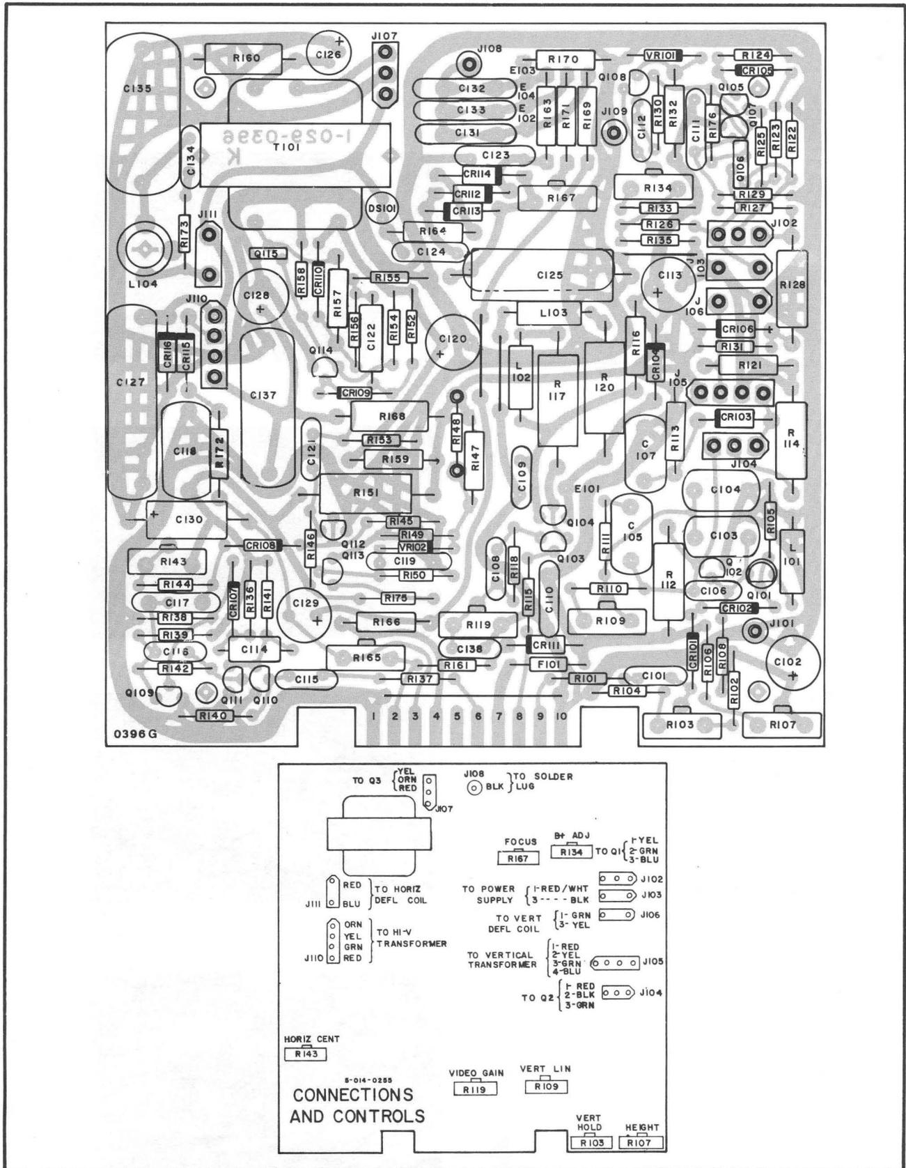
Fig. 5-1 Circuit Board Component Location and Intercabling Diagram.
