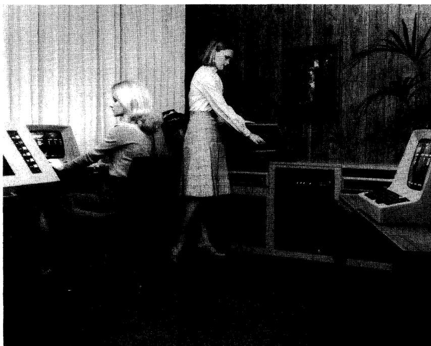
*Model 700 is the latest addition to the Basic/Four line. Included in the minimum-configuration system are 64K bytes of MOS memory, 4 video display terminals, a 300 line-per-minute printer, and 150 million bytes of disk storage. Purchase price is \$115,000.*
