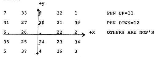
Moving in the +X direction slews paper on to the floor. +Y direction is arranged so that the coordinate system is right handed.
