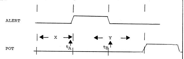
The general rule on timing of the ALERT, POT, and PIN strobes is that they rise at the end of the instruction\* during which the special condition is executed, and they fall at the end of the first interval\* during which the special condition does not exist. Thus it is possible to generate arbitrarily long strobes, but this should be avoided.
