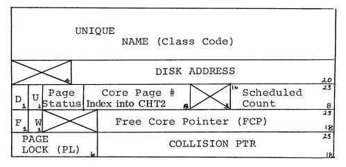
Core page address is given by index of entry
