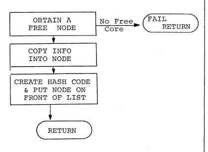
The CHT collision lists are of type 3 (see appendix). This is to facilitate removal of nodes from the free core list.
