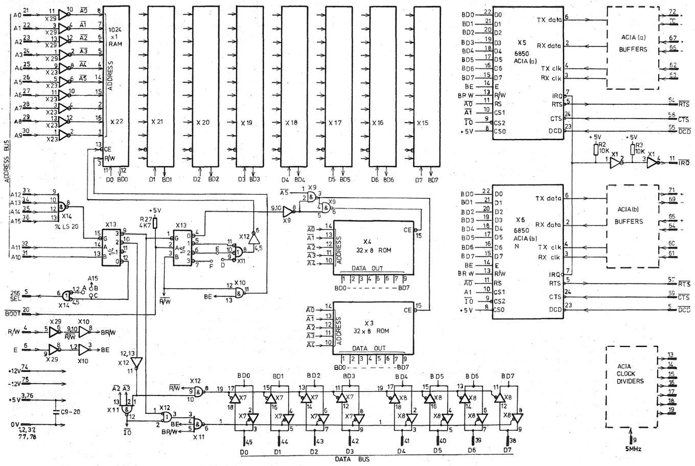
and selection of the appropriate memory depends upon the setting of a 'Boot' switch (connected between card pin 20 and OV), and whether the CPU is doing a Read or a Write.
