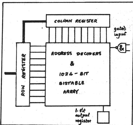
Figure 2. Block diagram of bistable store.
