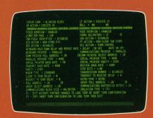
Beehive's unique Terminal Configuration Manager (TCM) allows the Micro 4400 to be configured from the keyboard. After storing in EAROM there is no need for reconfiguration
