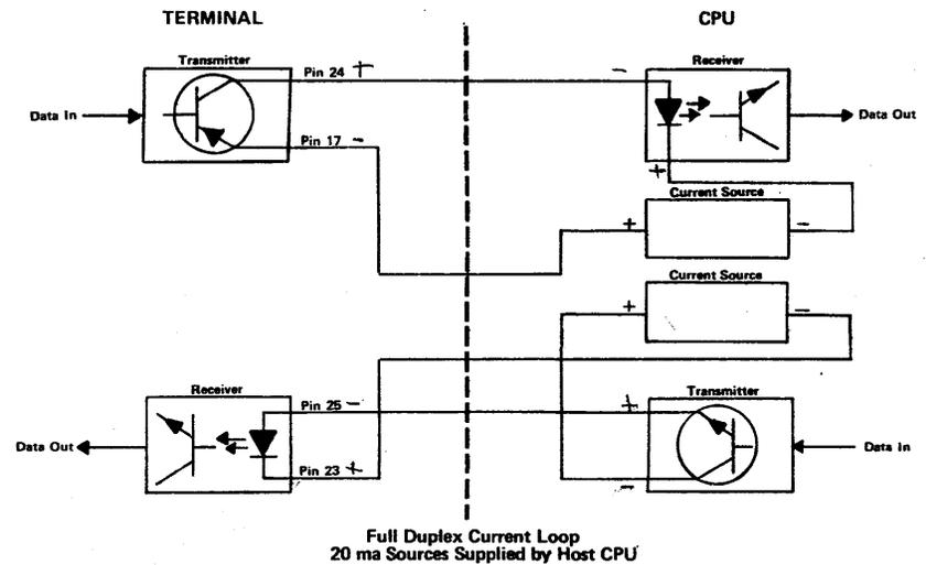
Figure 2-2 Current Loop Cabling
