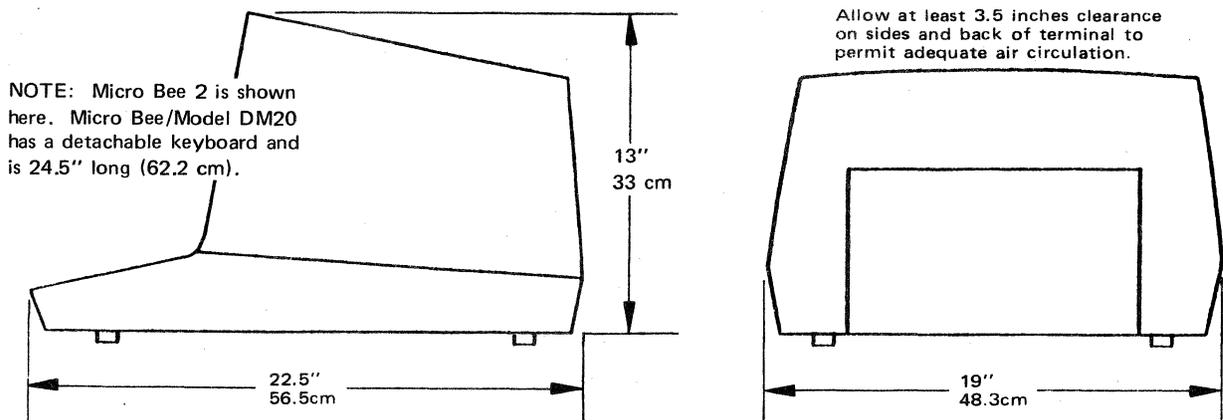
Figure 2-1 Mounting Requirements
