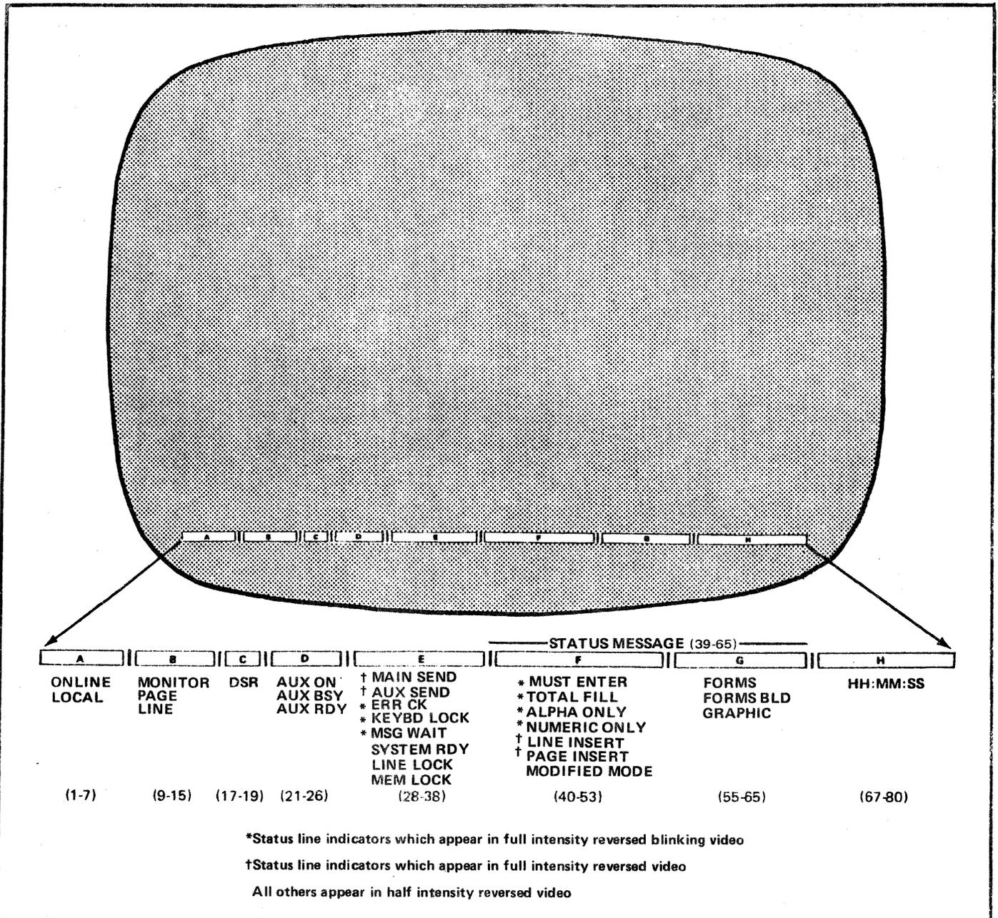
The status line is an invaluable ready-reference tool which enables the operator to tell at a glance which operating modes/features are currently in use on the DM 30, and whether the terminal is operating correctly.
