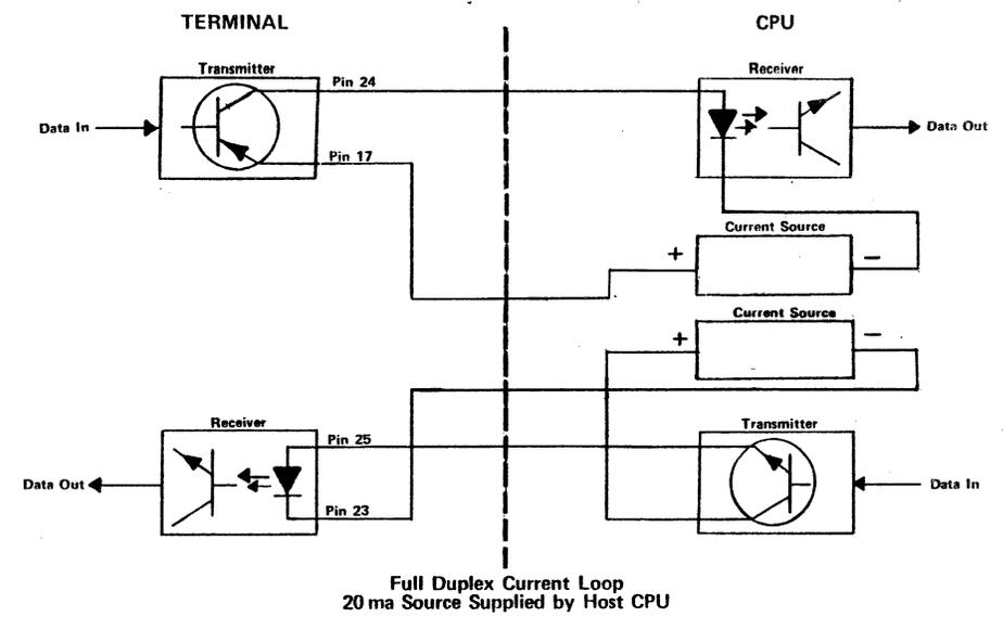
Figure 2-2 Current Loop Cabling
