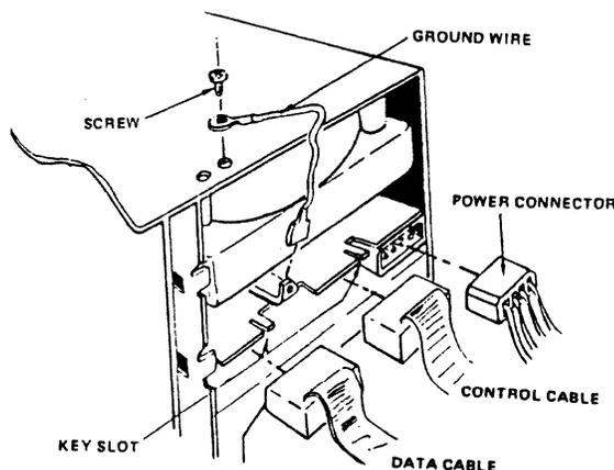
Figure 11. Cable Connections to Peripheral Device
