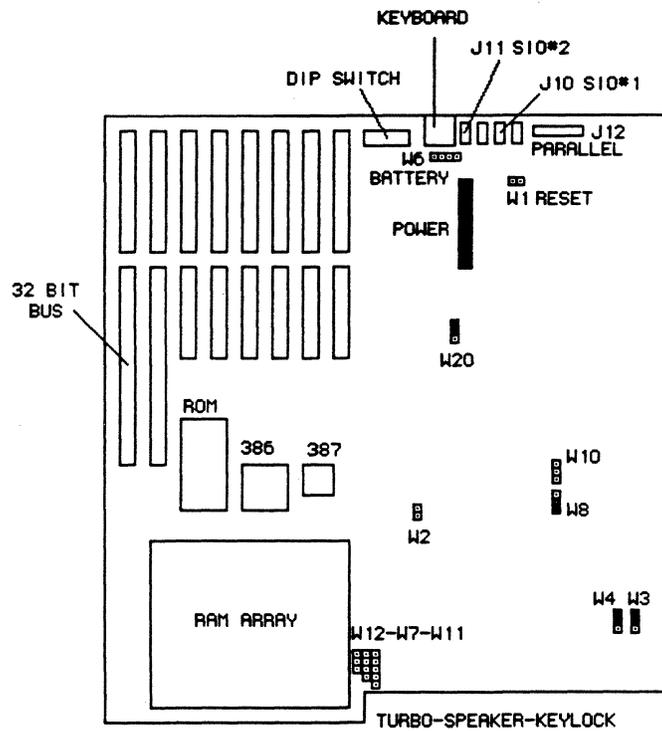
Figure 15. Locations of Items on System Board
