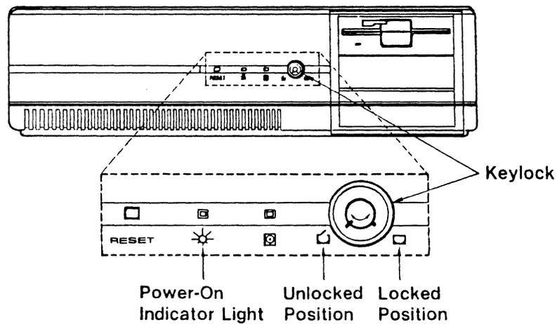
Figure 1. Front Panel and Key Lock
