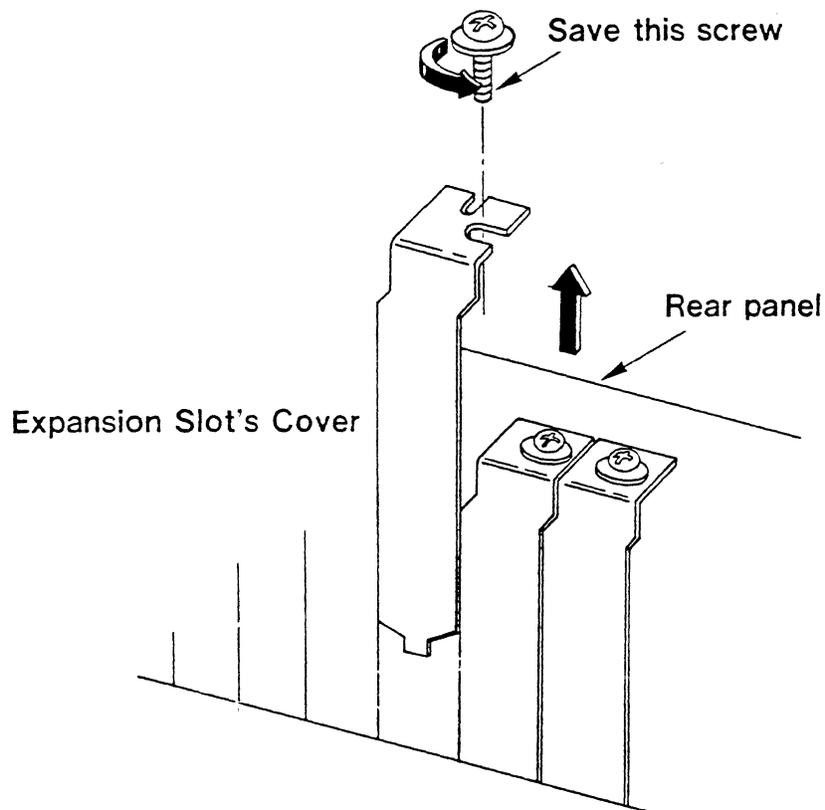
Figure 5. Remove the Expansion Slot Cover
