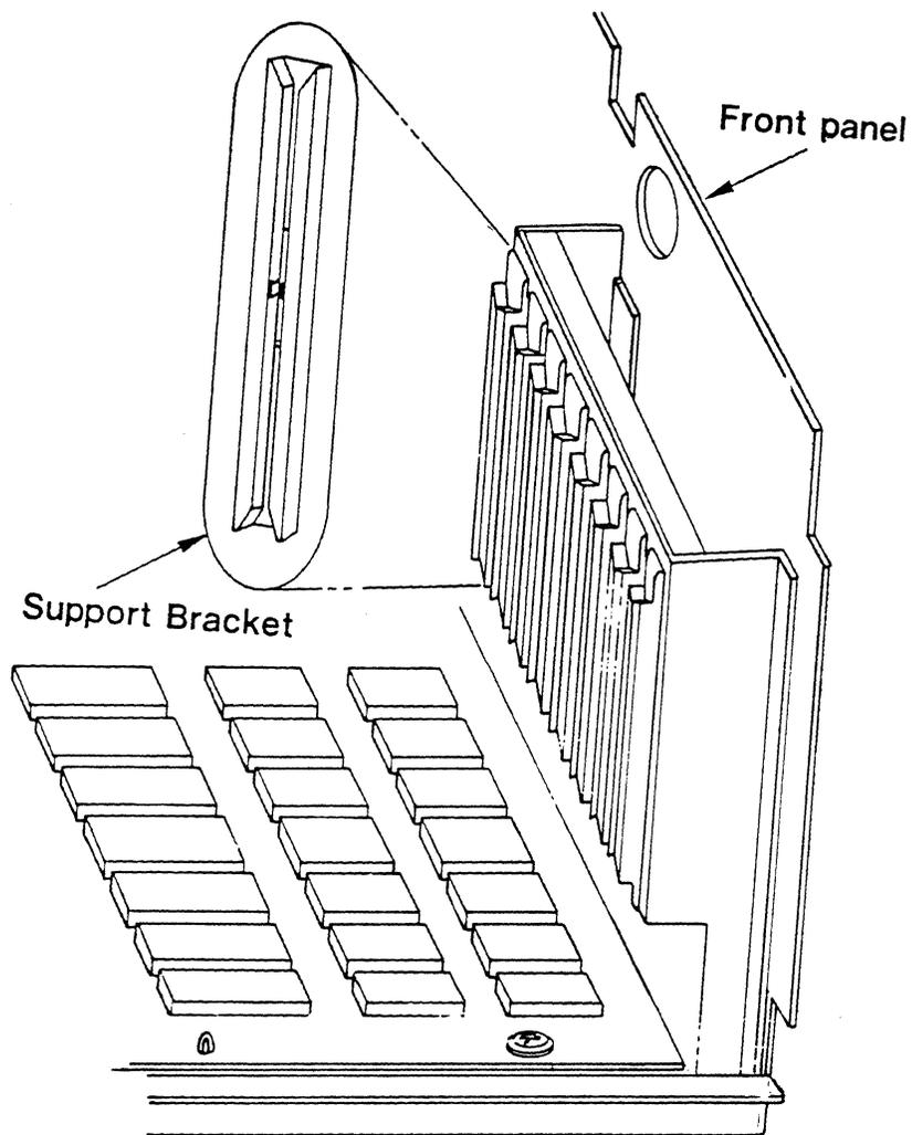
Figure 7. Card Edge Supporting Slide
