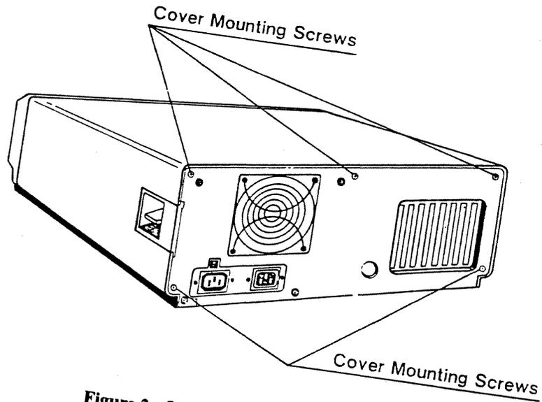
Figure 2. Cover Mounting Screws
