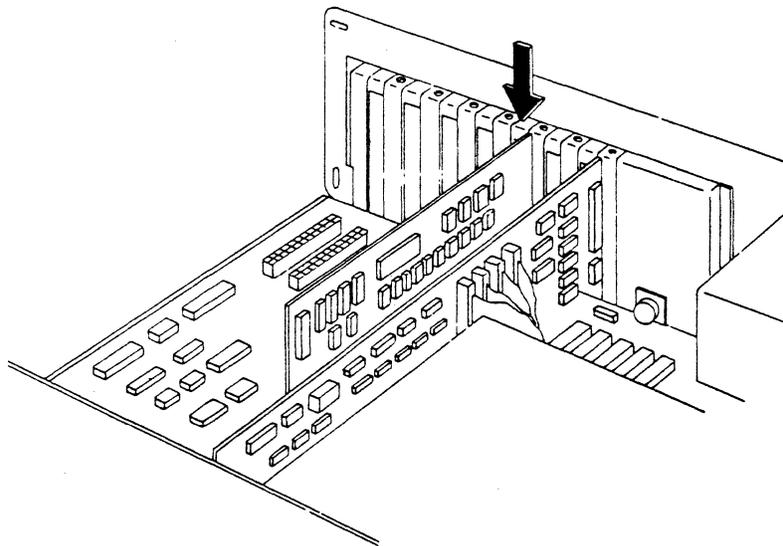
**Figure 8. Press Firmly on the Option Card**
