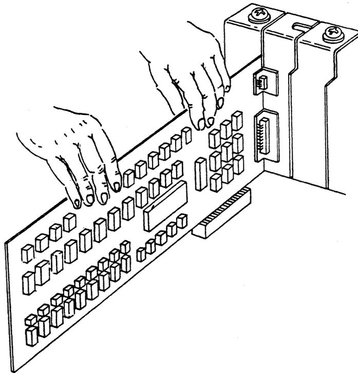
Figure 6. Installing an Option Card
