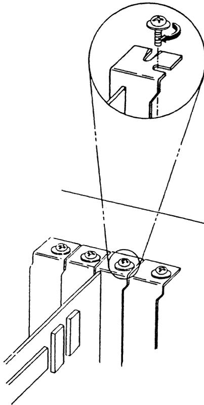
Figure 9. Replace the Bracket Screw
