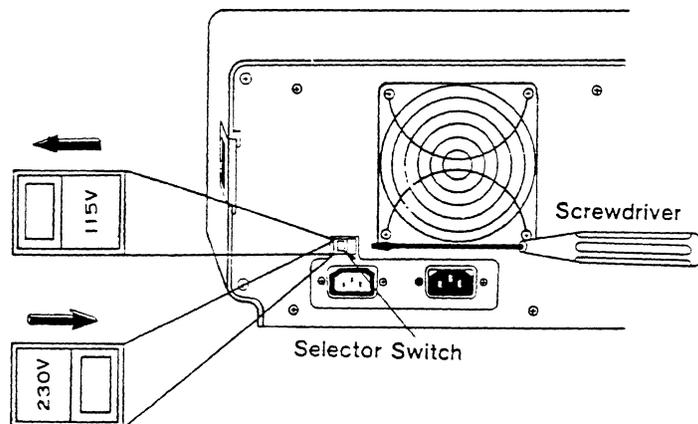
**Figure 12.** Set the Voltage Selector Switch
