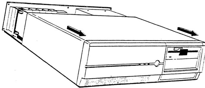
Figure 3. Removing the Cover
