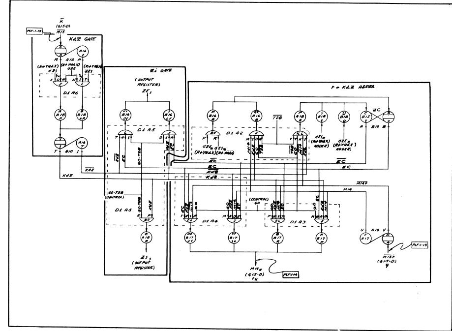
Figure 27. Schematic, r + Kdz Adder
