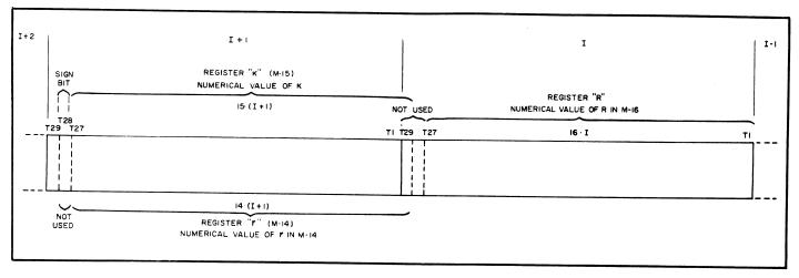
Figure 20. Location and Word Structure of K, R and "r" Registers
