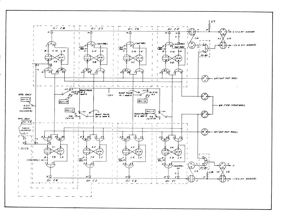
Figure 34. Schematic, dx Counter & Register
