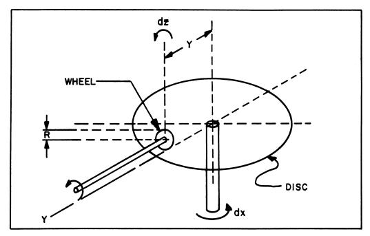
Figure 8. Mechanical Integrator
