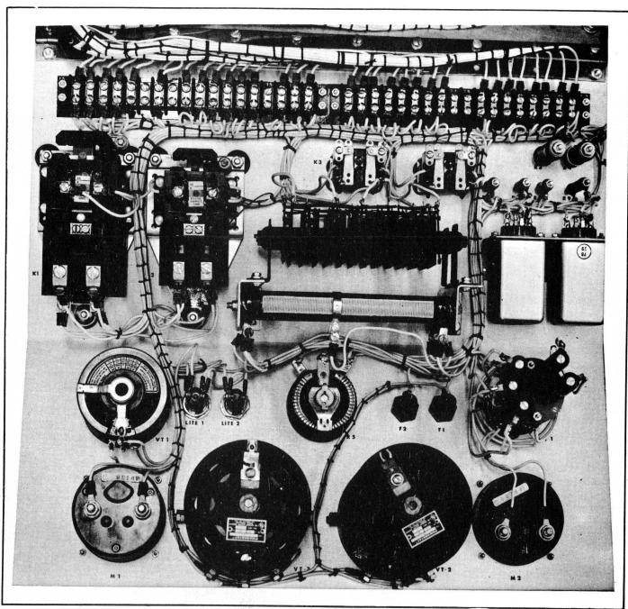
Figure 37. Power Supply, Hinged Panel, Open
