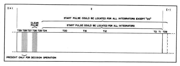
Figure 19. One Word Structure of Line ML8
