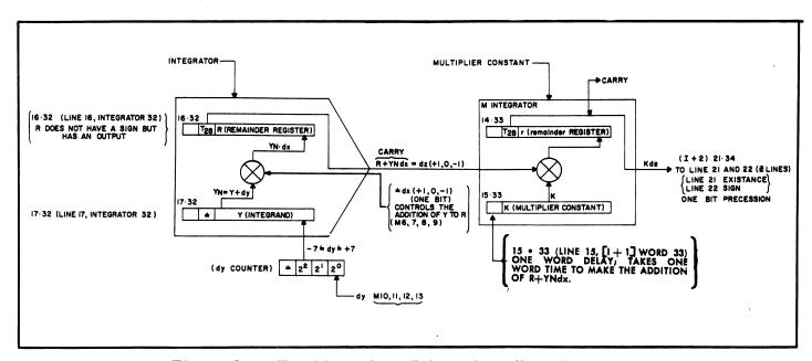
Figure 13. Function of an Integrator, No. 32
