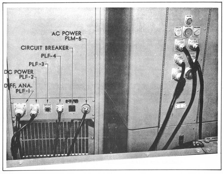
Figure 6. DA-1, G-15 Interconnecting Cables
