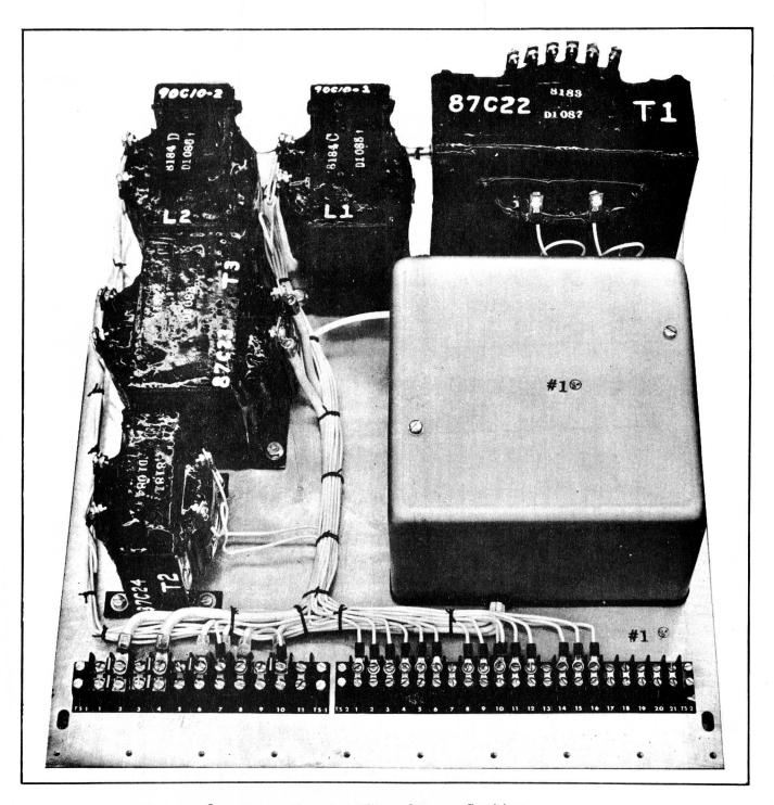
Figure 38. Power Supply, Transformer Section
