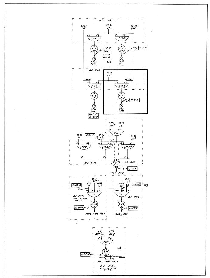
Figure 30. Schematic, Magnetic Tape Control, G-15, 3D597 (Blocked Area)
