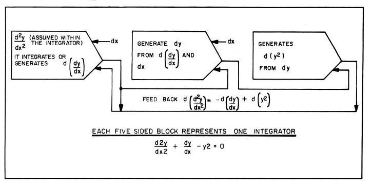
Figure 3. Simplified Diagram Integrator Connections
