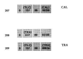
The TLC command transmits the "Call" to the Control Console with call number 250. The Control Console answers GRN and enters the CALLED state.
