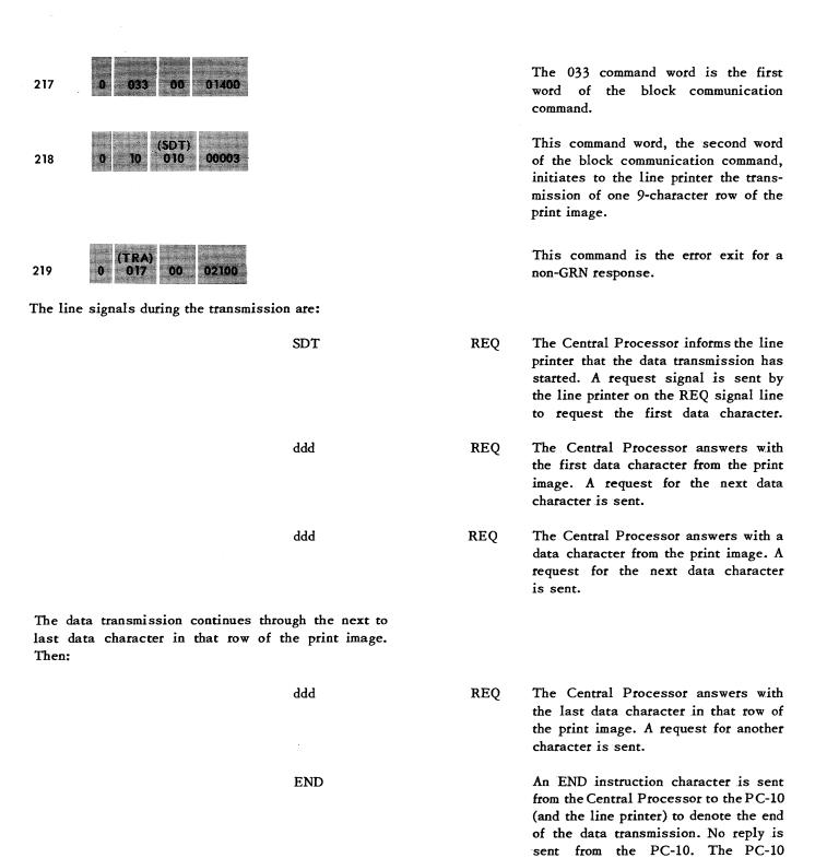
As shown above, the block command causes the Central Processor to automatically transmit to the PC-10 the twelve 8-bit characters found in locations 1400, 1401 and 1402. The first nine characters are
