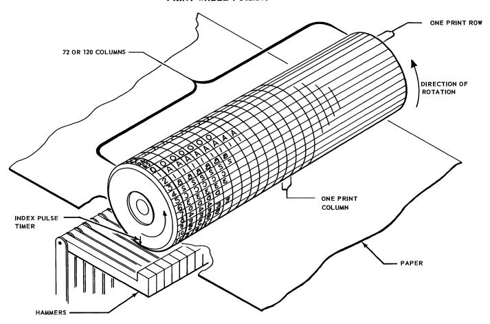
the third hammer is activated when the B row of the print wheel is in place and the second hammer is activated when the C row of the print wheel is in place. Thus the print wheel must make one complete revolution to print one line of print.
