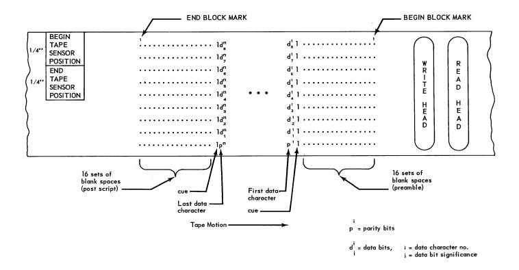
The End of Tape and Beginning of Tape indicators are pieces of one inch by one-quarter inch reflective tape attached to the end and the beginning of the tape. These indicators are sensed by the End of Tape and Beginning of Tape sensors, the condition of which can be ascertained by command.
