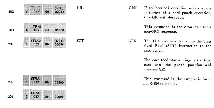
The last TRA command transfers the Central Processor away from the input output program to another portion of the program while the card punch is positioning the first card. When the card is positioned, an interrupt will be sent to the Central Processor from the PC-10. The interrupt will be processed and the Central Processor will return (under program control) to the input/output program.
