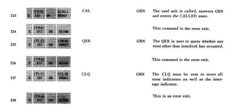
At this point the programmer can set up the counter to count the number of cards to be processed. In this example the counter will count three words. After the necessary bookkeeping, the programmer has some time left before the interrupt occurs for the next row. When the interrupt occurs, the program should transfer back to location 207 to initiate the punching of the next row.
