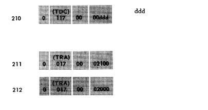
GRN The TDC command transmits the next data character to be typed out to the Control Console. The Control Console answers GRN.
