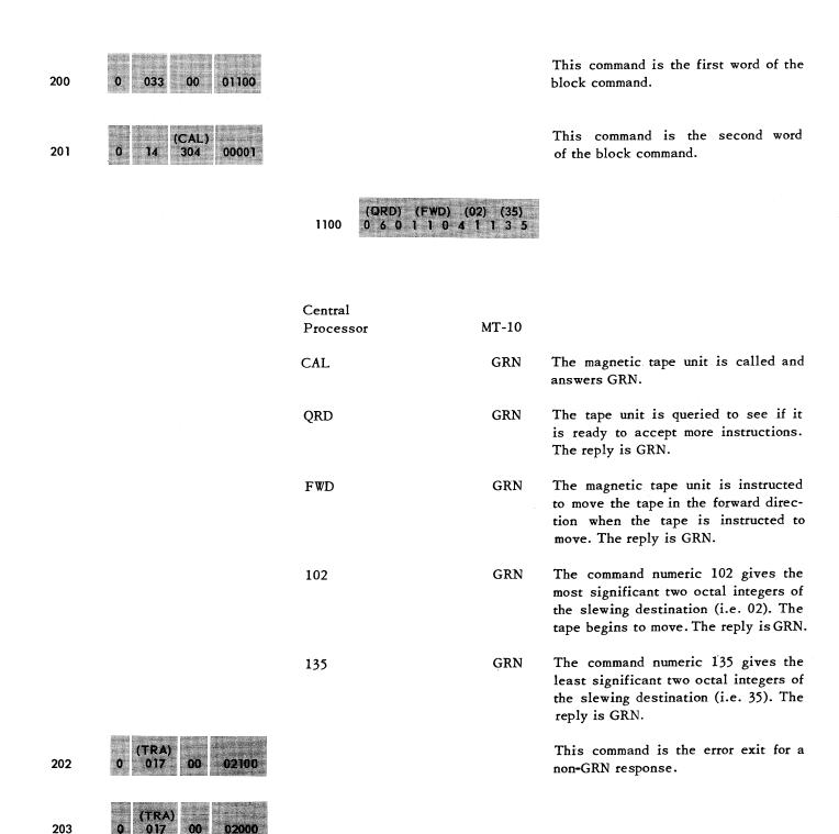
The Central Processor returns to another program. When the magnetic tape unit completes the slewing operation, the unit transmits an interrupt to the Central Processor.
