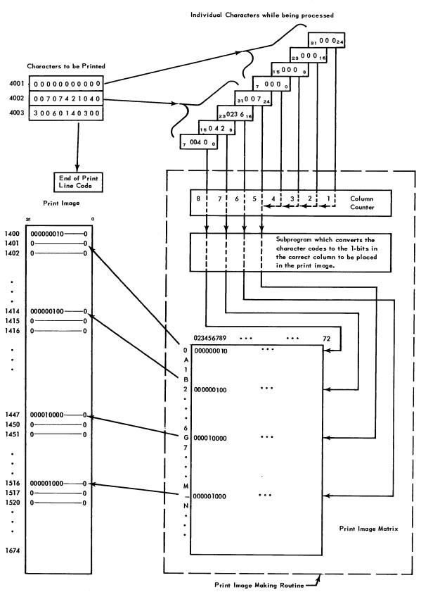
The preceding figure gives a schematic representation of the first print image constructed by the example program. Only the print image for the line print "G-20" is shown. In the upper left part of the figure in 4001 are shown the set of four all zero 8-bit characters which represent the four spaces to be left on the page of print; in 4002 are shown the four characters which
