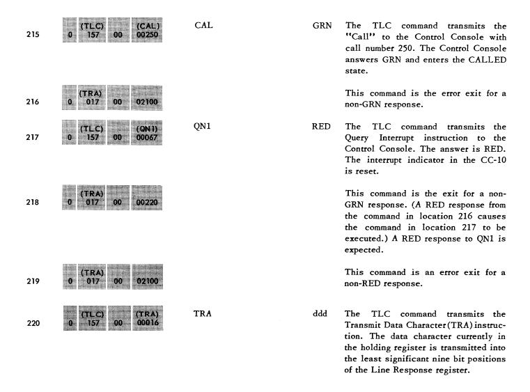
The input character is in the Line Response register and can be used as the programmer desires.
