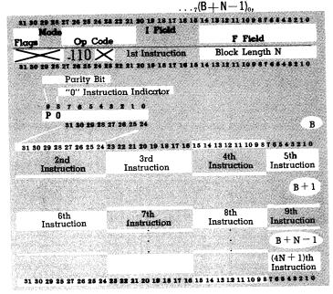
When a Block Transmit Instruction is processed, 8-bit instructions are transmitted to the specific piece of equipment starting with the 8-bit instruction in the second word of the Block Operator command, taking the next from location B, and continuing through location B+N-1 where N is the block length. A GRN is received from the external equipment acknowledging receipt of a proper instruction.
