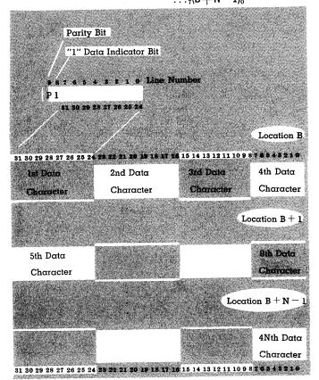
Upon receipt of REQ the response from the instruction in bits 15 through 22 of the second word of the Block Transmit Data Command, 8-bit data characters are transmitted to that piece of equipment starting with location B and continuing through location B+N-1, where N is the block length. An REQ is received from the external equipment before the transmission of each data character.
