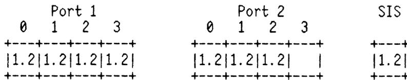
a. Port 1 request for SIS and configure it to Port 3. Note that the SIS will overlay the existing unit of 1.2MB and make it temporarily inaccessible.
