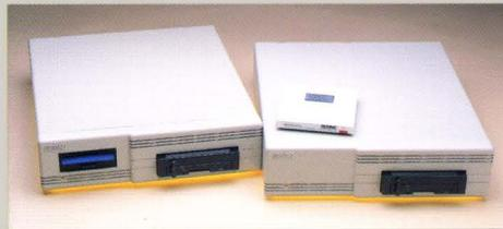
Packed in a small 10-MB cartridge, the removable hard disk delivers performance, security, and flexibility over tapes.
