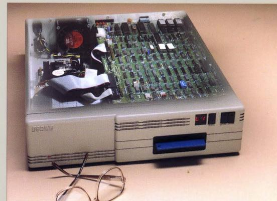
Modular design, compact packaging, and extensive self-diagnostics are standard features of the Series 8000.
