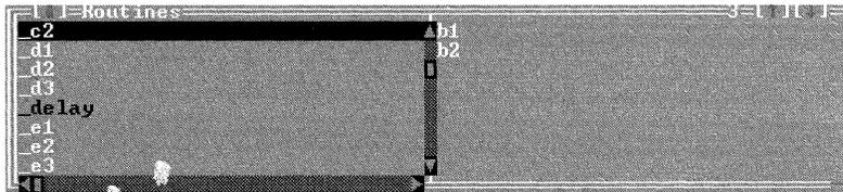
The Routines window is divided into two panes. The left pane lists routines global to your whole profiled program, and the right pane lists routines that are local to the current module of the program you’re profiling.
