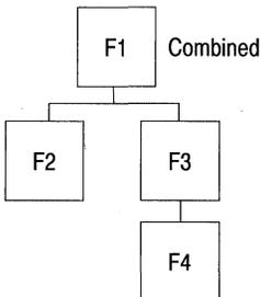
In this illustration, the routine *F1* has its Timing set to Combined. Turbo Profiler collects the timing information for all the routines (*F1*, *F2*, *F3*, and *F4*), and sums them into the timing information collected for the routine *F1*.
