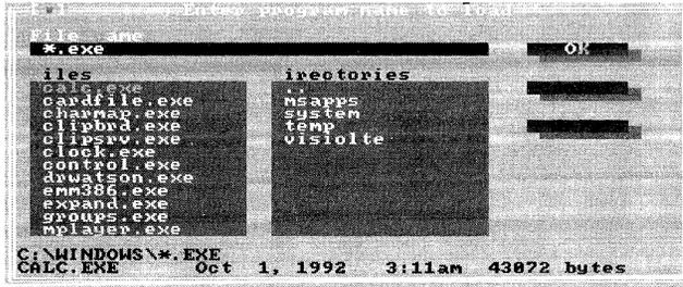
The Files list box displays the files in the currently selected directory. By entering a file mask into the File Name input box (such as *\*.EXE*), you can specify which files should be listed. You can also use the File Name input box to change disk drives.
