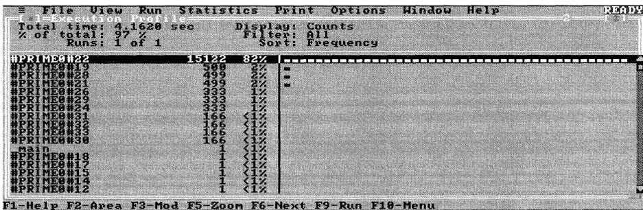
This display of PRIME0's statistics shows that line 22 is the most frequently called line in PRIME0.
