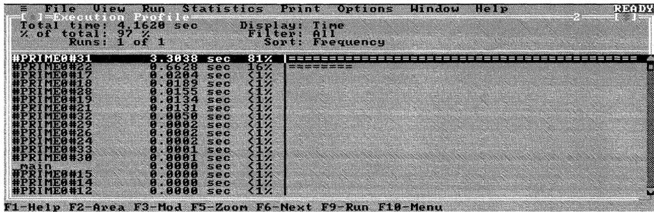
The upper pane of the Execution Profile window displays the program's total execution time, along with information about the data in the lower pane. The lower pane has four fields for each line:
