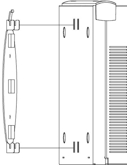
2. Position the logic unit on the bracket by directing the slots in the unit around the tabs on the bracket.
