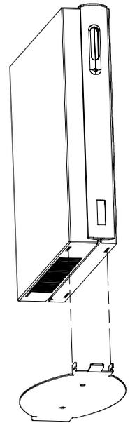
2. Position the logic unit on the bracket by directing the slots in the unit around the tabs on the bracket.
