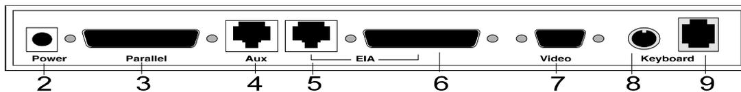
2. **Power Connection** - plug the power cord into this connector and the wall-mount or other remote transformer into a properly grounded receptacle.
