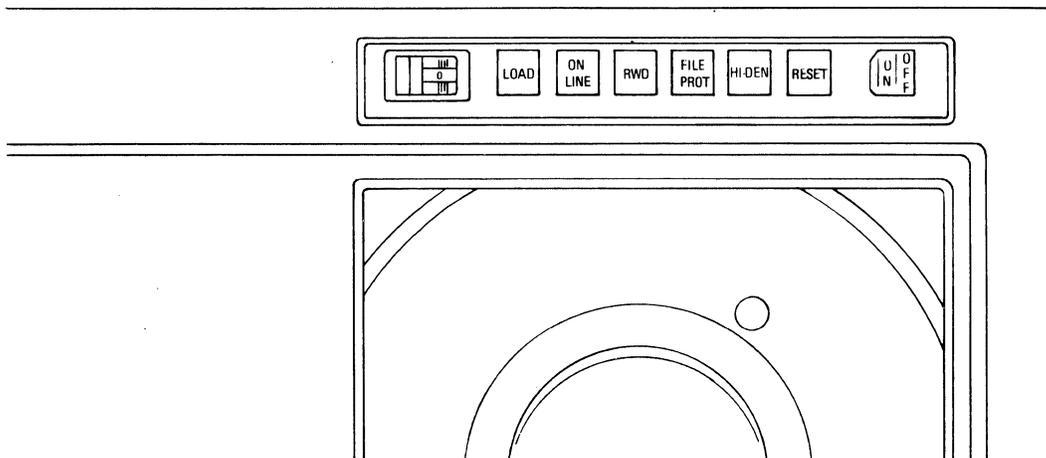
Figure 3-1. Tape Unit Front Panel Controls and Indicators
