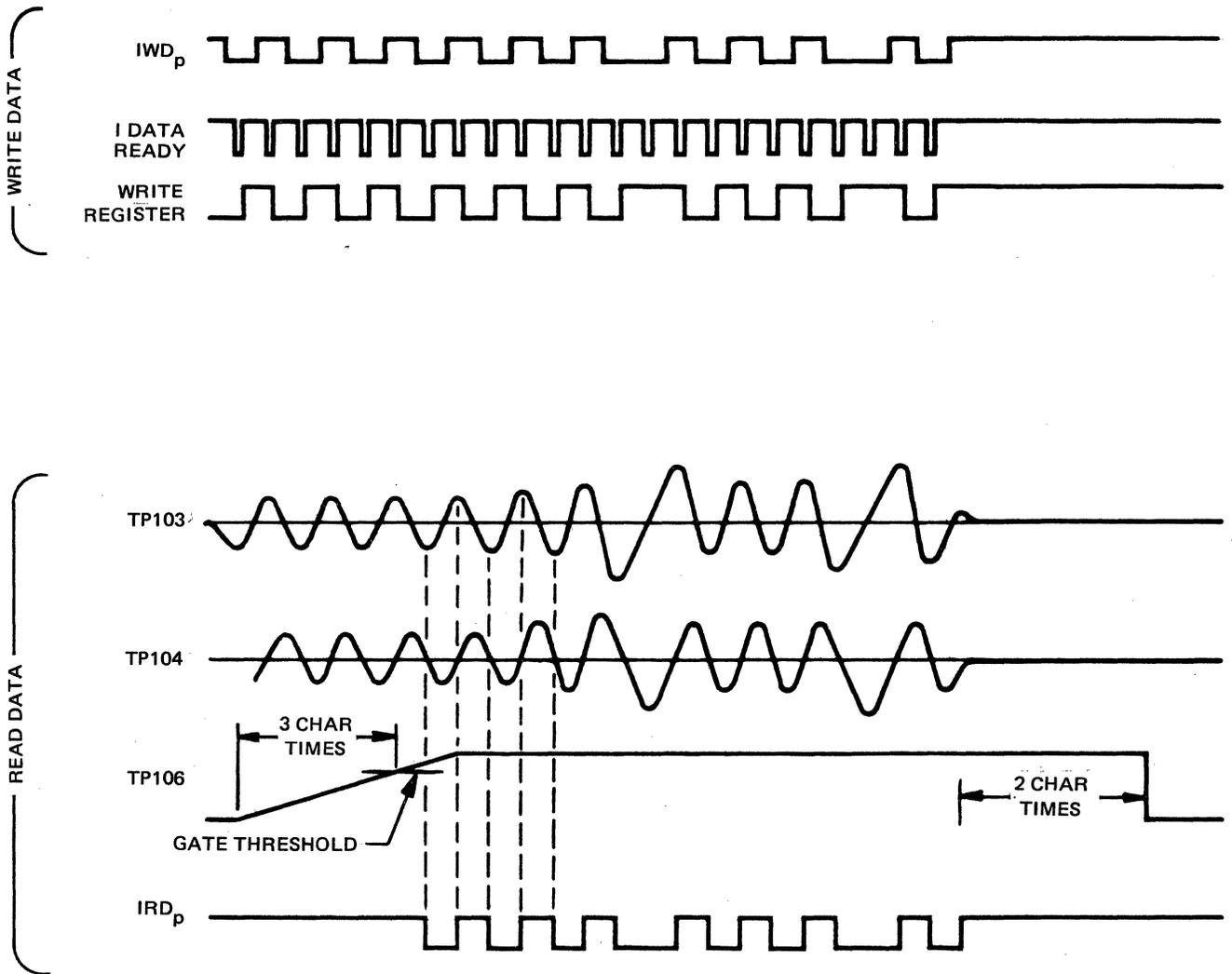
Figure 4-28. PE Data Write/Read Timing Diagram
