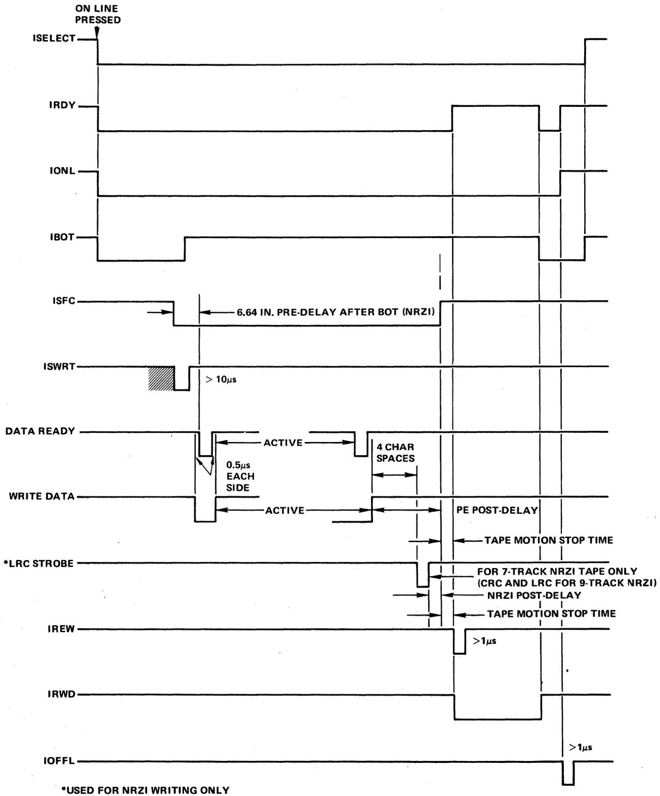
Figure 3-10. Timing Diagram for a Typical Start-Write-Stop Sequence.
