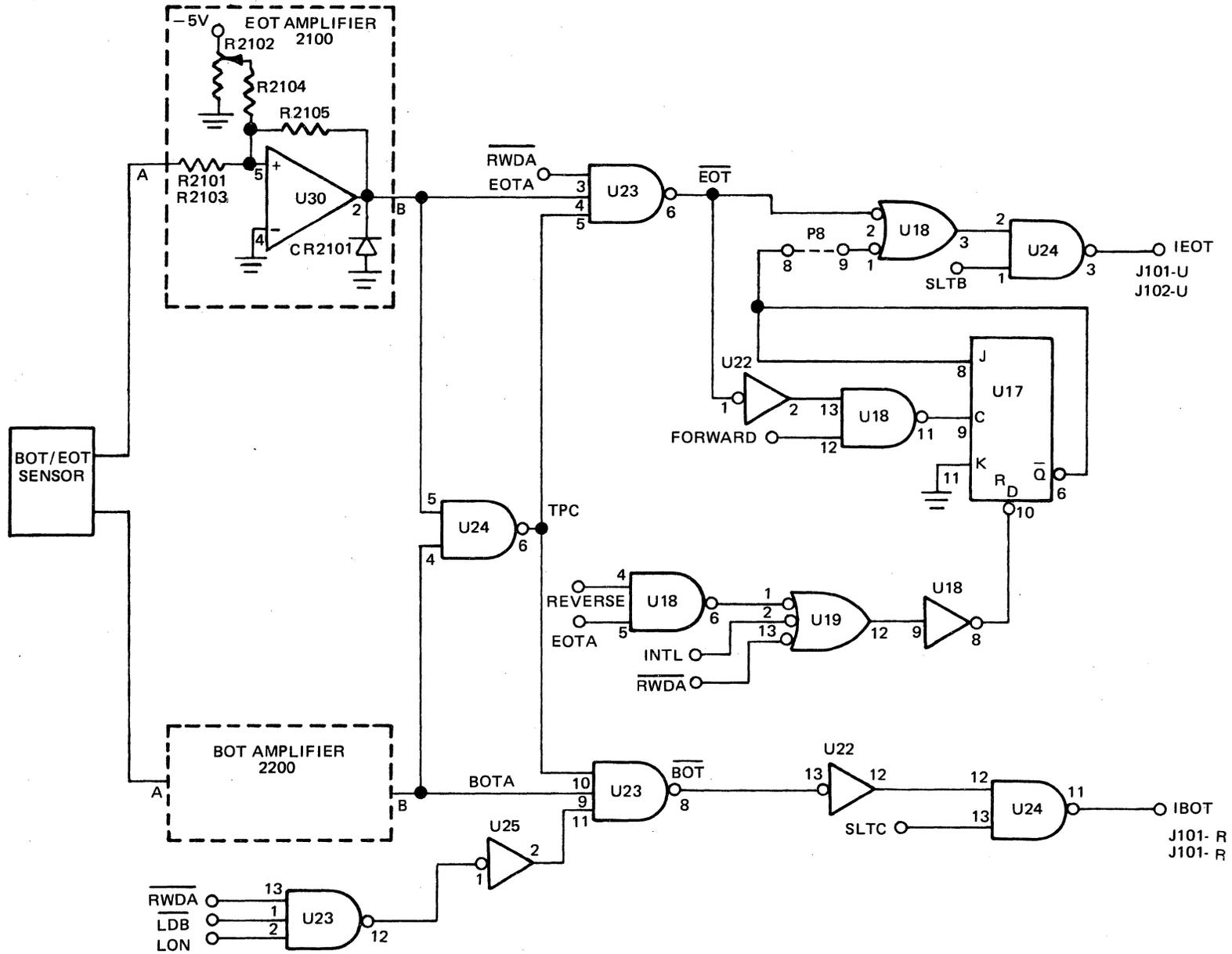
Figure 4-22. EOT/BOT Control Logic Circuit Simplified Diagram
