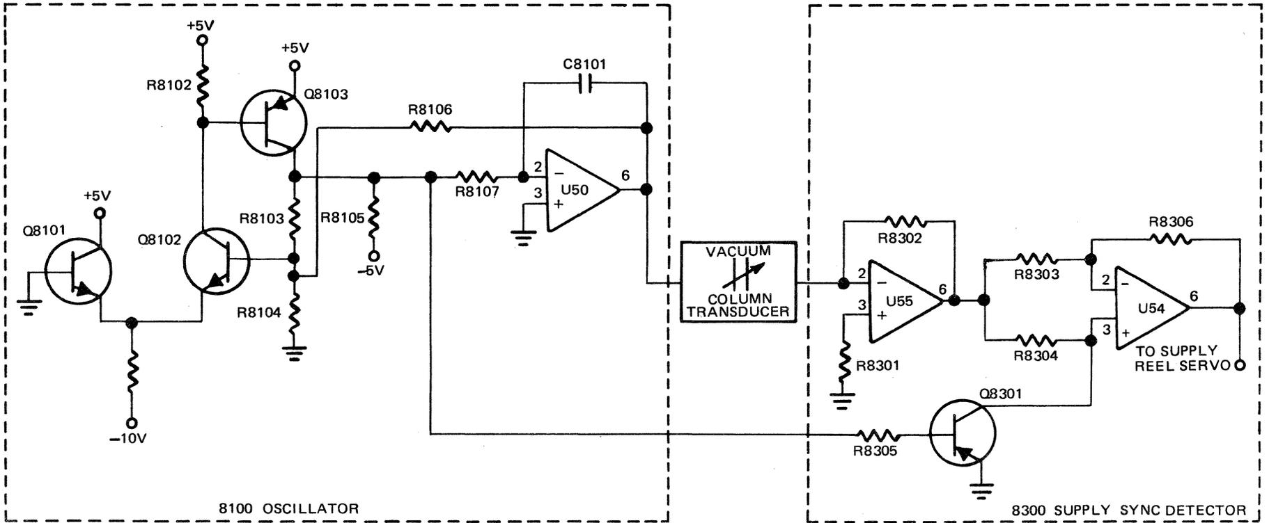
Figure 4-11. Vacuum Column Position Sensor Circuits Simplified Diagram
