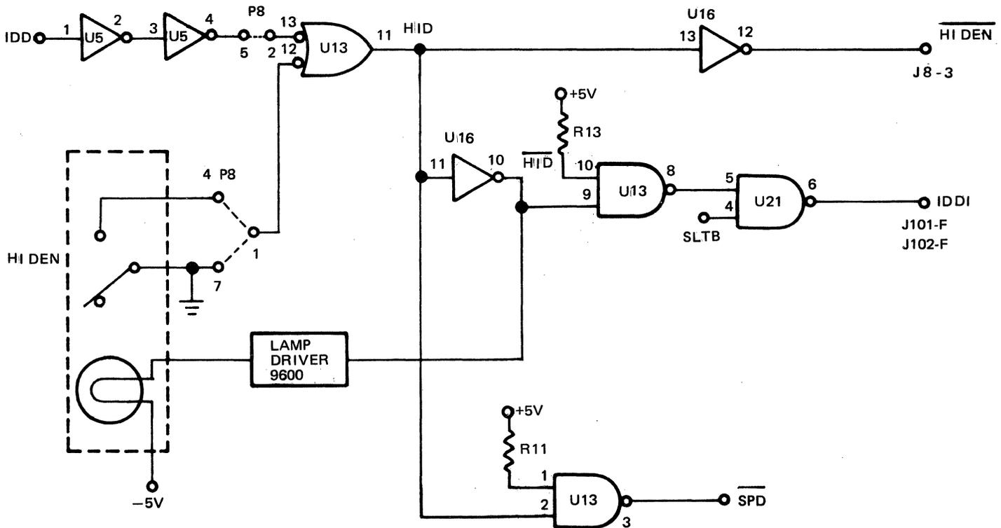
Figure 4-23. Density Select Circuits Simplified Diagram
