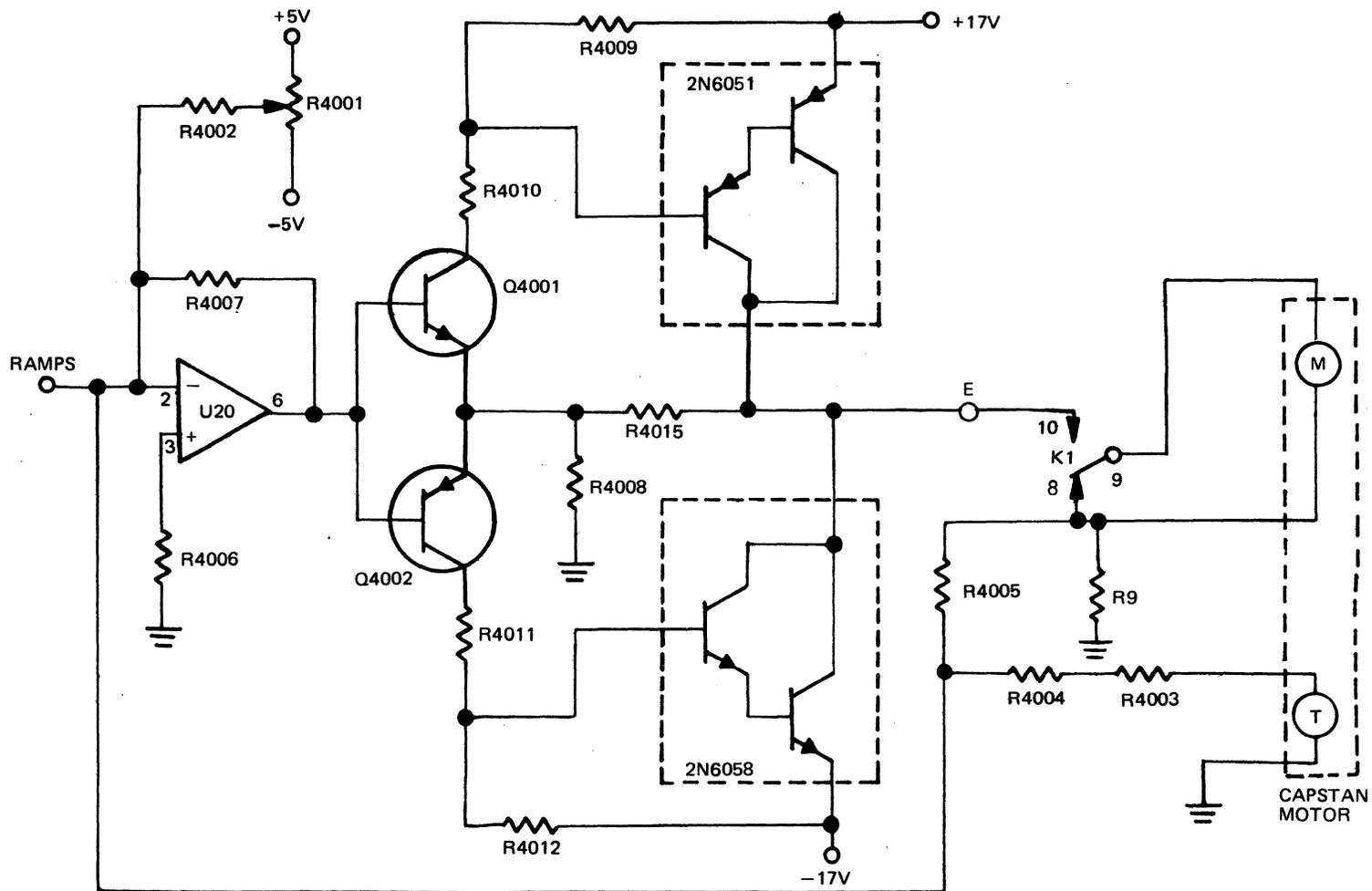
Figure 4-15. Capstan Amplifier Circuit Simplified Diagram
