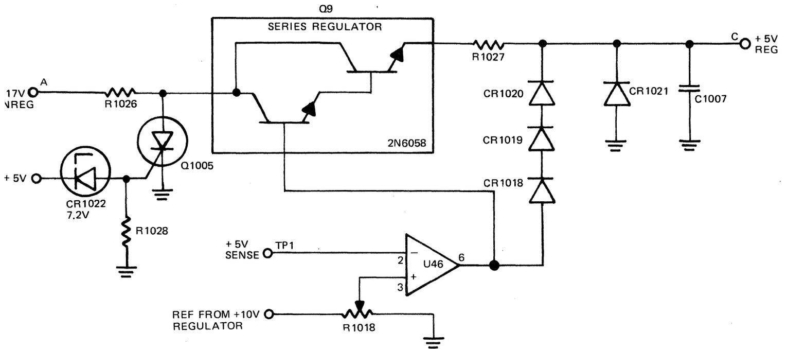
Figure 4-6. + 5 Volt Regulator Circuit Simplified Diagram
