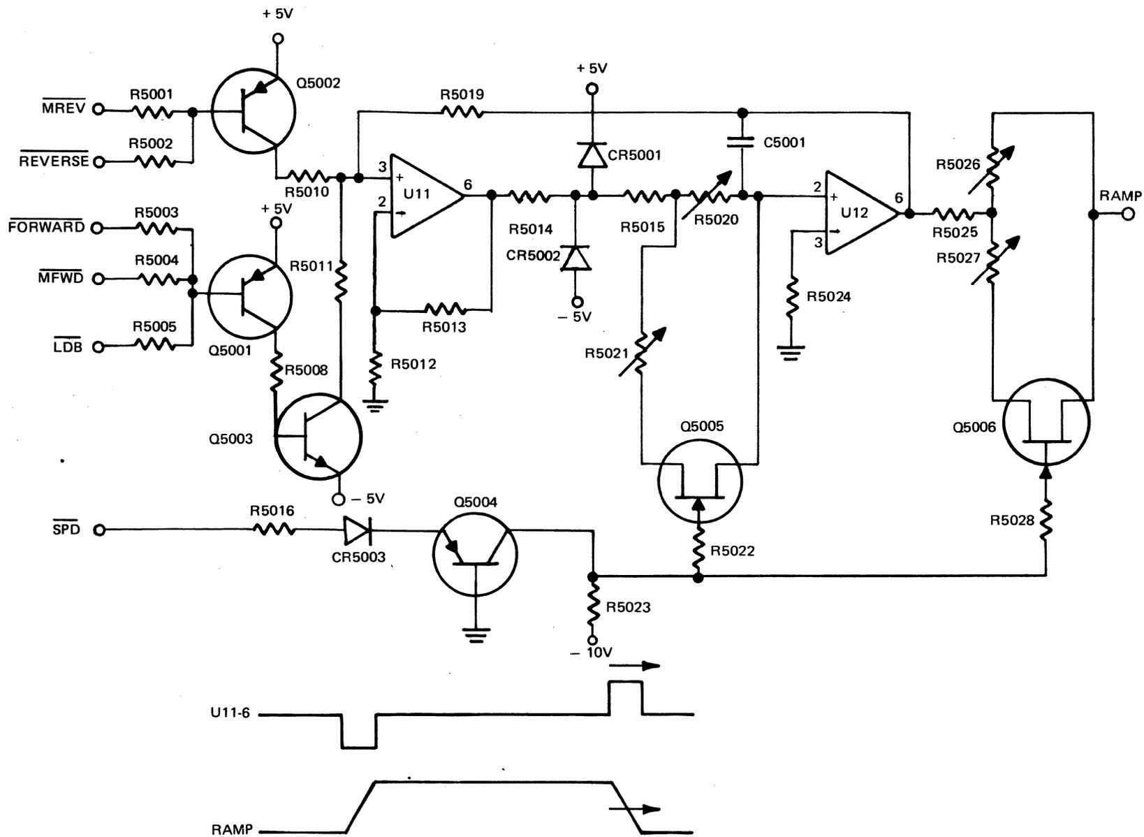
Figure 4-13. Forward/Reverse Ramp Generator Simplified Diagram
