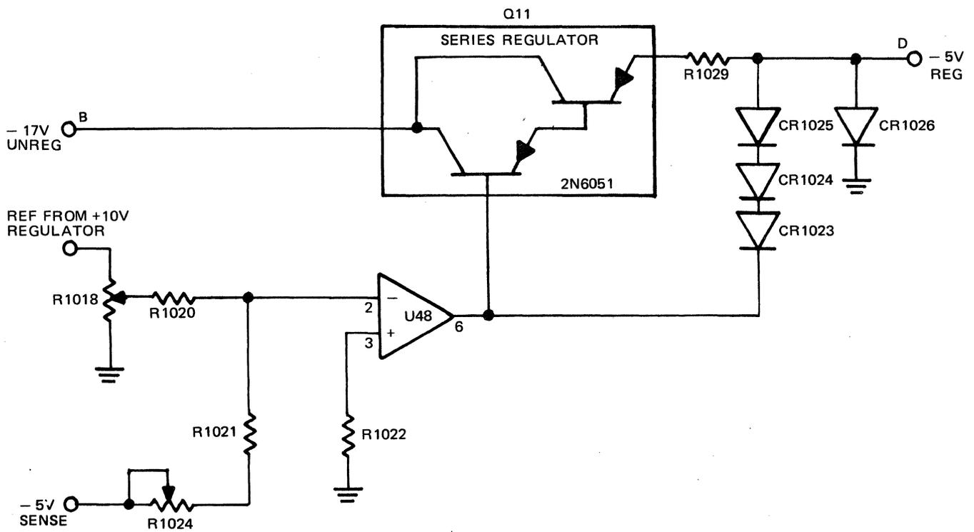
Figure 4-7. -5 Volt Regulator Circuit Simplified Diagram
