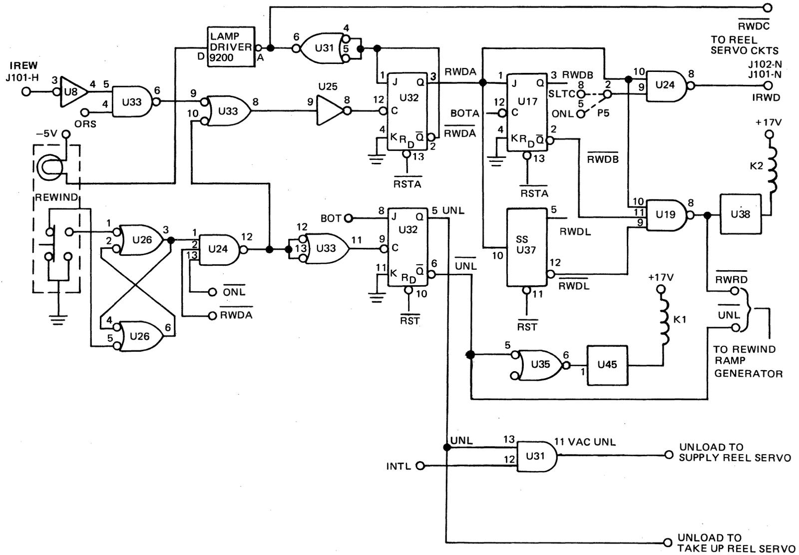
Figure 4-21. Rewind/Unload Control Circuits Simplified Diagram
