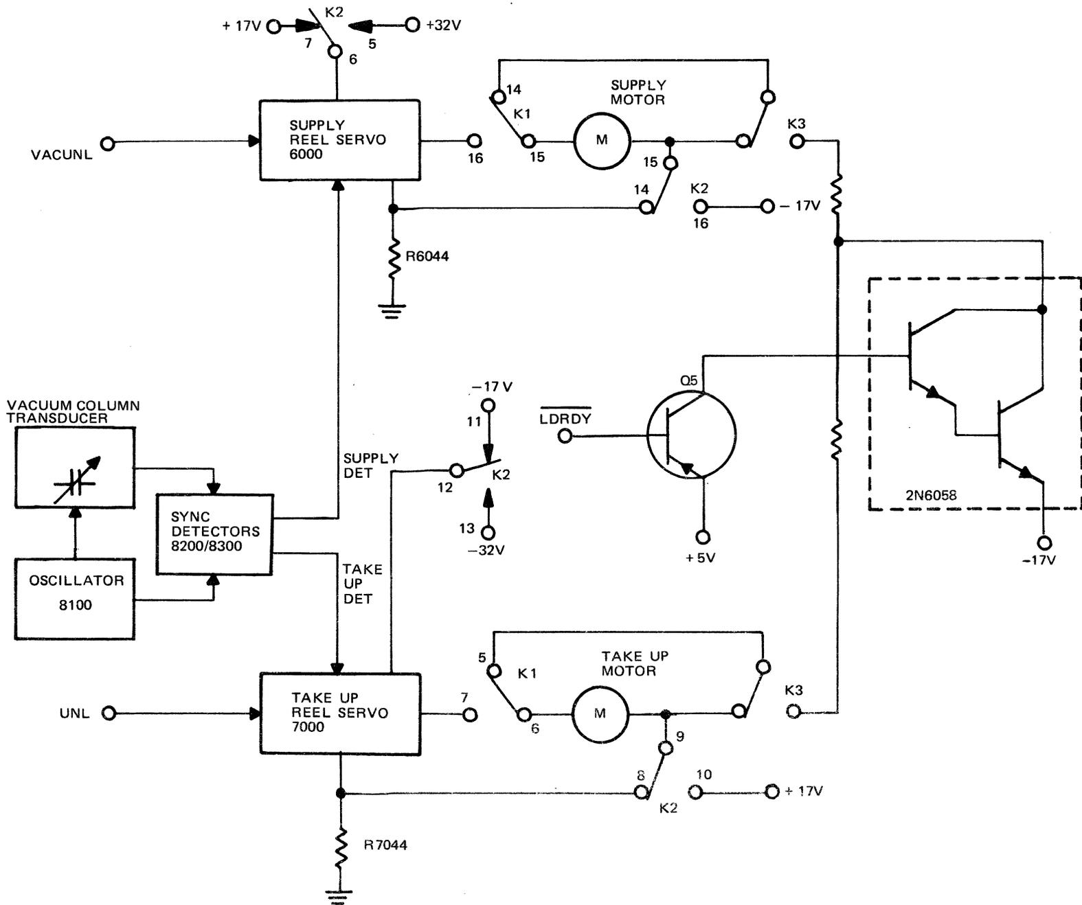
Figure 4-10. Reel Servo Electronics Simplified Diagram
