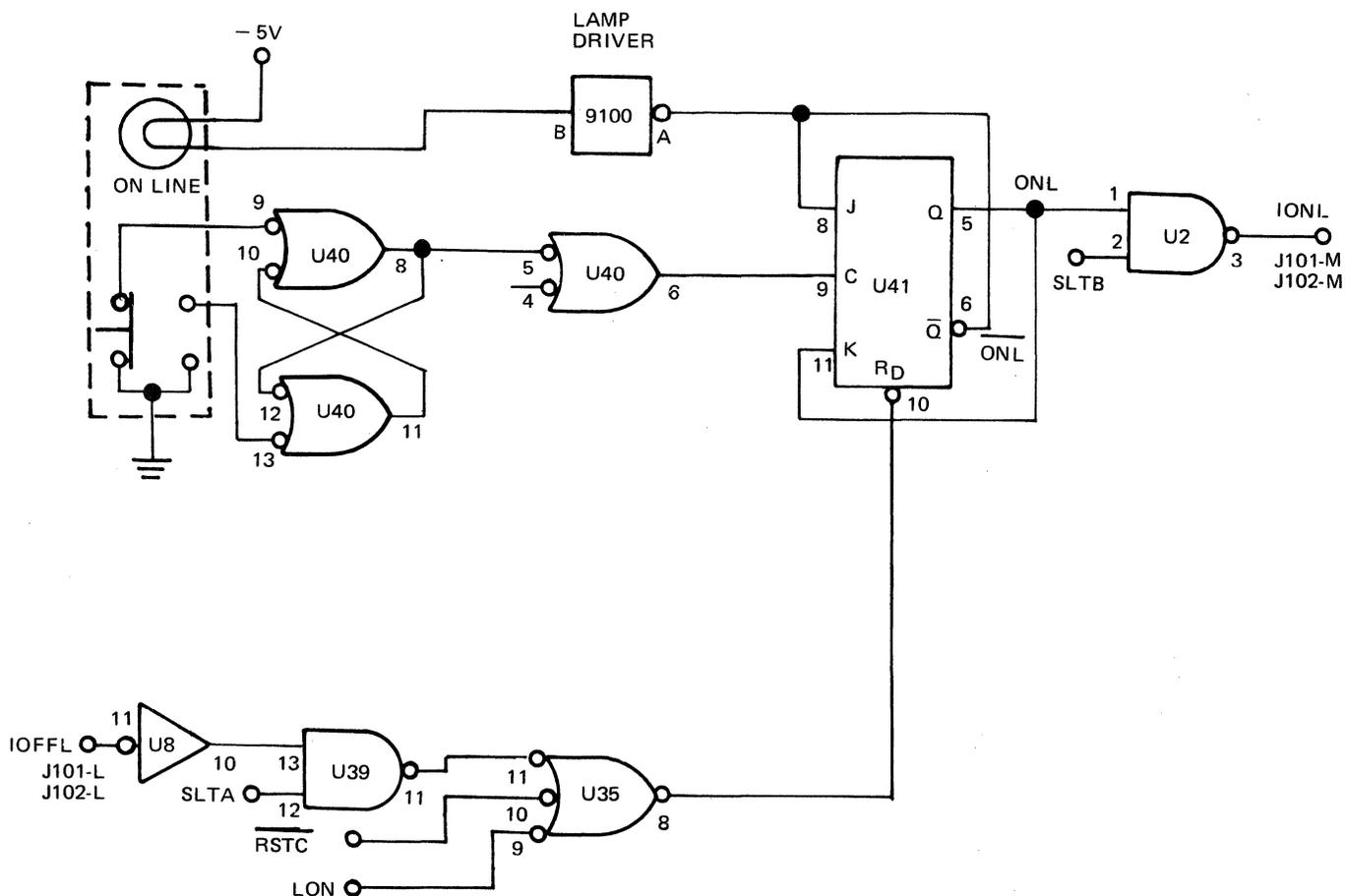
Figure 4-16. On-Line/Off-Line Logic Circuits Simplified Diagram
