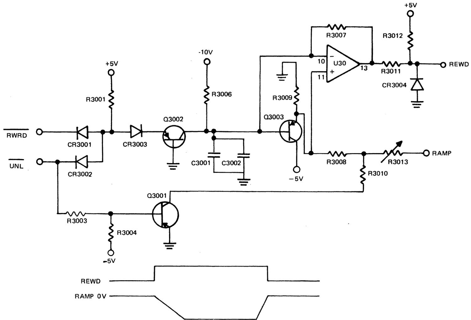
Figure 4-14. Rewind Ramp Generator Circuit Simplified Diagram
