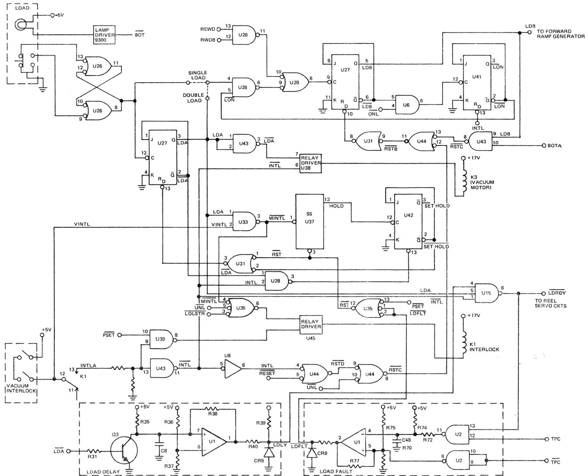
Figure 4-9. Vacuum Column/Double Load Logic Simplified Diagram
