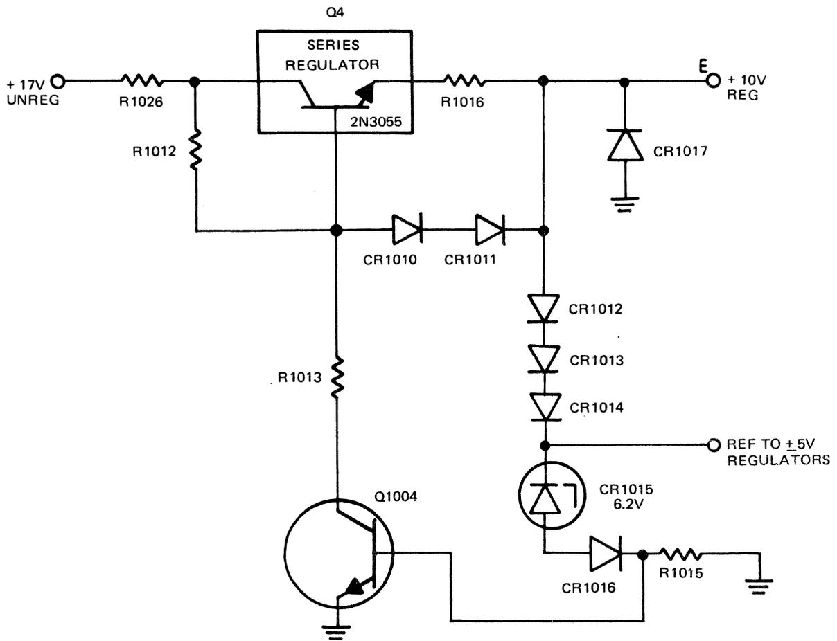
Figure 4-4. +10 Volt Regulator Circuit Simplified Diagram
