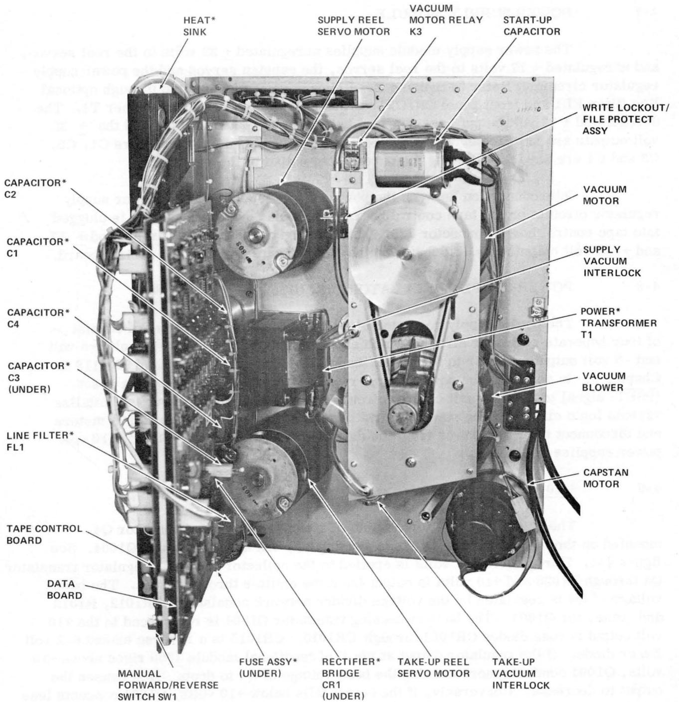
Figure 4-2. Model 2750 Tape Unit Mechanical Assembly
