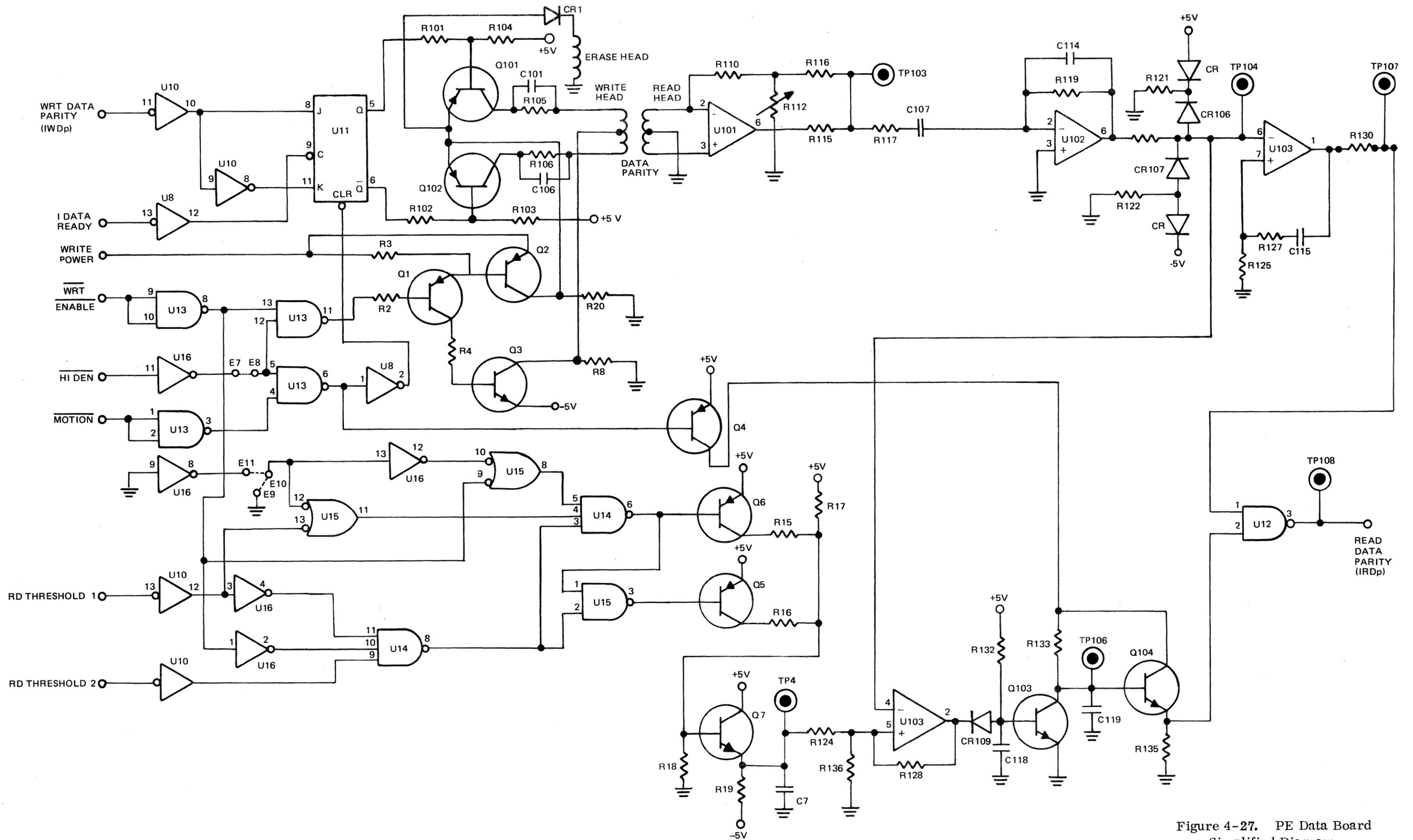
Figure 4-27. PE Data Board Simplified Diagram
