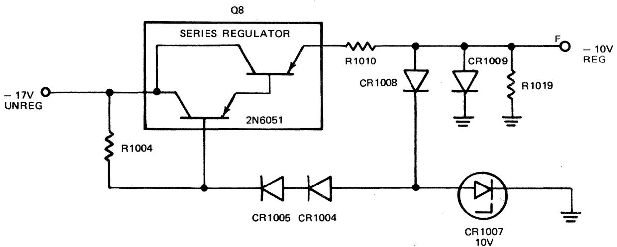
Figure 4-5. -10 Volt Regulator Circuit Simplified Diagram
