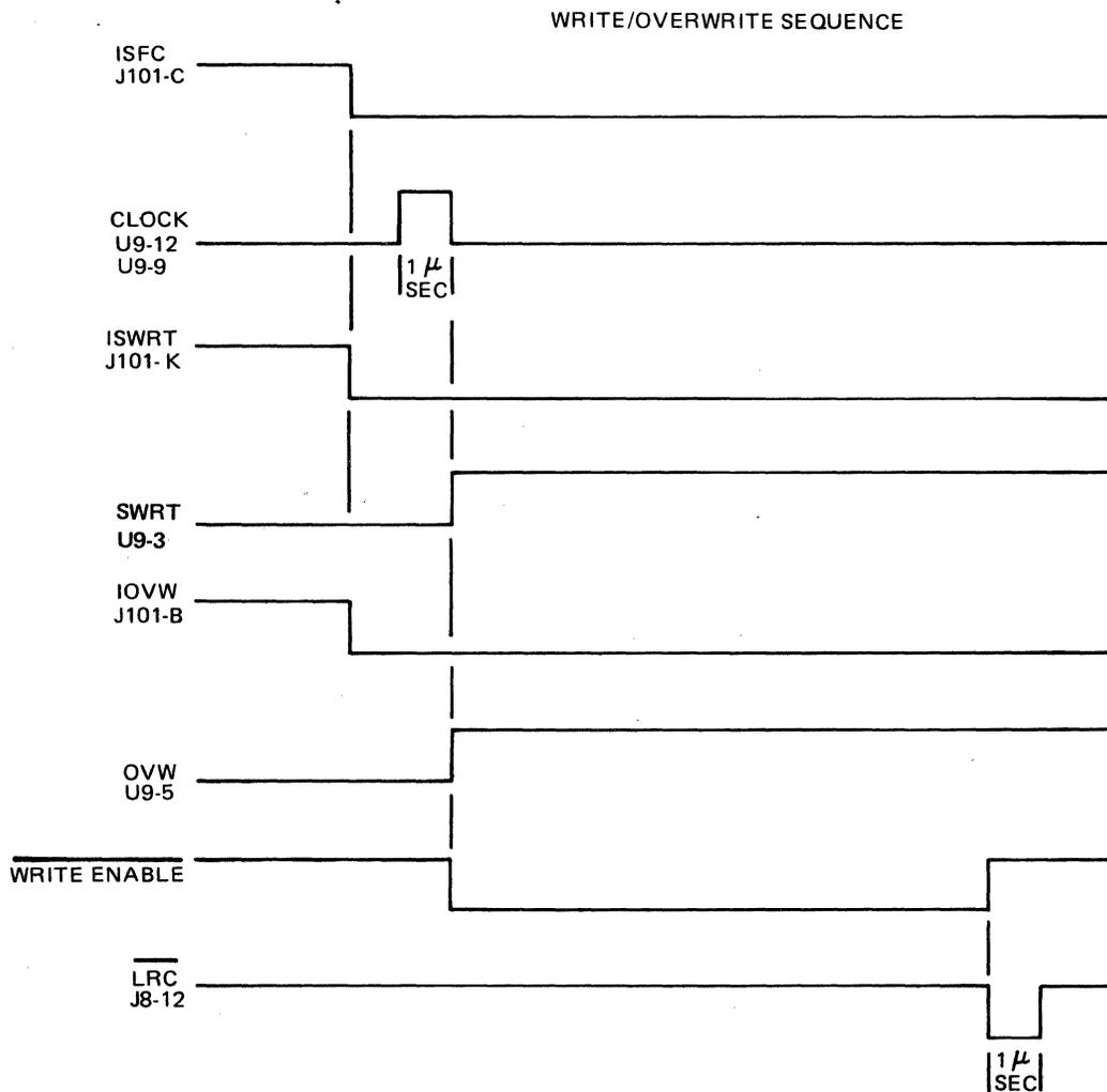
Figure 4-20. Write/Overwrite Timing Diagram
