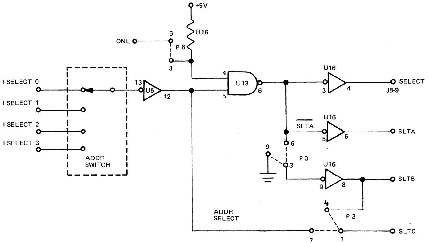
Figure 4-17. Address Logic Circuit Simplified Diagram
