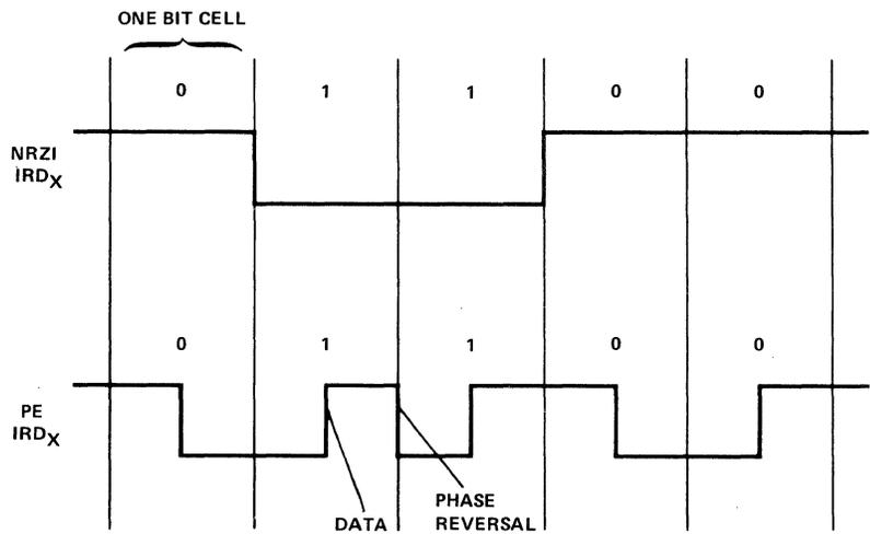
Figure 3-5. NRZI and Phase Encoded Data Formats
