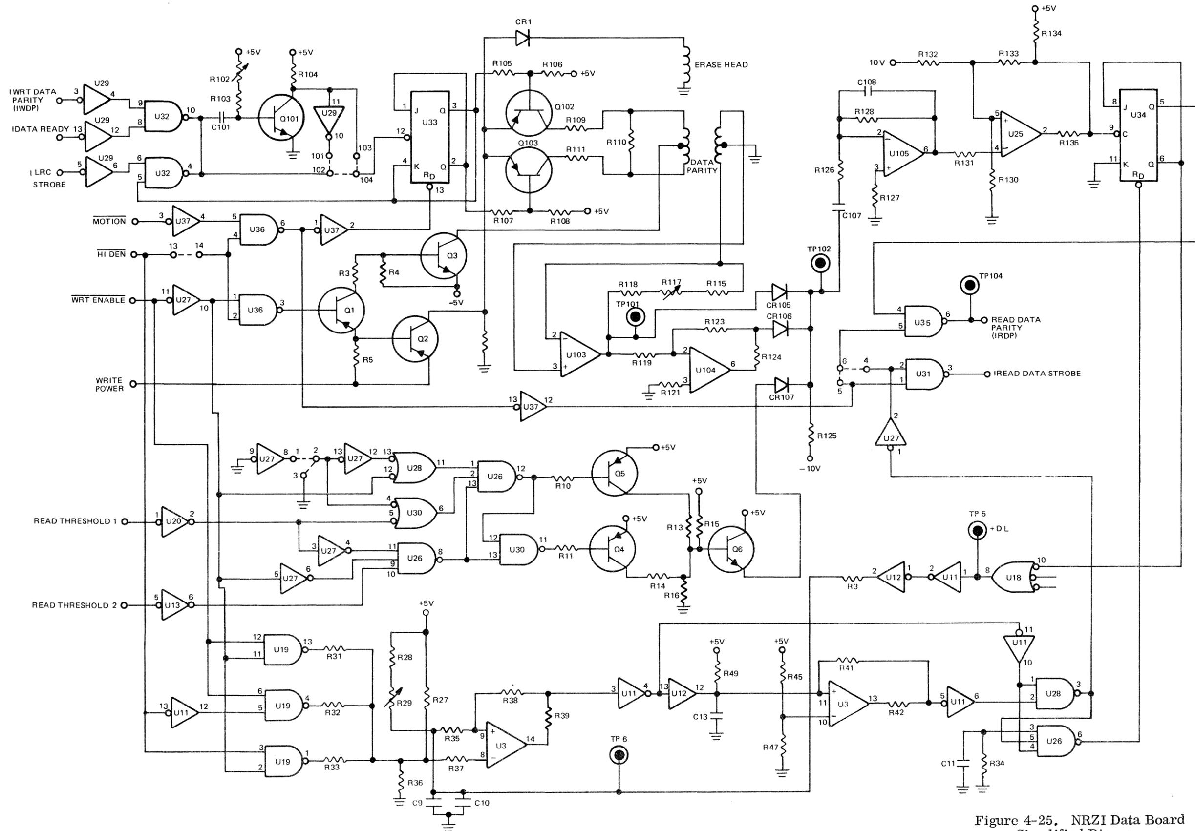
Figure 4-25. NRZI Data Board Simplified Diagram
