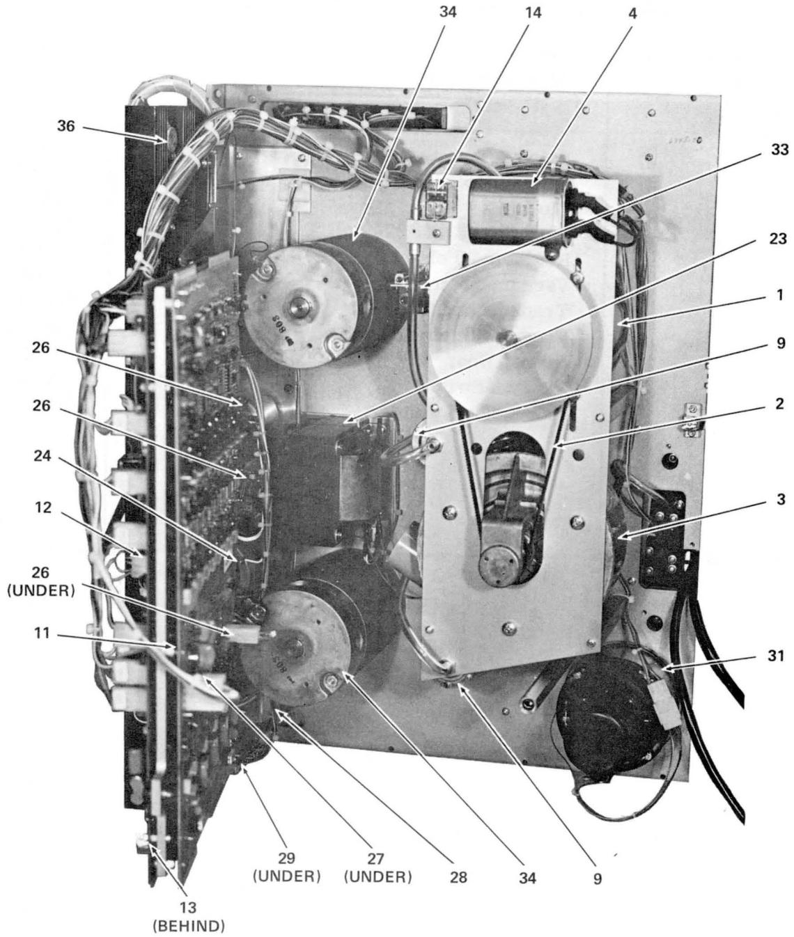
Figure 6-2. Model 2750 Parts Location, Rear View
