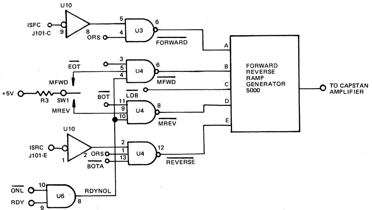
Figure 4-18. Forward/Reverse Control Circuits Simplified Diagram
