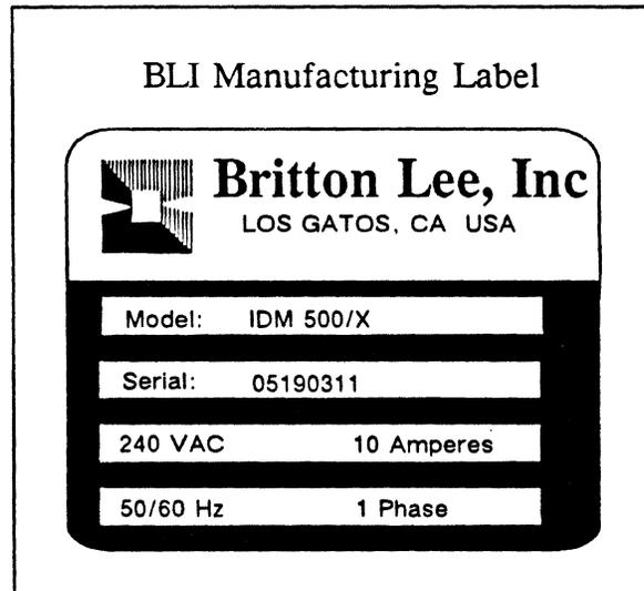
Figure D-1: BLI Manufacturing Label
