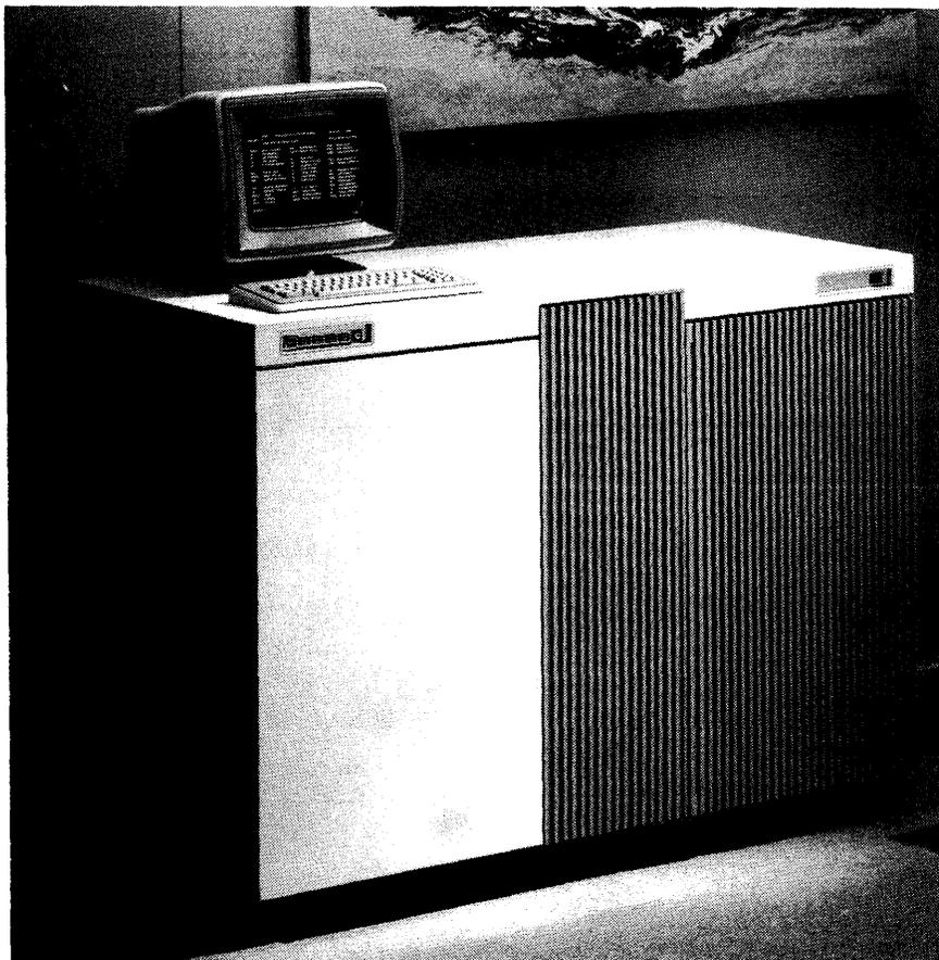
*The Unisys A 5 Model F is a single-processor system with 6 megabytes of memory, expandable to 24 megabytes in 3-megabyte increments. It contains two I/O bases in its processor cabinet and can accommodate one expansion cabinet with two additional I/O bases supporting a total of 160 data communications lines.*
