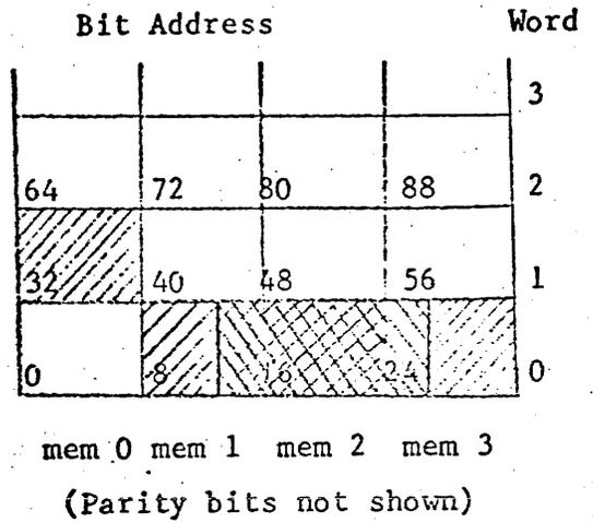
Figure 8. Words (shaded cells) delivered to FIU satisfying request for 13 bits beginning with location 13, forward.
