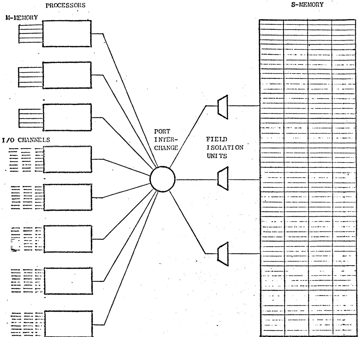
Each processor may have either 1-8 I/O channels or 1-4 micro-program memory modules of 16,384 bits each.
