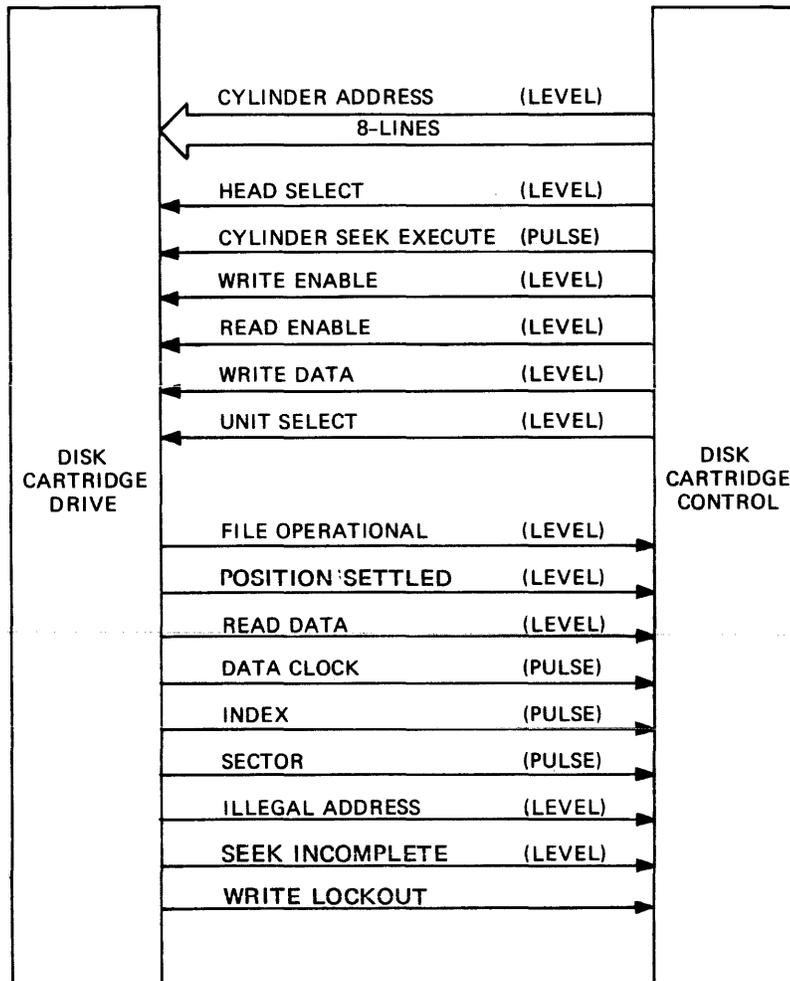
Fig. I-3 CONTROL TO DISK CARTRIDGE INTERFACE
