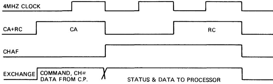
Fig. II-14 BASIC INTERFACE TIMING
