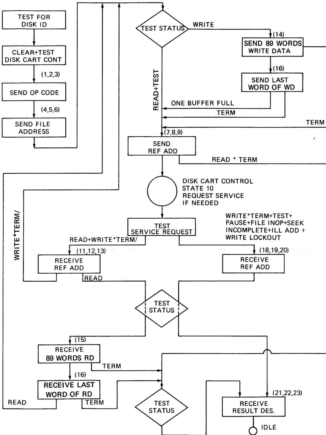
Fig. V-1 PROCESSOR TO DISK CARTRIDGE CONTROL FLOW
