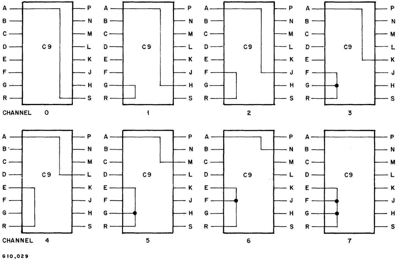
Figure VI-2. Channel Designate Wiring (Channels 0 through 7)
