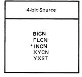
\* INCN is not physically present on the S-Memory Processor. When addressed as a source it yields a binary value of 0. When addressed as a sink (destination) the data is lost.
