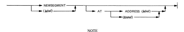
The  $\langle literal \rangle$  must be MOD 16, meaning the last four bits must be @ (1) 0000 @.
