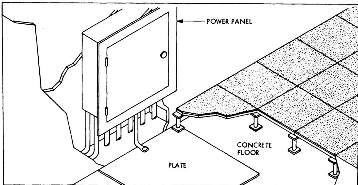
Figure I-4. Elevated Floor Grounding
