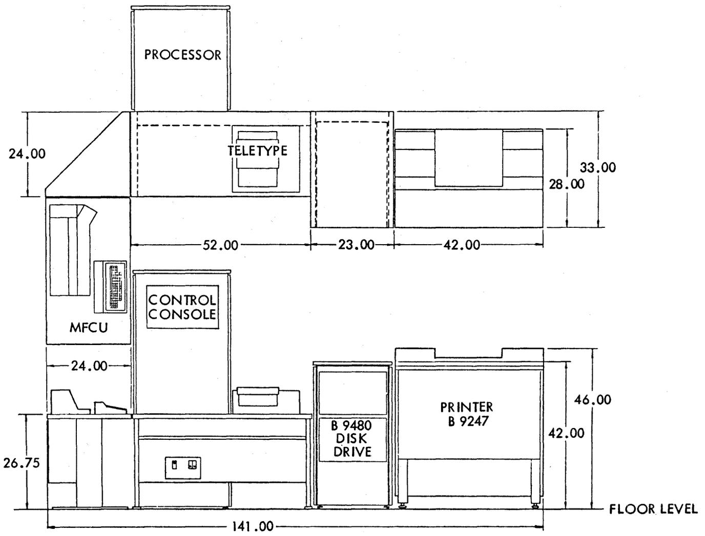
Figure IV-9. Corner Table With Printer to the Right (Sheet 3)
