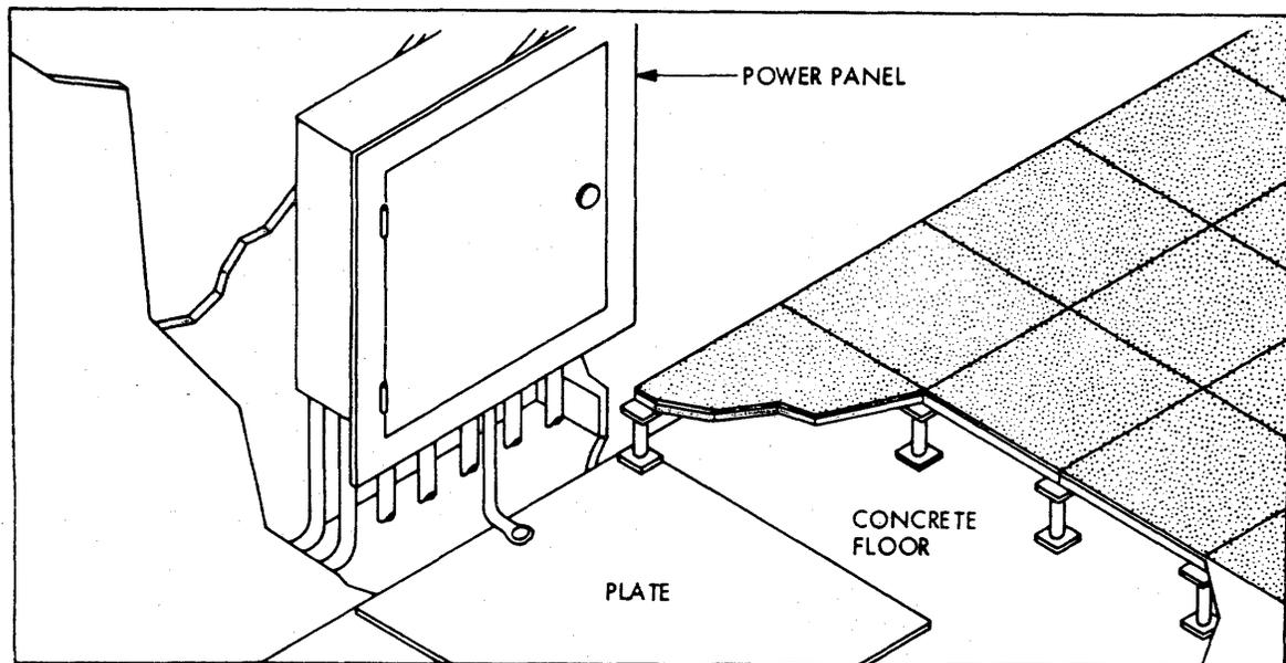
Figure I-4. Elevated Floor Grounding
