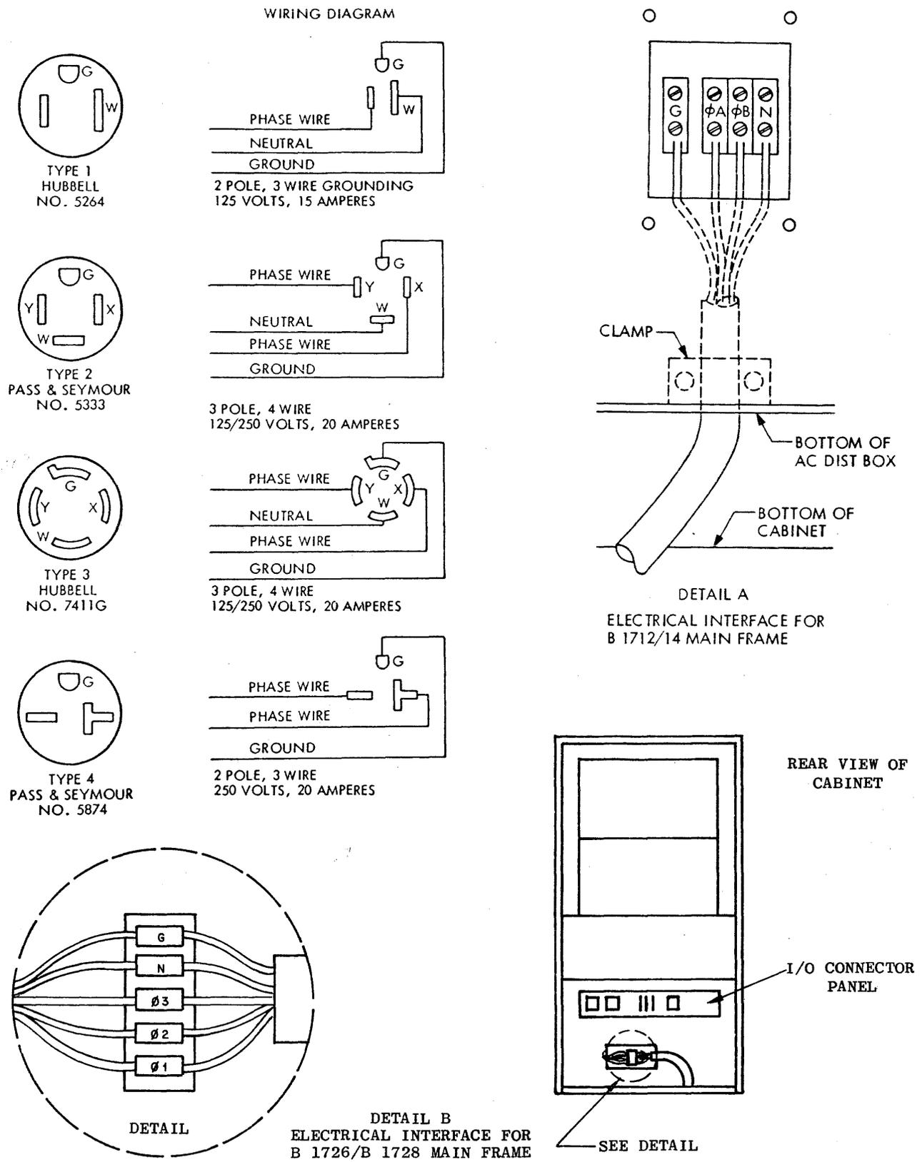
Figure I-5. Receptacle Description (Sheet 1)
