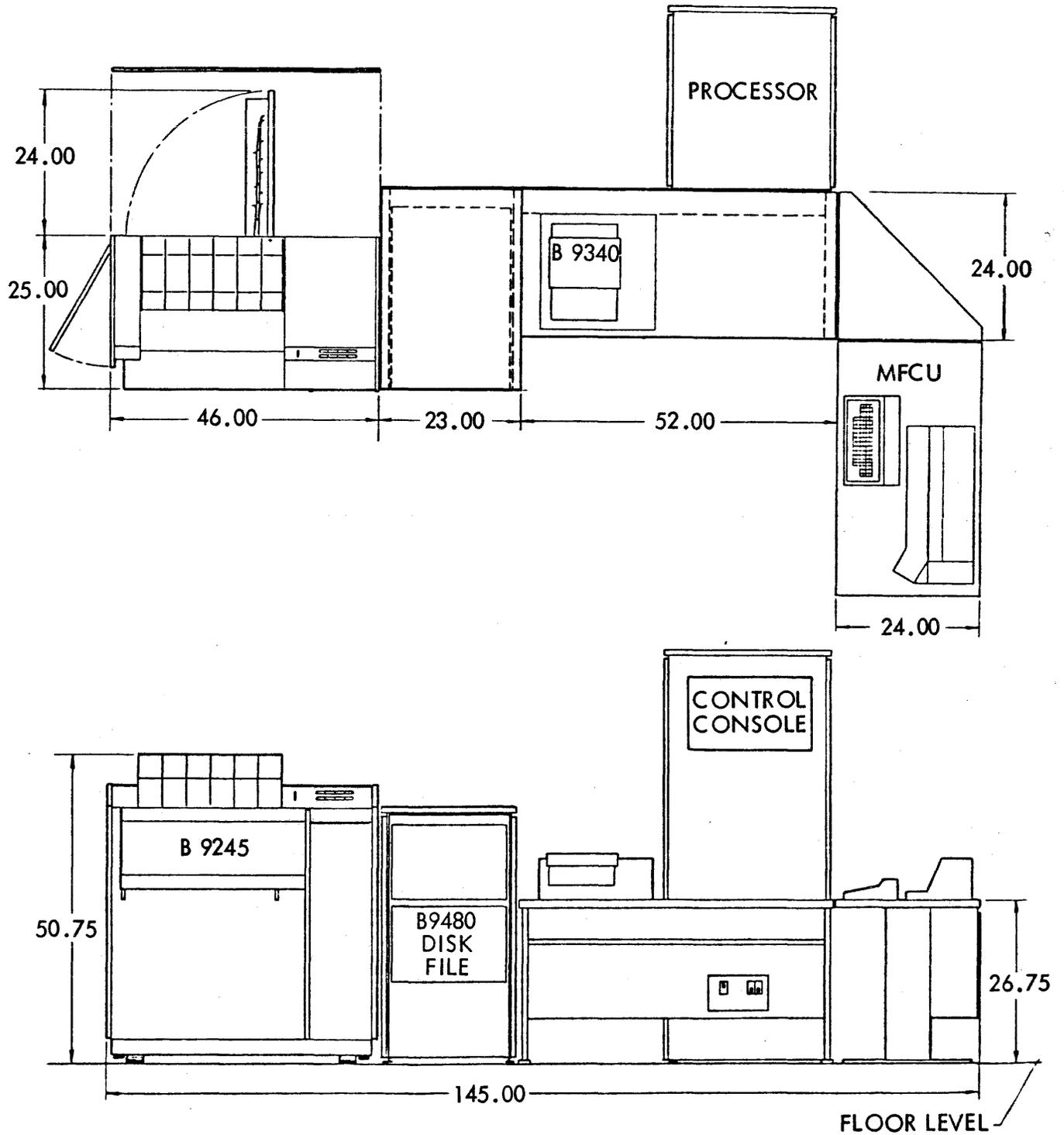
Figure IV-9. B 1712/B 1714 Corner Table with Printer to the Left (Sheet 1)
