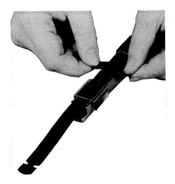
Figure 2-58. Applying Adhesive Tape to Magnetic Tape Ends
