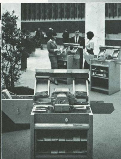
The lightning-fast J700 Printing Calculator, left, is one of more than 20 adding machines offered by Burroughs on the California market. At the right is a MICRIGHT on-premise encoding system, one of several Burroughs devices used by banks to imprint personalized encoded checks.
