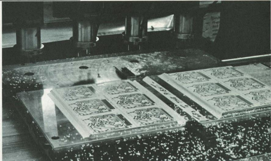
A numerically-controlled drilling machine automatically drills precise holes in printed circuit boards.
