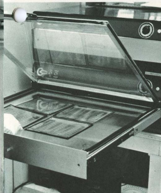
A photo printer produces patterns on circuit boards coated with photo-sensitive material.
