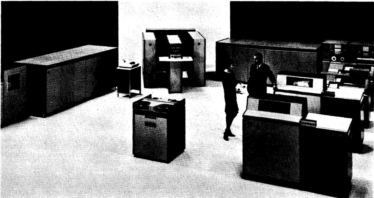
*Dual printers and card readers plus several disk file modules equip this B 3500 system for effective multiprogramming.*
