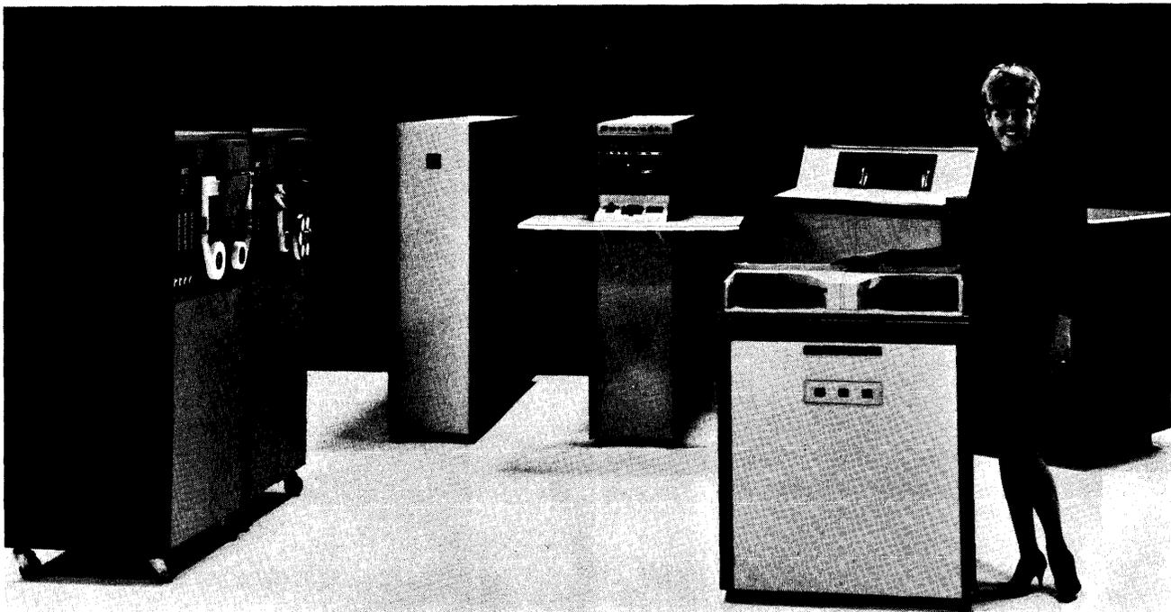
*This small B 2500 configuration includes the unique Burroughs Magnetic Tape Cluster (foreground) and paper tape I/O units (at left).*
