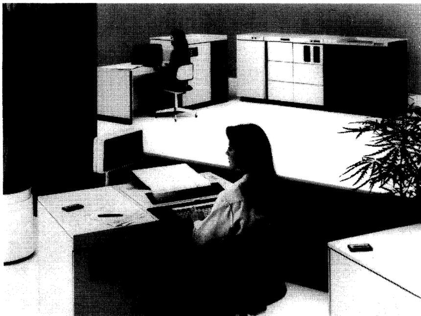
*The B 1830, smallest member of the new Burroughs small-to-medium-scale computer family, offers 48K to 262K bytes of MOS memory. The unit in the foreground is Burroughs' new AE 412 Audit Entry Data Preparation System.*
