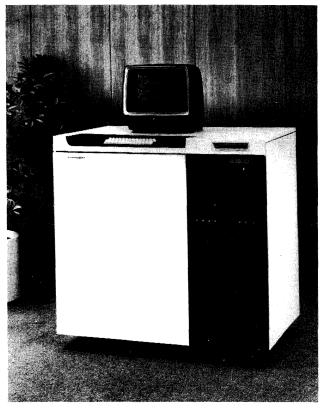
Burroughs claims the new B 1800 processors offer significant price/performance improvements over the older models. The B 1815, B 1855, and B 1885, which now make up the actively marketed B 1800 product line, occupy 50 percent less floor space and consume 25 percent less electrical power than the older processor models such as the B 1870.
