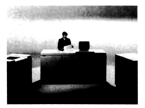
Burroughs claims the B 1885, shown here, is the first system in its price class to offer two independent central processors. The processors share the main memory, which can extend from 512K bytes to 1.02 megabytes. One processor acts as a slave in this configuration, with the MCP operating system residing only in the master processor.
