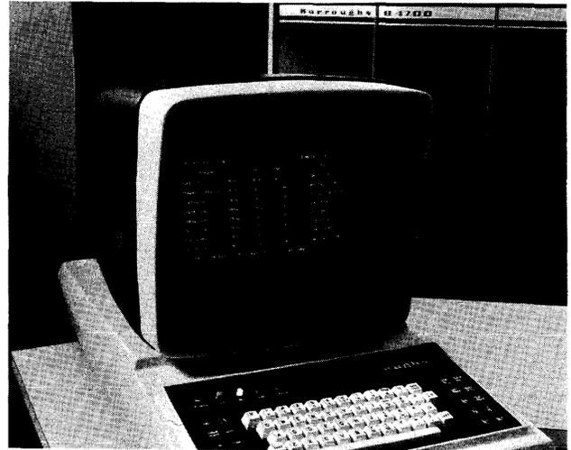
*The B 9340-1 Operator Display Console facilitates man/machine communications and provides regularly updated status displays that list the active programs in the multiprogramming mix.*
